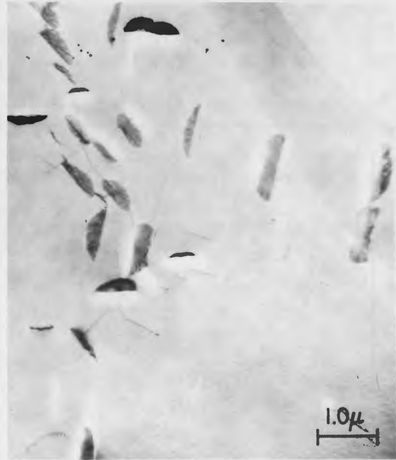
(a) 1 hr., 100°C, MATRIX PLUS DISLOCATION (b) 10 min., 200°C, DISLOCATION
