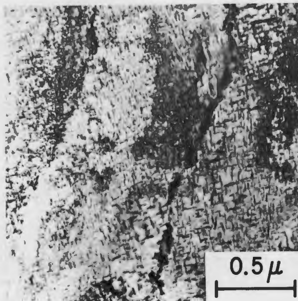
FIG. 21 -- PRECIPITATION IN A MARTENSITIC Fe-20Ni-1Ti ALLOY AGED AT 500°C FOR 24 HRS.
