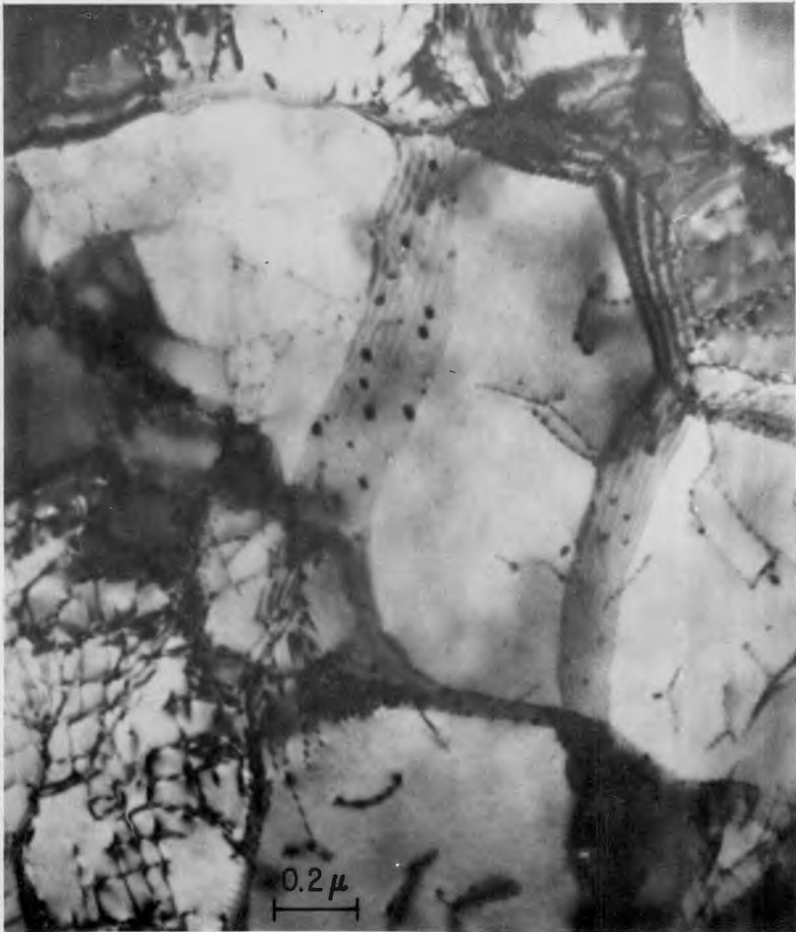
FIG. 28 -- COPPER PRECIPITATED IN CELL BOUNDARIES. Fe-0.8% Cu, COLD ROLLED 60%, HELD 3 HRS. AT 500°C, 10 MIN. AT 650°C.
