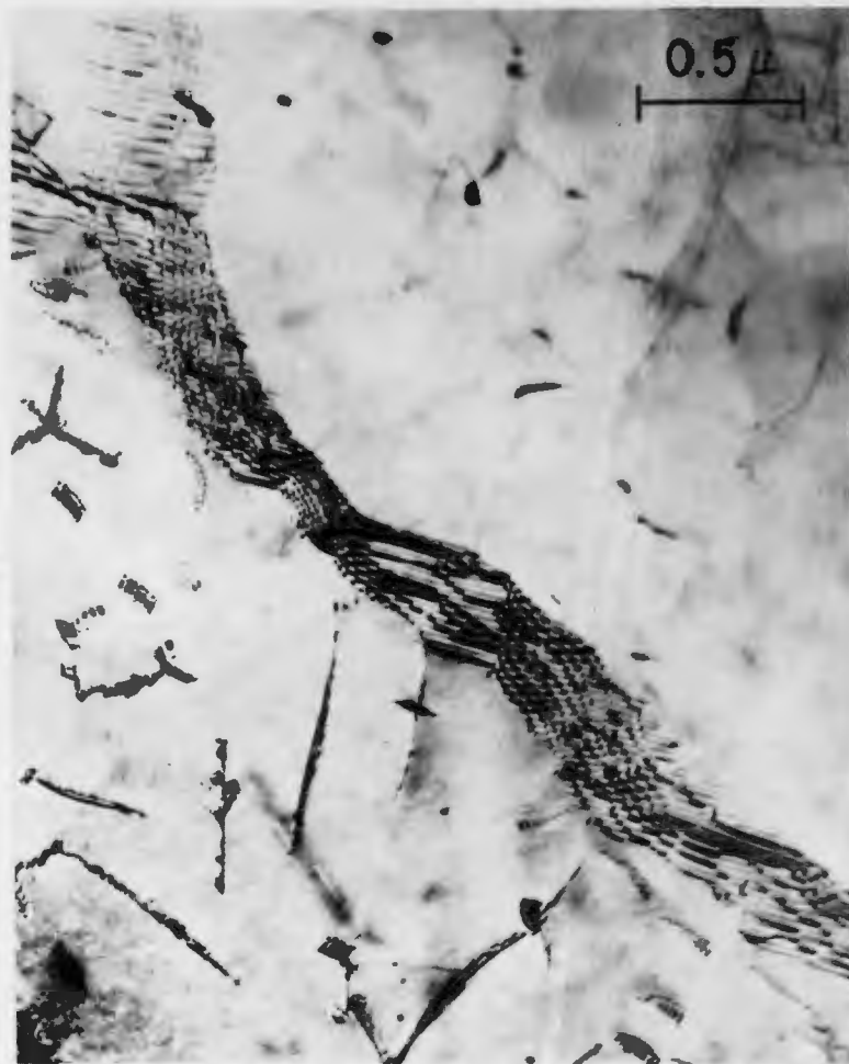
FIG 7 -- PRECIPITATION OF \text{Fe}_{16}\text{N}_2 ON A SUBBOUNDARY IN AN Fe-0.01% N ALLOY AGED 2 HRS. AT 100°C.
