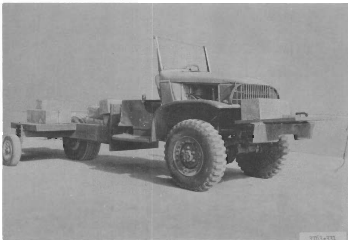
Figure 2. Load vehicle used on lanes 15 and 16
