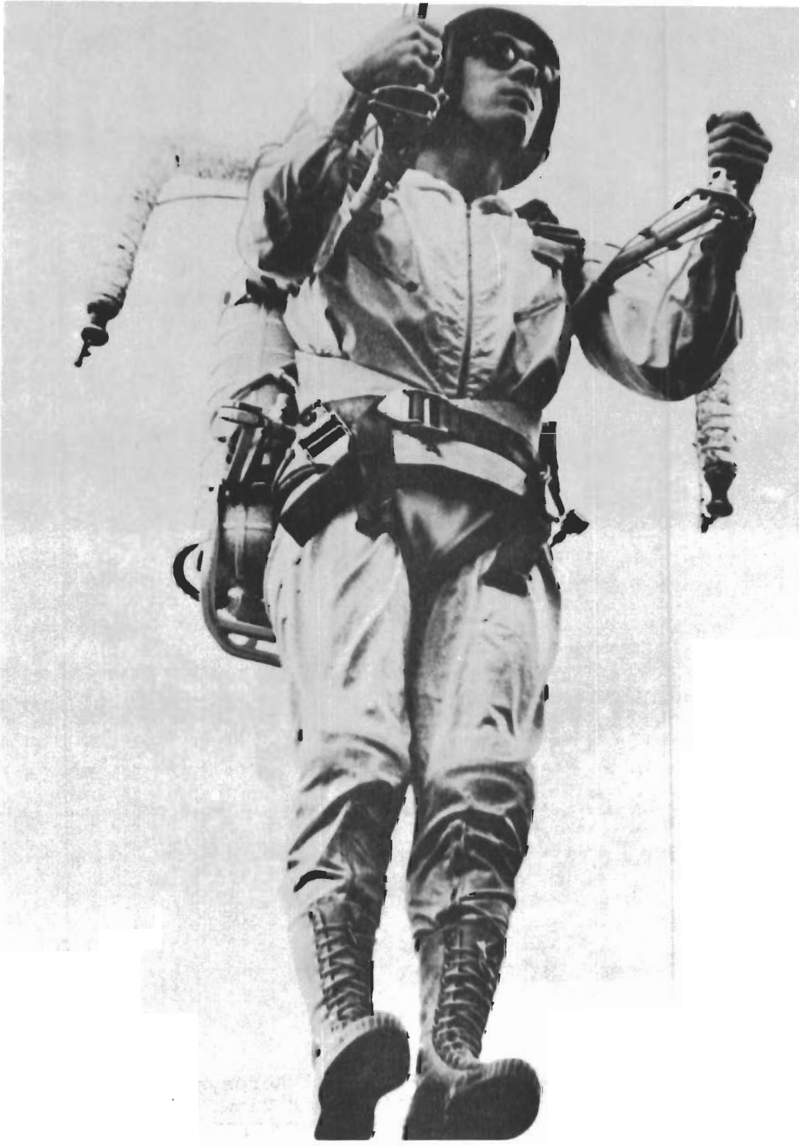
Figure 2.2.2.9 Final Configuration of the Bell Aerosystems Rocket Belt, in Flight (Courtesy Bell Aerosystems Co.)
