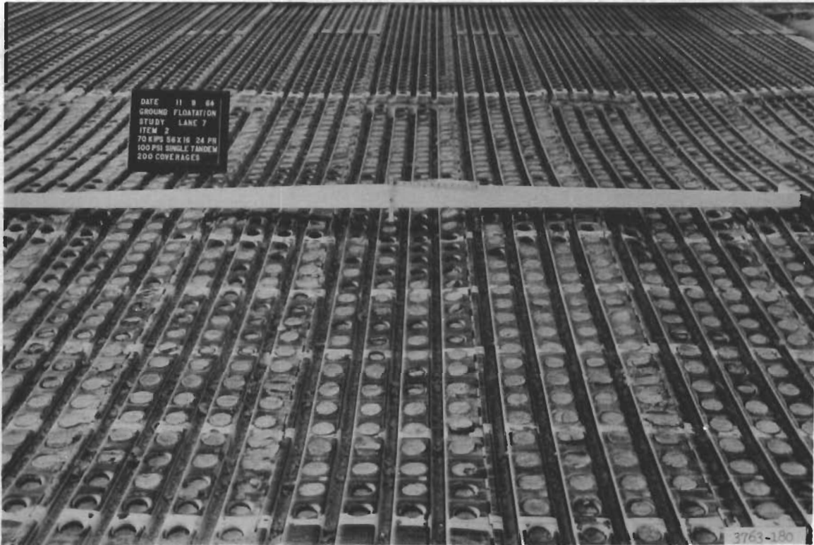
Fig 10. Lane 7, item 2. Longitudinal straightedge shows roughness along mat joint line at 200 coverages (failure)
