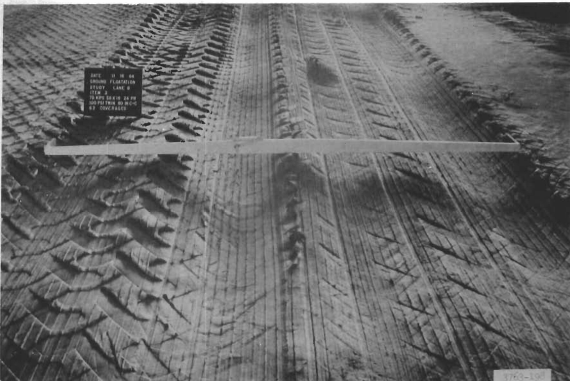
Fig 19. Lane 8, item 3. Transverse straightedge shows rutting at 62 coverages (failure)
