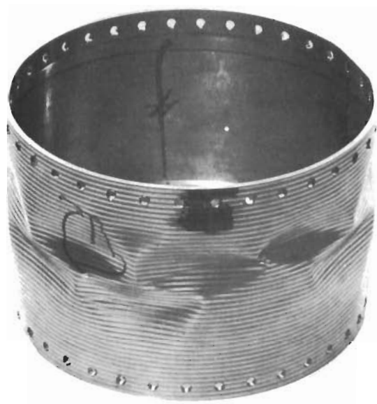
Ring Stiffened Cylinder (Specimen No. 67)
