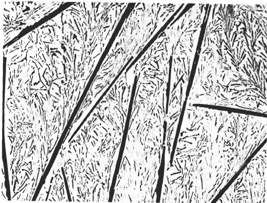
Figure 104. Ti-Mo-C (22-20-58 At.%), Melted and Rapidly Cooled.
