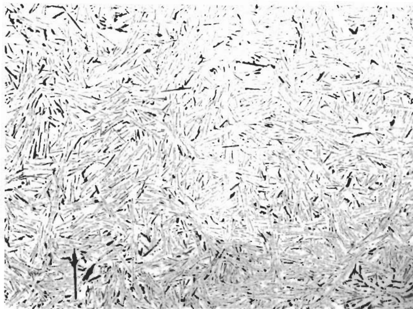
Figure 103. Ti-Mo-C (16-34-50 At.%), Quenched from Liquidus Temperatures.
