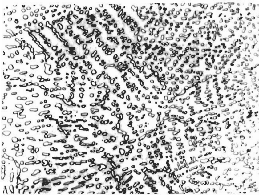
Figure 63. Ti-Ta-C (53-40-7 At.%), Quenched from Liquidus Temperatures. X1000 Metal + Monocarbide Eutectic-Like Structure.
