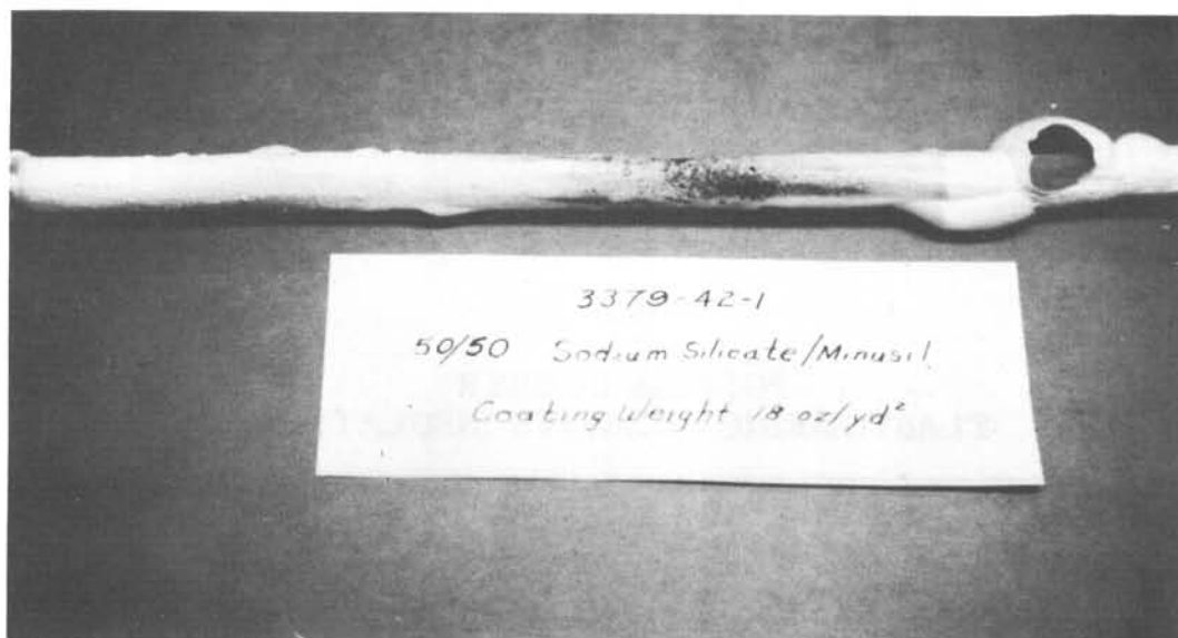
Figure 9. Sodium Silicate Coating after Test
