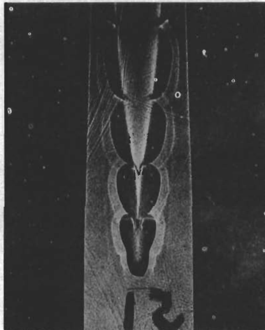
FIGURE 13-18. SHADOWGRAPH OF V-FLAME IN COMBUSTION CHAMBER. d = 0.125 IN., V = 15 FT PER SEC
