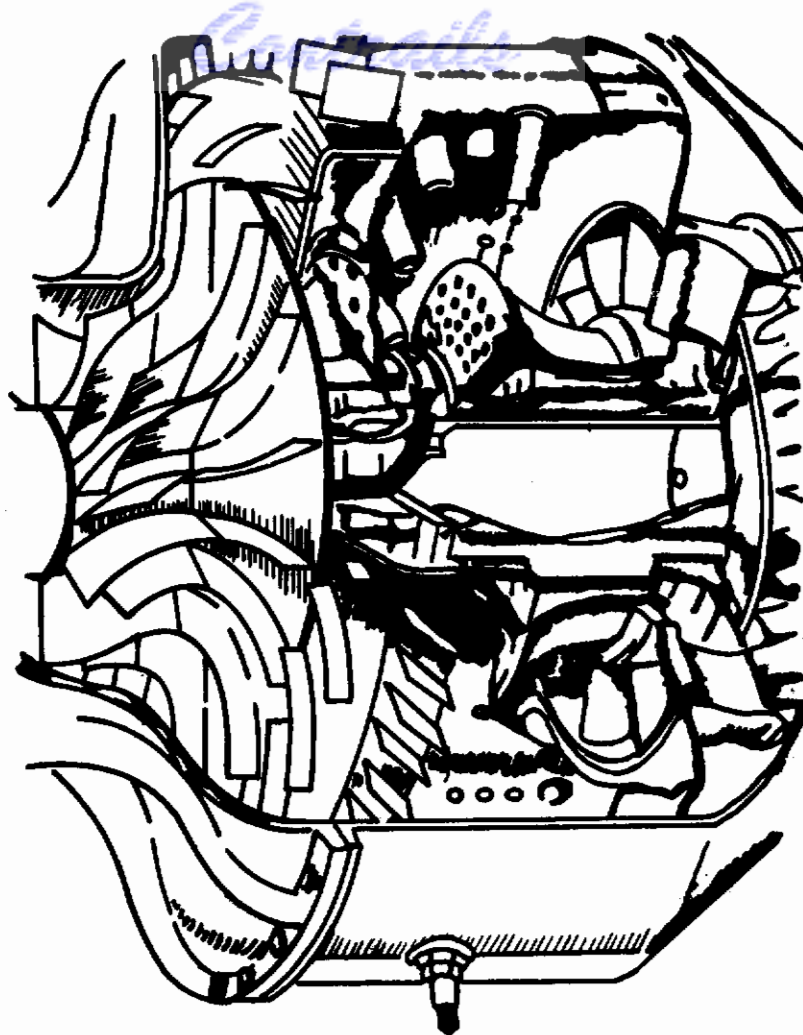
FIGURE 2-14. ROTATING FUEL INJECTION SYSTEM USED BY TURBOMÉCA (2-19)
