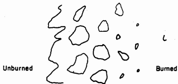
FIGURE 15-6. SCHEMATIC DIAGRAM OF HIGHLY TURBULENT FLAME
