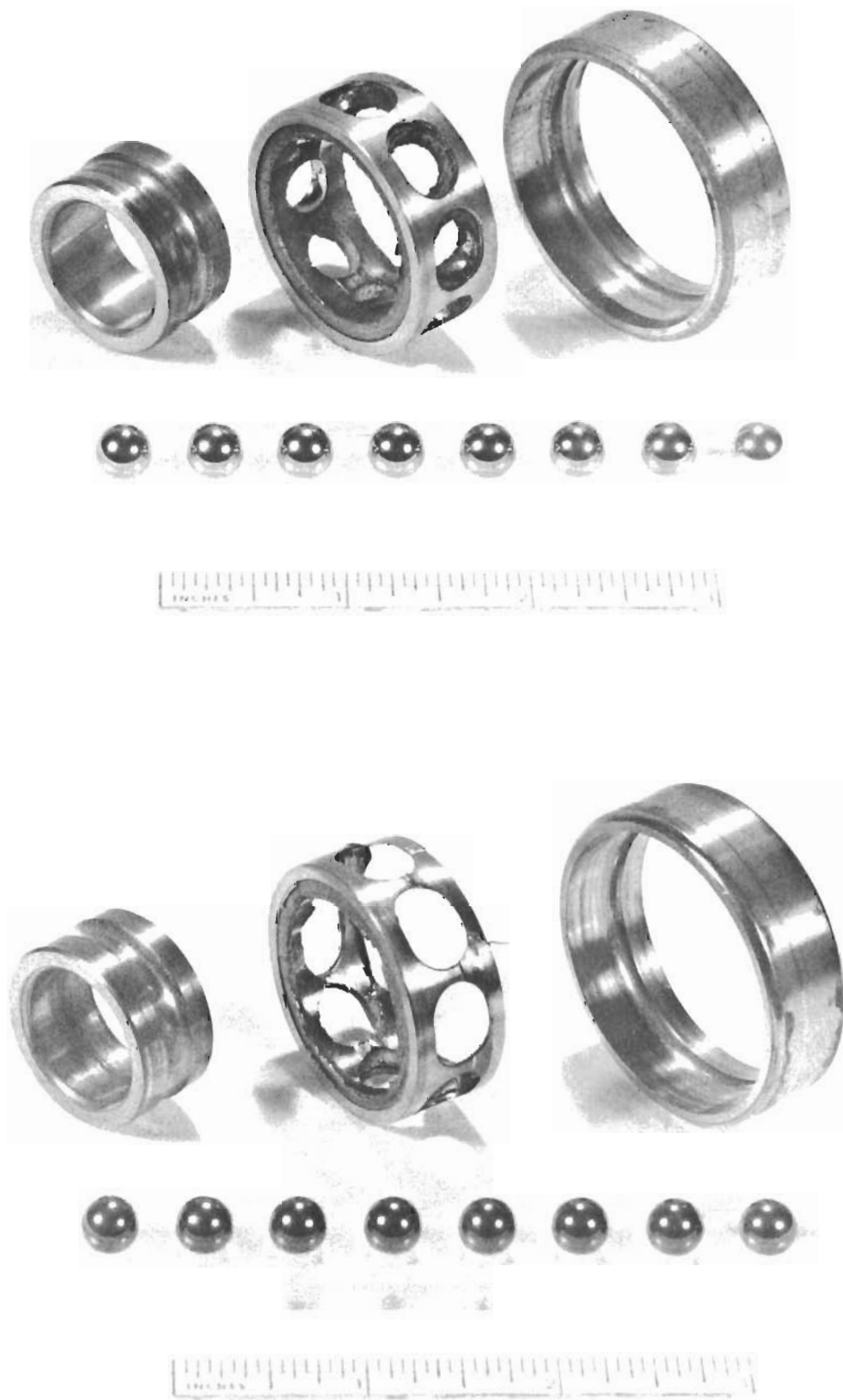
Fig. 9—Run 10 — 204 size bearings from 3/4 H. P. motor after 5058 hrs. at 3,400 rpm and ~ 240,000 ft. altitude
