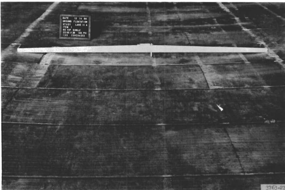
Figure 9. Lane 11A, item 1. Transverse straightedge shows deformations at 130 coverages (failure)
