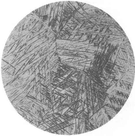
Fig. 6 Ti-3%Al-6%Cr. Center of \frac{1}{2} -in. Bar. 1000°C-20min/W.Q. VHN=260 100X.
