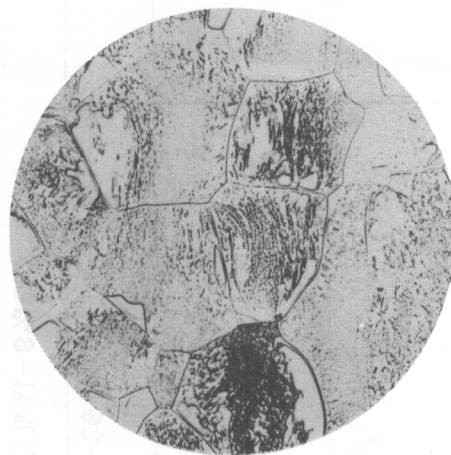
Fig. 27 Ti-3%Al-10%Cr. Center of \frac{1}{2} -in. Bar 1000^{\circ}\text{C} -20min/ 400^{\circ}\text{C} -5min/W.Q. VHN=320. 100X
