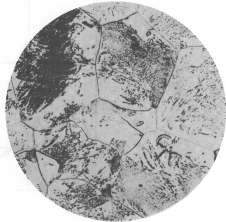
Fig. 18 Ti-12%Cr. Center of \frac{1}{2} -in. Bar. 1000°C-20min/400°C-5min/W.Q. VHN=300. 100X.
