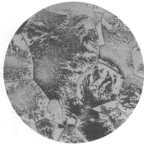
Fig. 16 Ti-10%Cr. Center of \frac{1}{2} -in. Bar. 1000°C-20min/400°C-5min/W.Q. VHN=475. 100X
