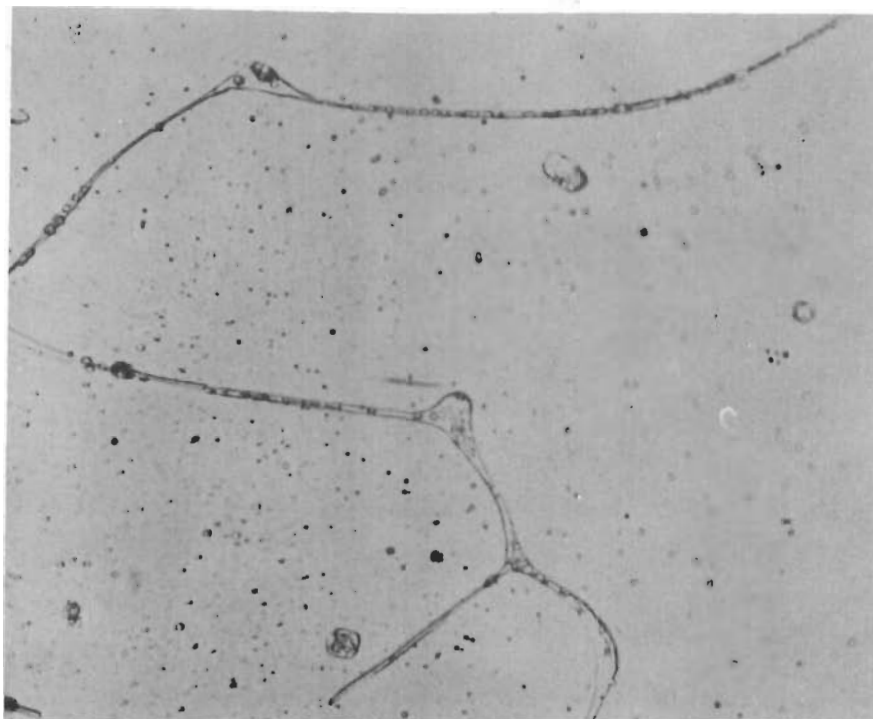
Fig. 12. 0.78 atomic per cent boron. Quenched from 1000°C. Electromechanically etched. x 800
