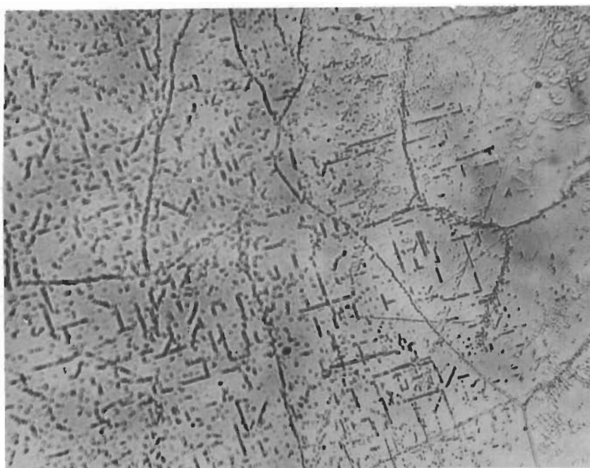
Fig. 19. Substructure in 0.32 atomic % B-W alloy. x 400
