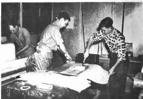
FIG. 20.026.1 PREIMPREGNATION OF GLASS MAT BY HAND JUST PRIOR TO PRESS MOLDING (LUNN LAMINATES)
