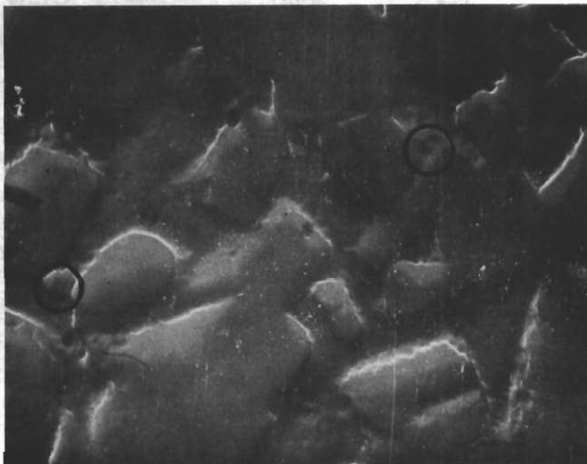
Figure 48. K-152-B As-sintered. Fine particles of TiC in Ni phase are circled.
