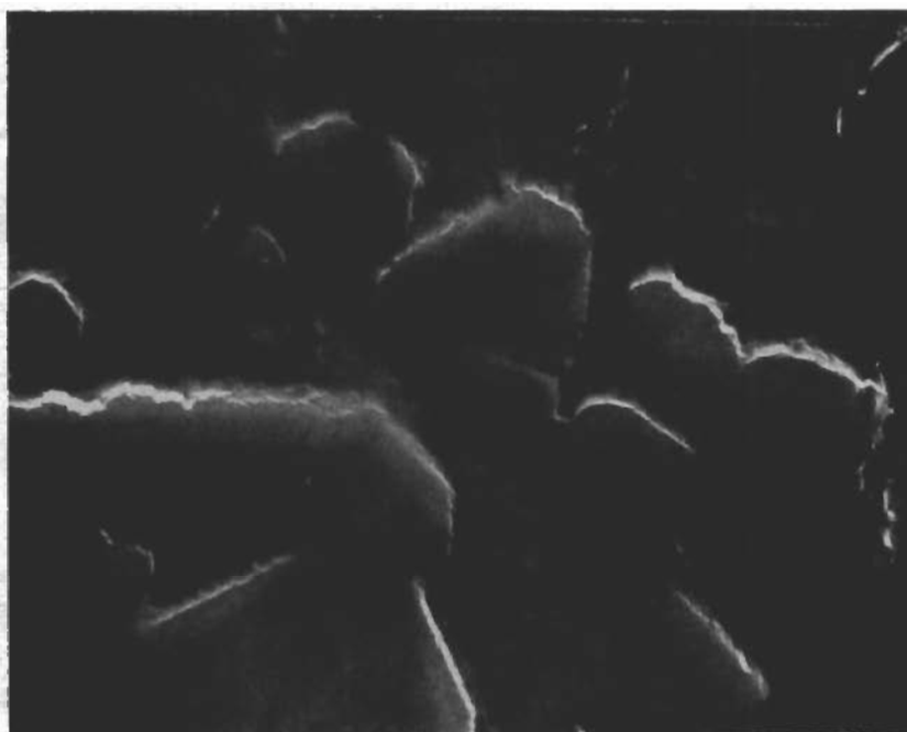
Figure 43. K-152-B As-sintered. Fine particles of TiC in Ni phase are circled.
