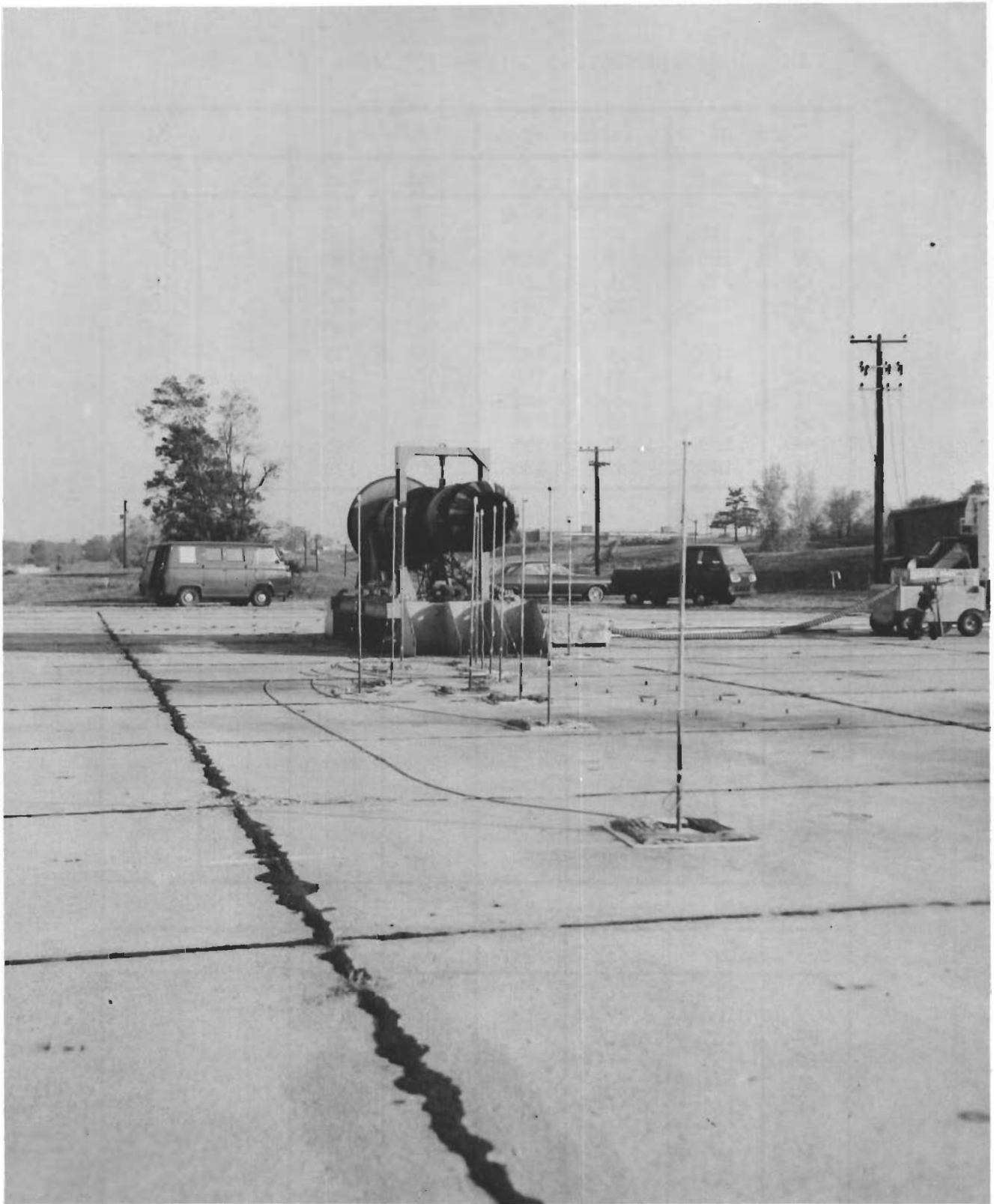
Figure 2. Typical Setup of Twelve Microphone Locations
