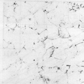
Fig. 14. Ti 75A Same Treatment as (12) + 27.8 hrs at 1000°F and 6,500 psi - X250D
