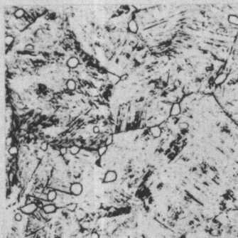
Fig. 33. Ti 150A 1 hr at 1800°F + 1 hr Iso. Trans. at 1000°F + Water Quench - X500D Etchant: 1 HF, 1 Glycerine
