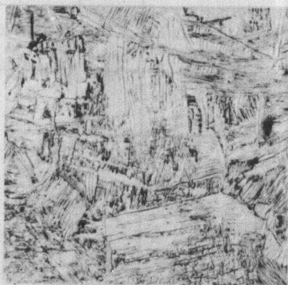
Fig. 52. 6% Al \alpha Alloy 2025°F Water Quench + Tensile Test at 1000°F - X100D
