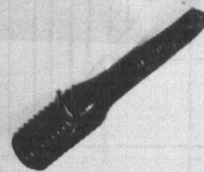
(1 hr 1325°F + Water Quench) 1000°F 40,000 psi 74.5 hrs 54.4% Elong. 37.9% Red. Area
