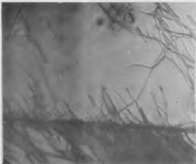
Figure 7. Section showing sub grain boundary. (x 15,000)
