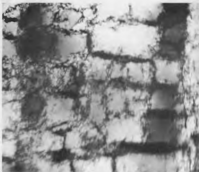
Figure 9 Crystal deformed at 78°K. Double glide orientation. (x 15,000) (Basinski & Dove, to be published.)
