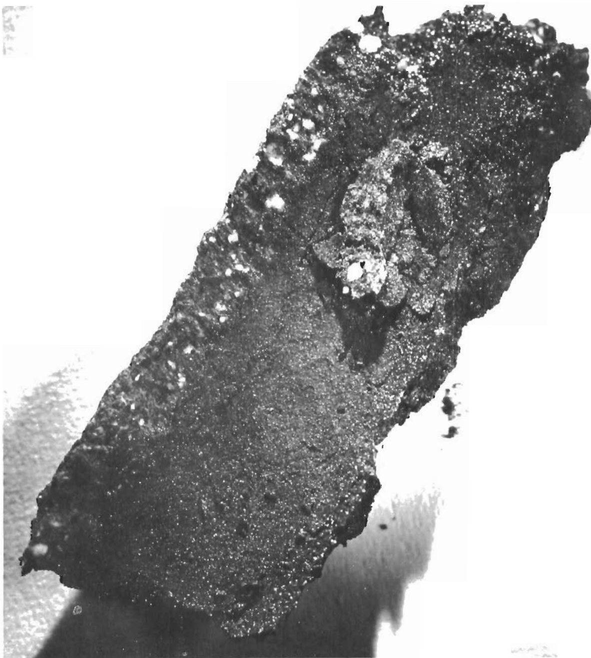
ADL-17 Powder After Heating to 2000 0 F for Several Days
