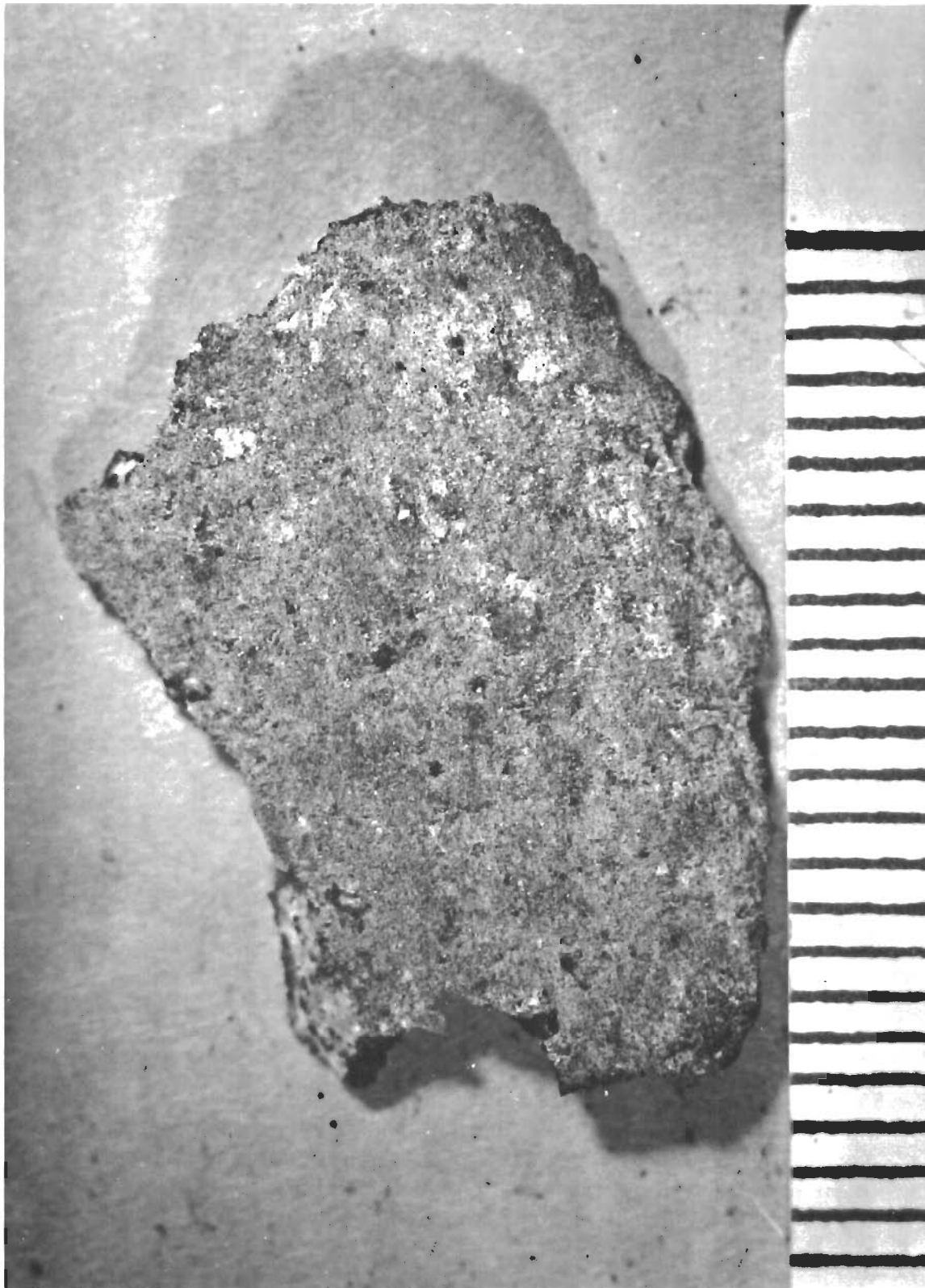
ADL-17 After Heating to Over 2200°F for Two Weeks
