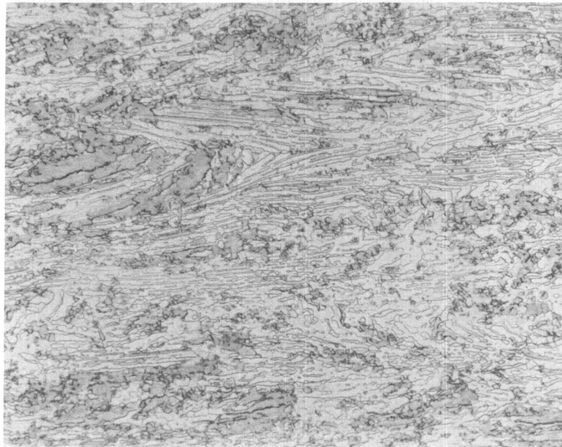
FIGURE 26. MASSIVE HYDRIDE IN Ti-2Mn-2Fe (K-24) CONTAINING 200 PPM HYDROGEN
