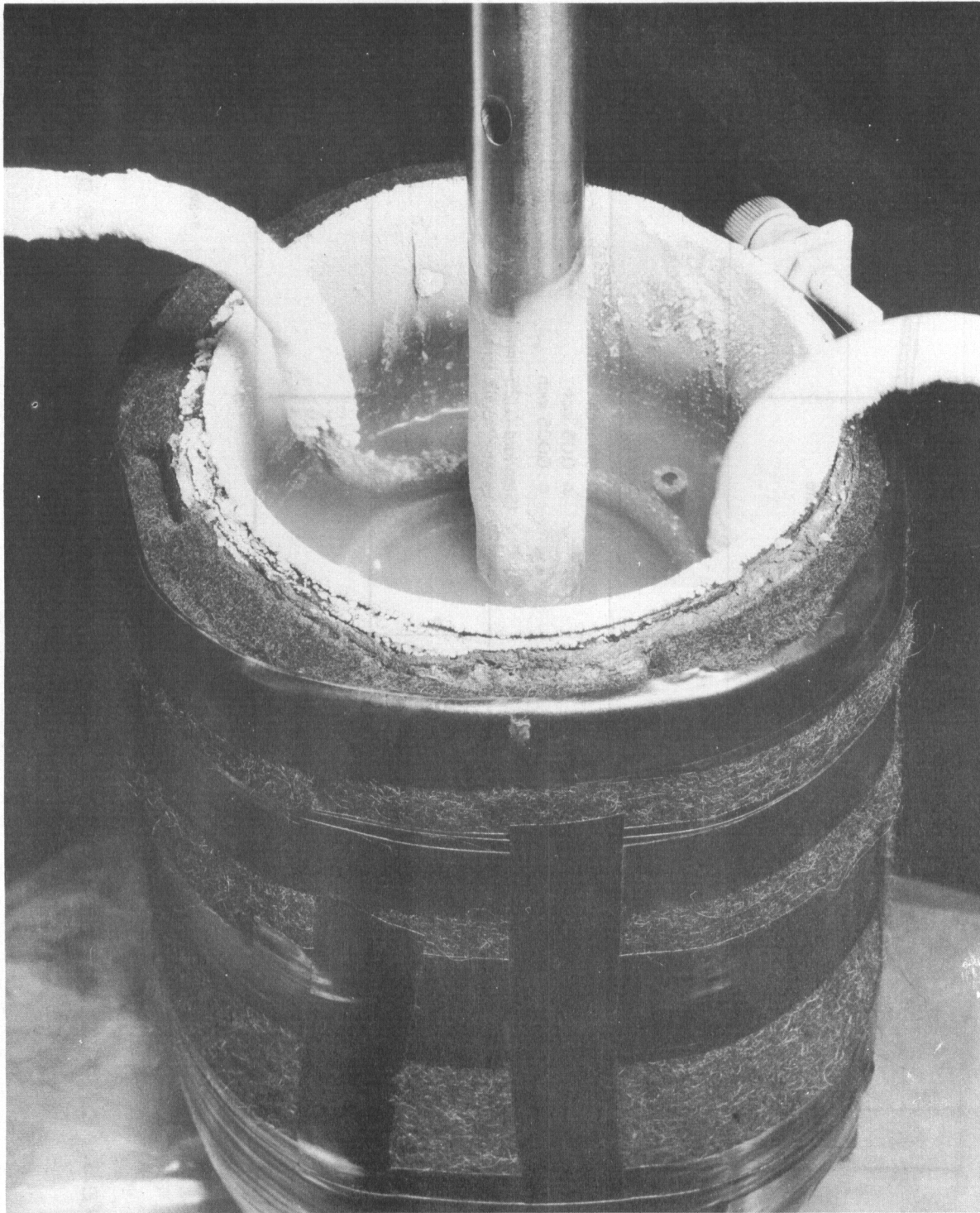
FIGURE 2. CLOSE-UP OF ISOPENTANE BATH AND COOLING COIL
