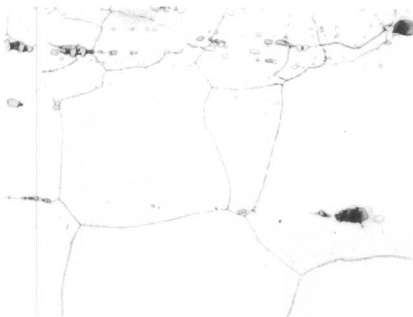
a. Specimen No. 44. Sample taken from "as received" end of test bar. Longitudinal section, etched with mixed acids, 95-3-2; 1000X.
