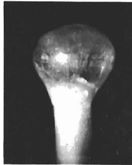
Figure 7. Two views of a spinel boule grown in the R. F. plasma crystal growth facility utilizing a polycrystalline seed and minus 200-mesh arc-fused spinel feed material.
