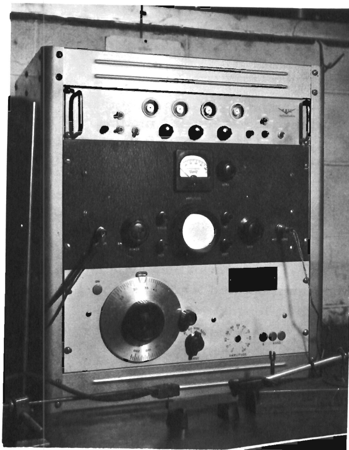
Figure 2. Apparatus for Measuring Young's Modulus at Room Temperature
