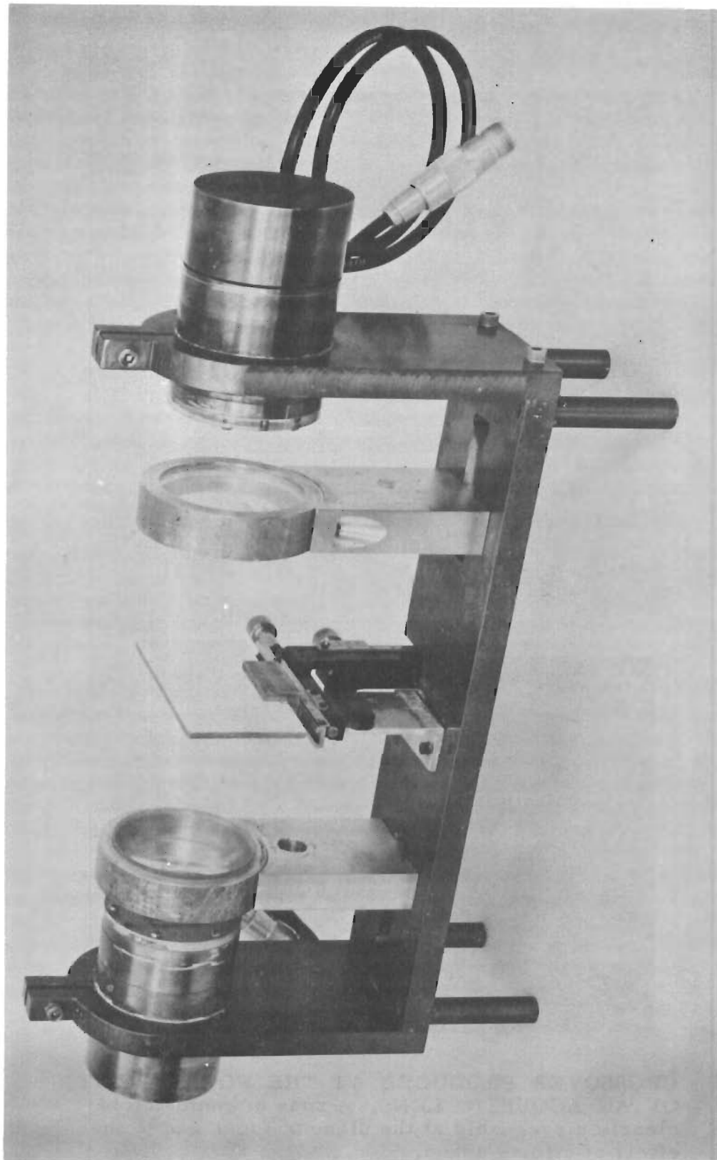
Fig. 13 - ACOUSTIC LENSES. The lenses are mounted with their plane surface toward and parallel with each transducer element. The specimen traverse mechanism, located midway between transducers, is horizontally and vertically adjustable. The focal point of both lenses is adjustable over one inch.
