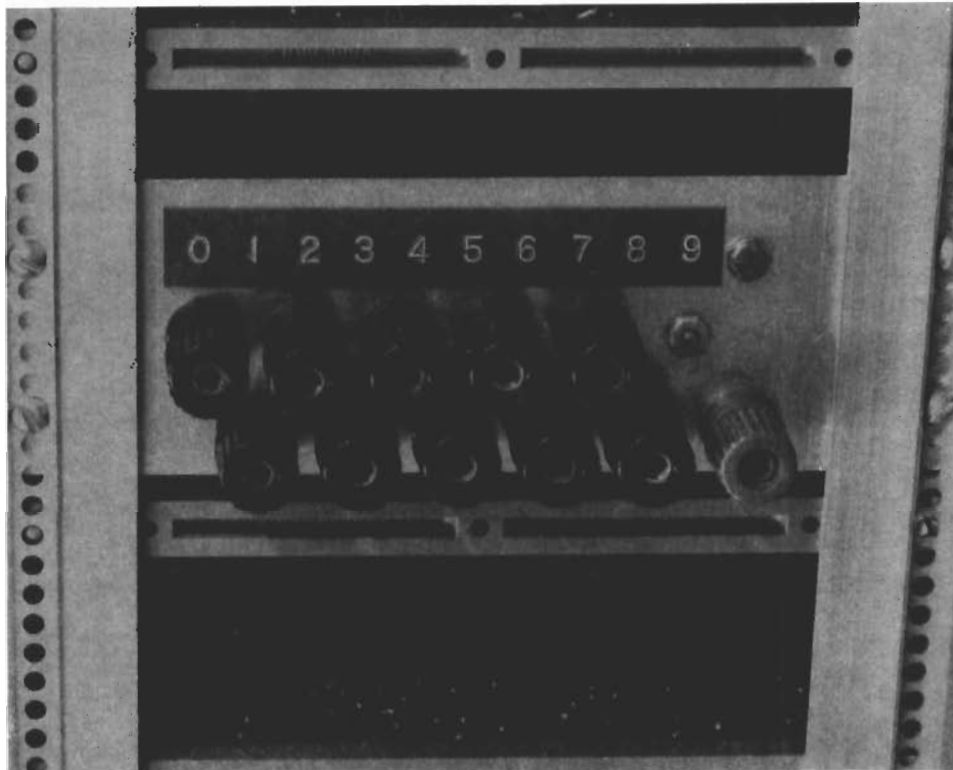
Figure 7. Patch Panel Inside Top Cover
