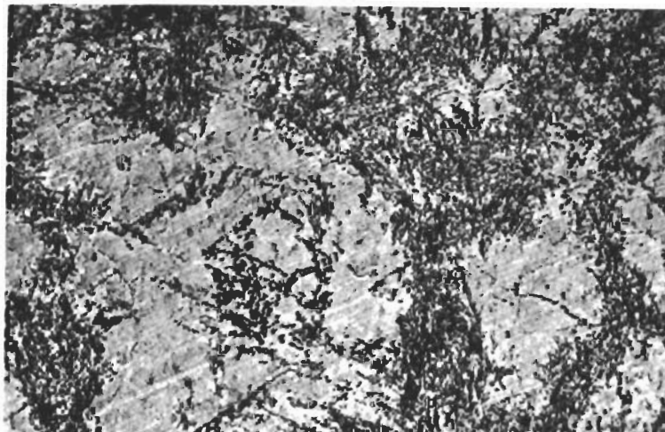
600X Etchant: 2% Nital R3131 (b) Heat Affected Zone Structure
