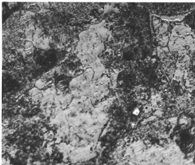
600X Etchant: 5% Nital R3179 a) Heat-Affected Zone Structure
