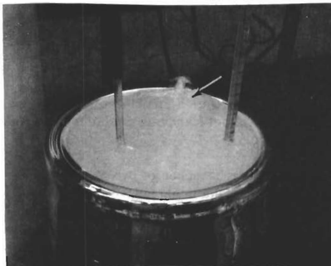
Fig. 5. Two 1x3" slides plunged into -4.0^{\circ}\text{C} alcohol-ice bath. The slides are contained in an evacuated polyethylene bag.
