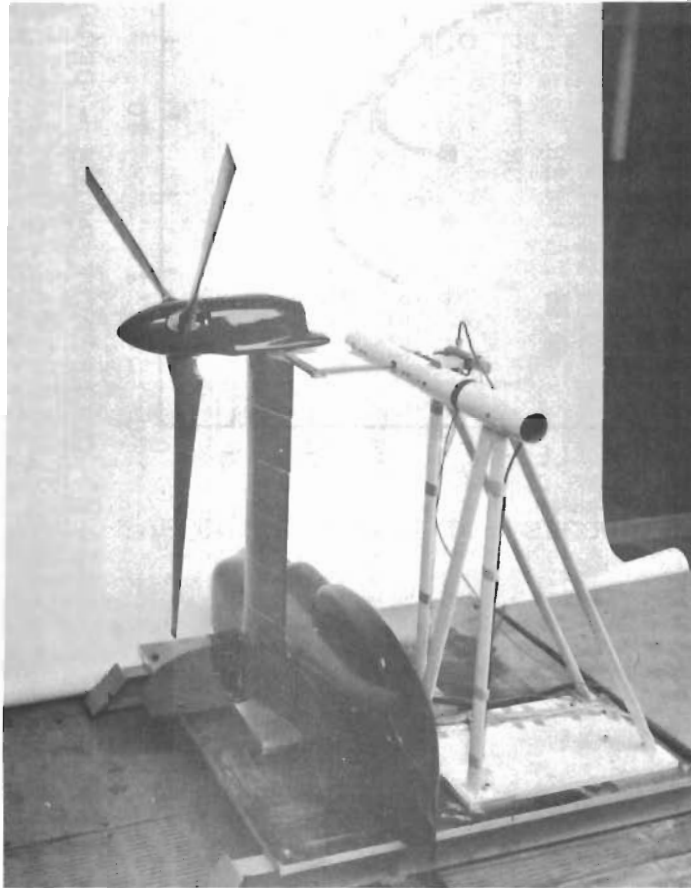
Figure 22. 1/10-Scale M160 Dynamic Model
