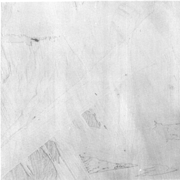
Neg. No. 3752 X 75 Fig. 66 A 0.8% oxygen alloy quenched from 1700°C. Structure shows an extremely coarse transformation structure.
