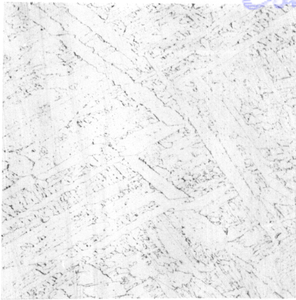
Neg. No. 3903 X150 Fig. 64 A 0.2% oxygen alloy quenched after 48 hours at 950°C, showing a serrated \alpha type of transformation structure.
