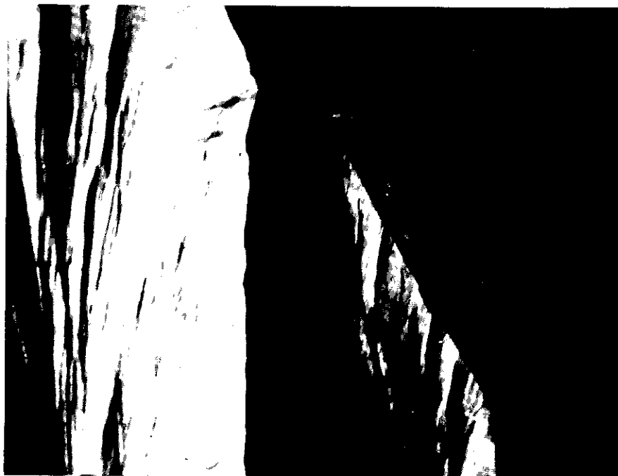
After Annealing, Density 2.208 g/cc
