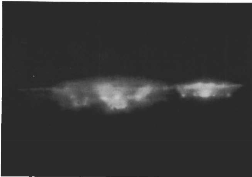
Figure 26. Discharge Between Plane Polished Surfaces of the Two Halves of a 10 K, 2 Watt Carbon Resistor, Gap Distance = .0025 Inch. Some RF Radiation Observed Due to Contamination.
