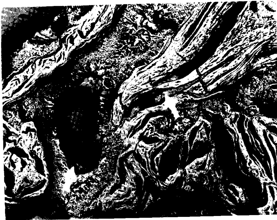
Figure IV.7. AX Coke, Calcined to 1350°C, Pitch Treated and Recalcined to 525°C, 100X N-4533
