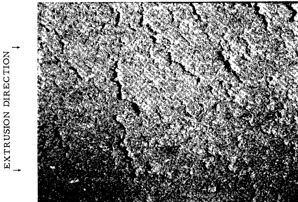
Figure VI.5. Extrusion with 200 lbs. Back Pressure, Sawed Surface Showing Flow Line Patterns 45° to Direction of Mix Flow, 9X
