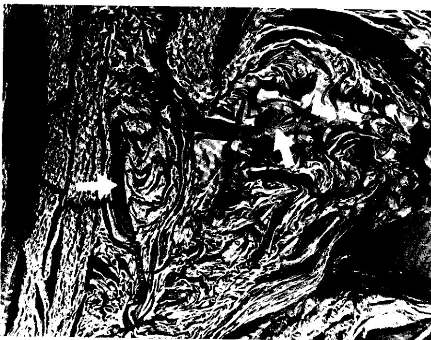
Figure IV.6. AX Coke, Calcined to 1350°C, Pitch Treated and Recalcined to 500°C, 100X N-4532
