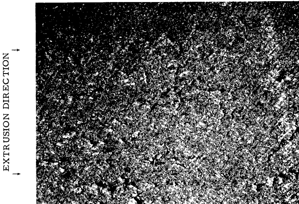
Figure VI.6. Extrusion with no Back Pressure, Flow Lines Approximately Parallel to Direction of Mix Flow, 9X
