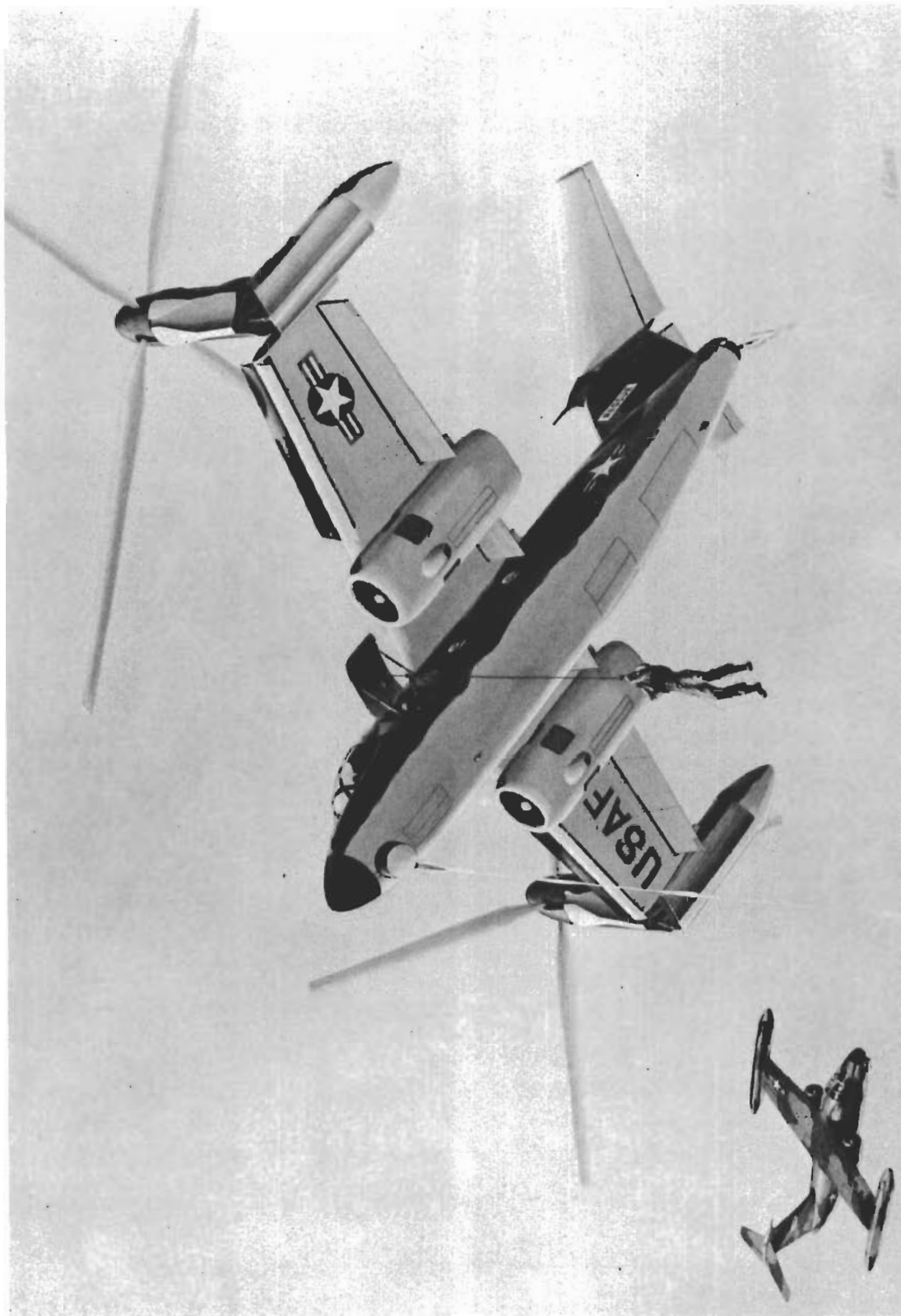
FIGURE 1.2 STOWED TILT ROTOR RESCUE AIRCRAFT
