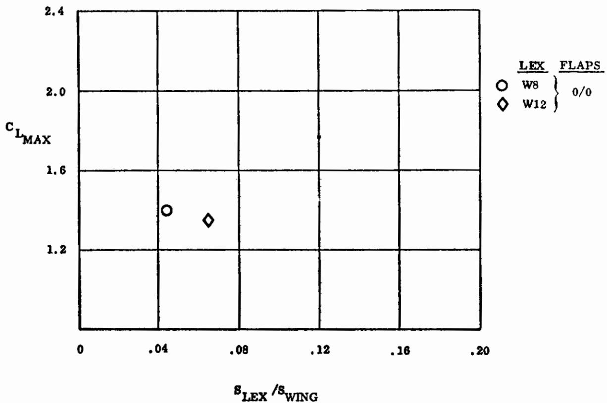
Figure 224. Effect of Lex Planform on  $C_{L_{MAX}}$
