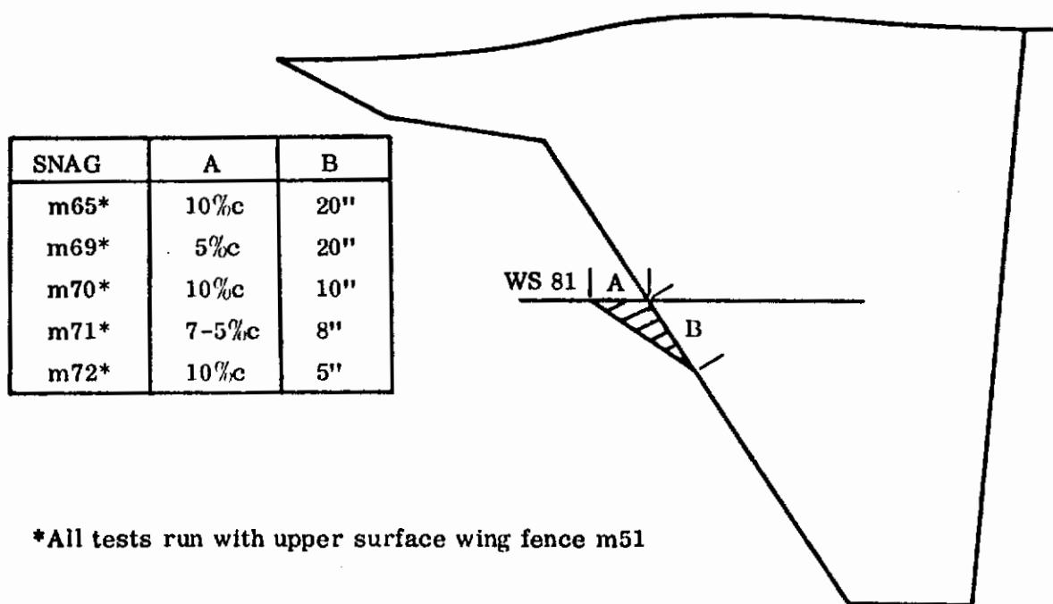
\*All tests run with upper surface wing fence m51
