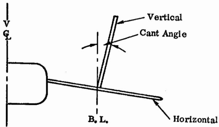
Figure 30. Twin Vertical Tail Configurations Mounted on the Horizontal Tail
