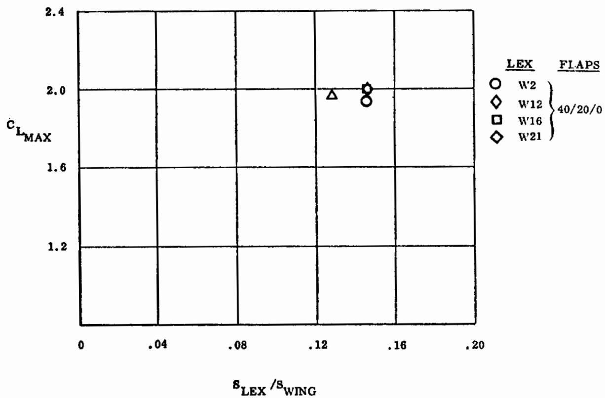
Figure 127. Effect of Lex Cross Section on  $C_{LMAX}$
