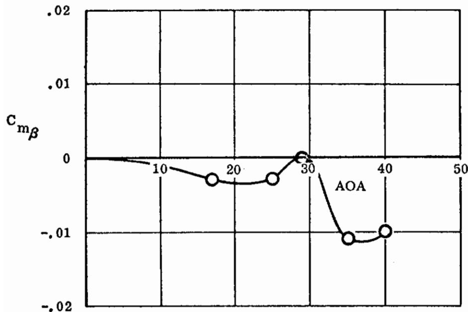
Figure 113. Pitching Moment Due to Sideslip
