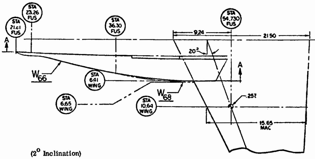
Figure 92. Increasing LEX Span (W66, 68)
