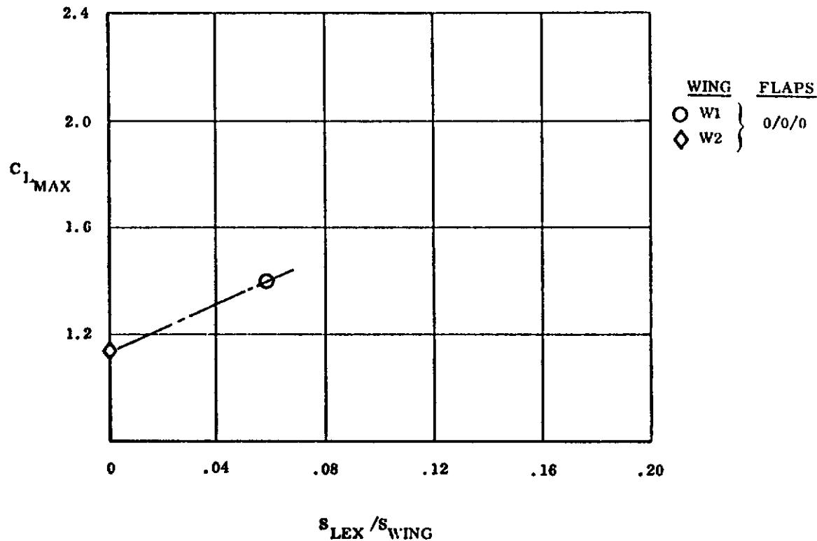
Figure 10. Effect of LEX on  $C_{L\text{MAX}}$
