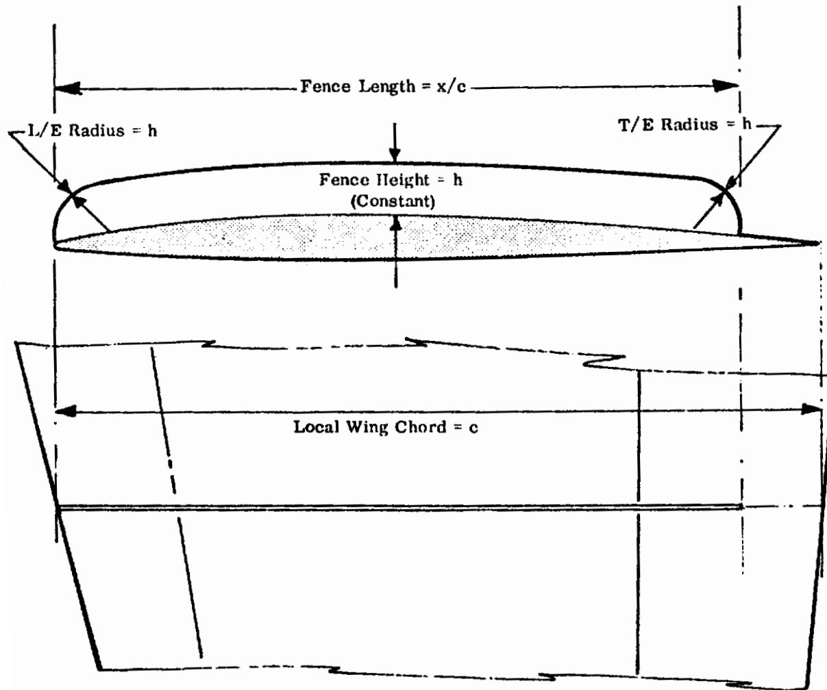
Figure 254. F-5E/F Wing Fence Geometry
