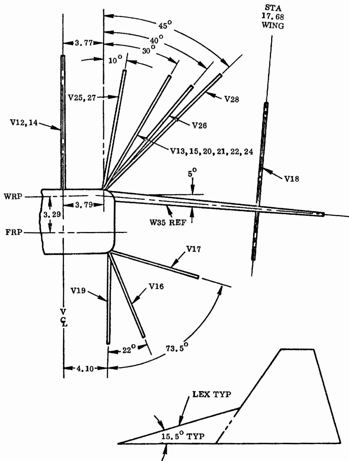
Figure 22. Vertical Tail Size, Shape, and Location
