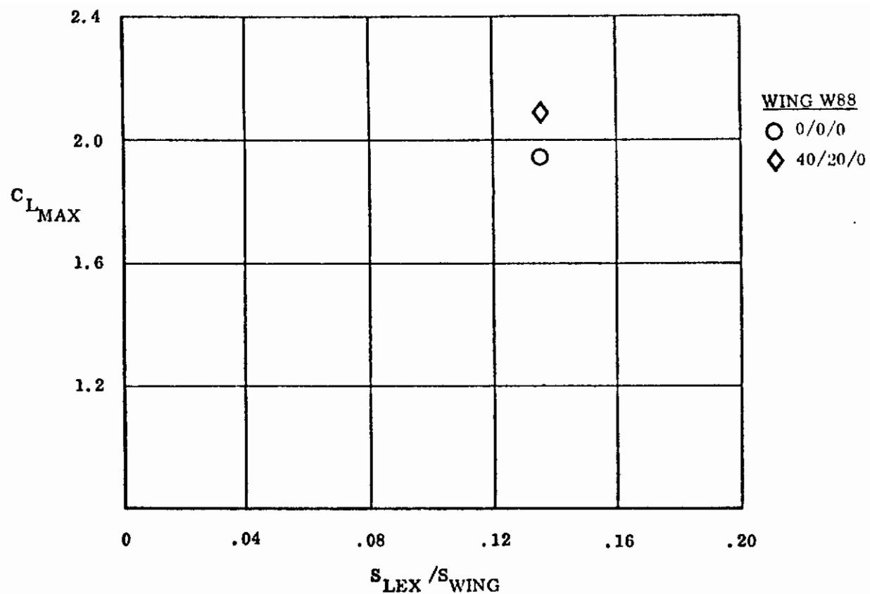
Figure 72. Effect of Flaps on  $C_{L_{MAX}}$
