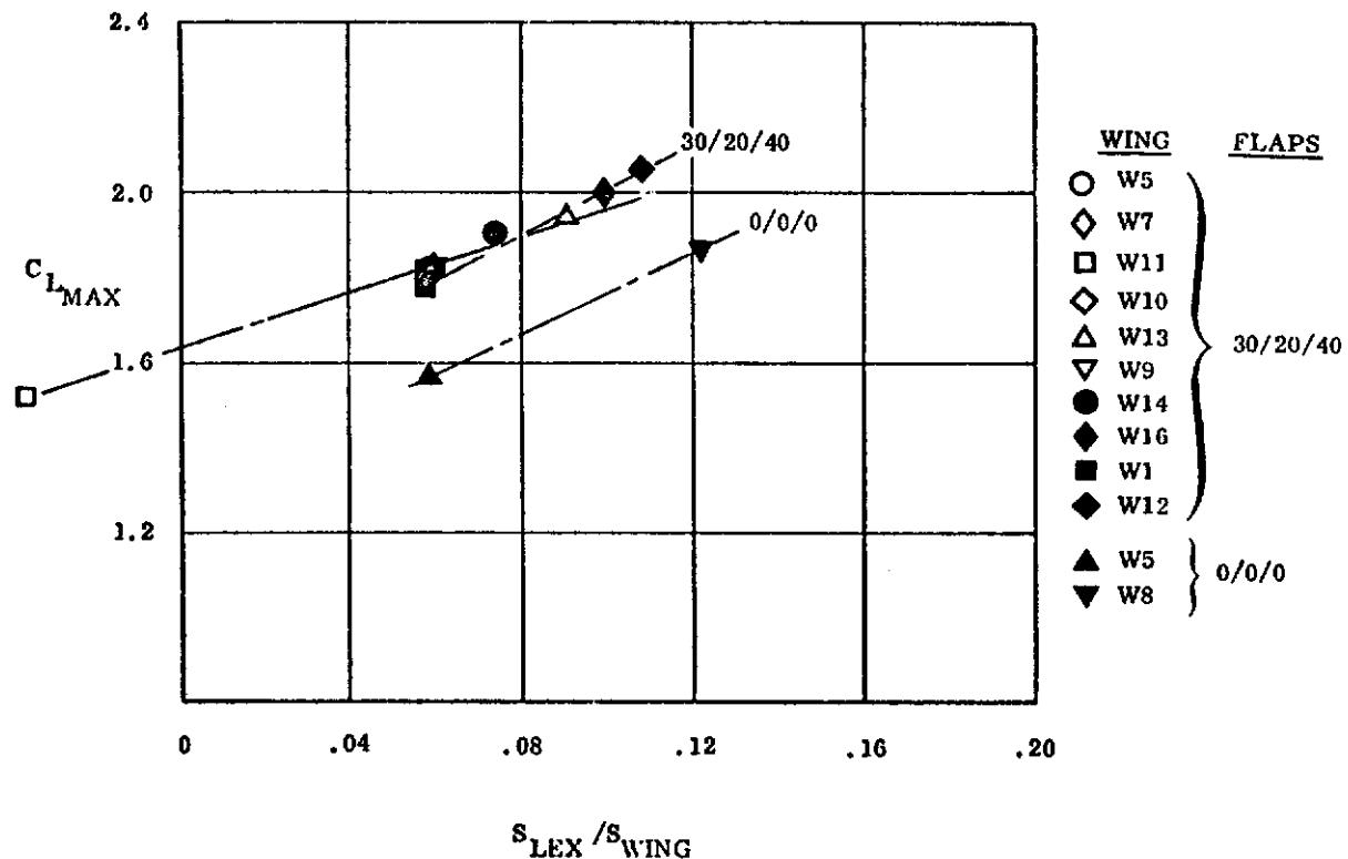
Figure 14. Effect of LEX Airfoil, Effect of LEX Planform on  $C_{L_{MAX}}$
