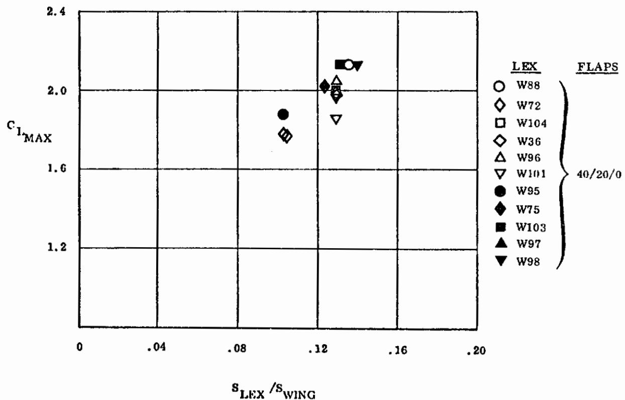
Figure 57. Effect of Various LEX Planforms on  $C_{L_{MAX}}$
