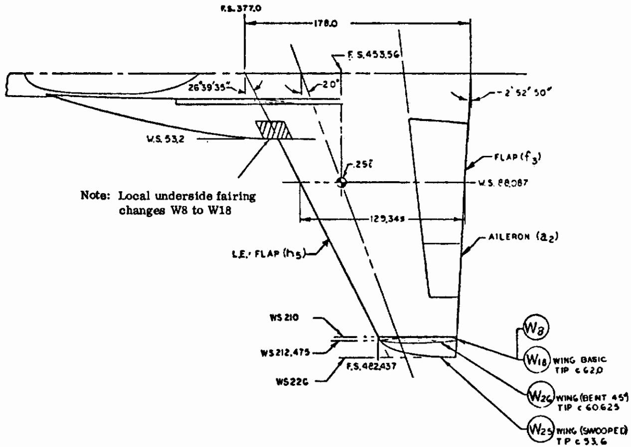
Figure 198. Wing Tips W18, W25, W26
