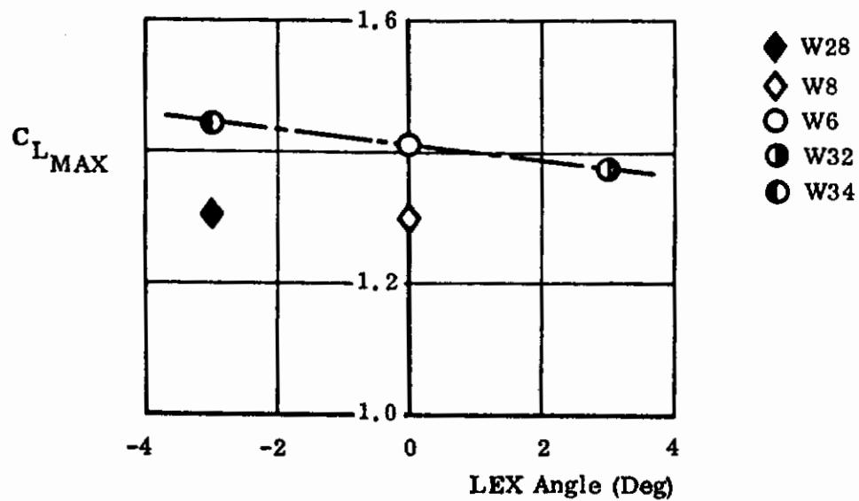
Figure 287. Effect of Lex Angle of Attack
