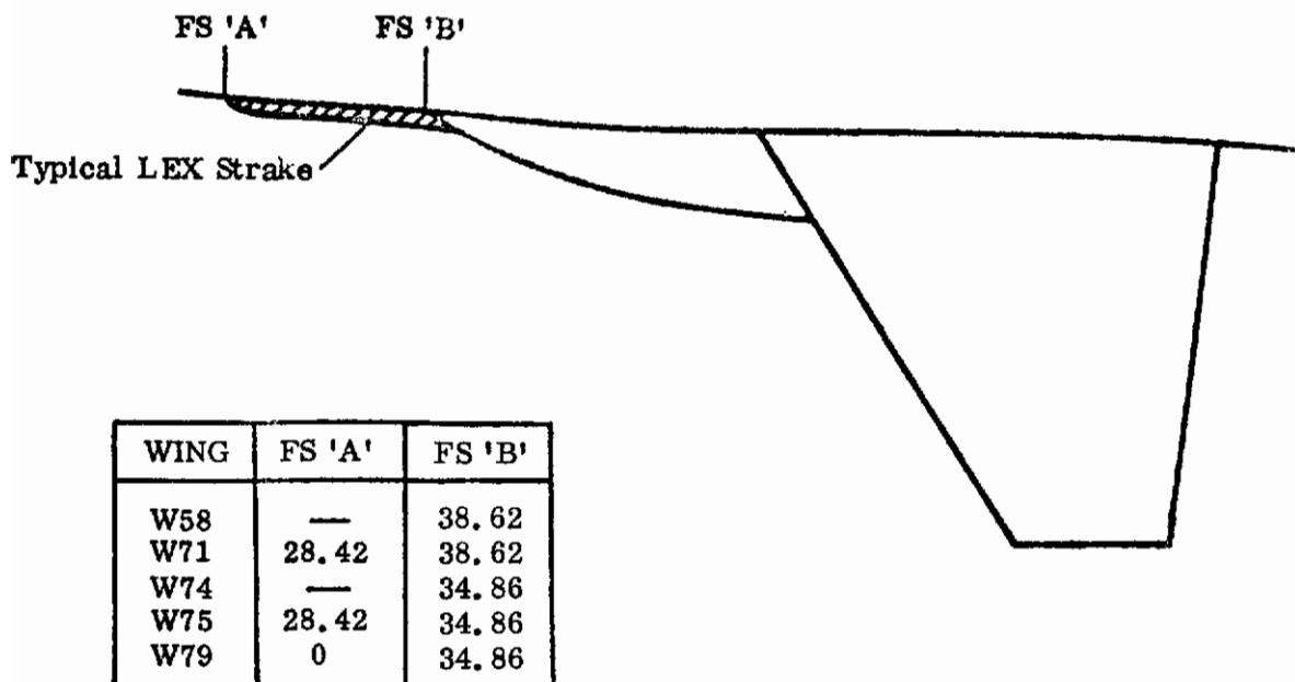
Figure 42. LEX Strake Configurations
