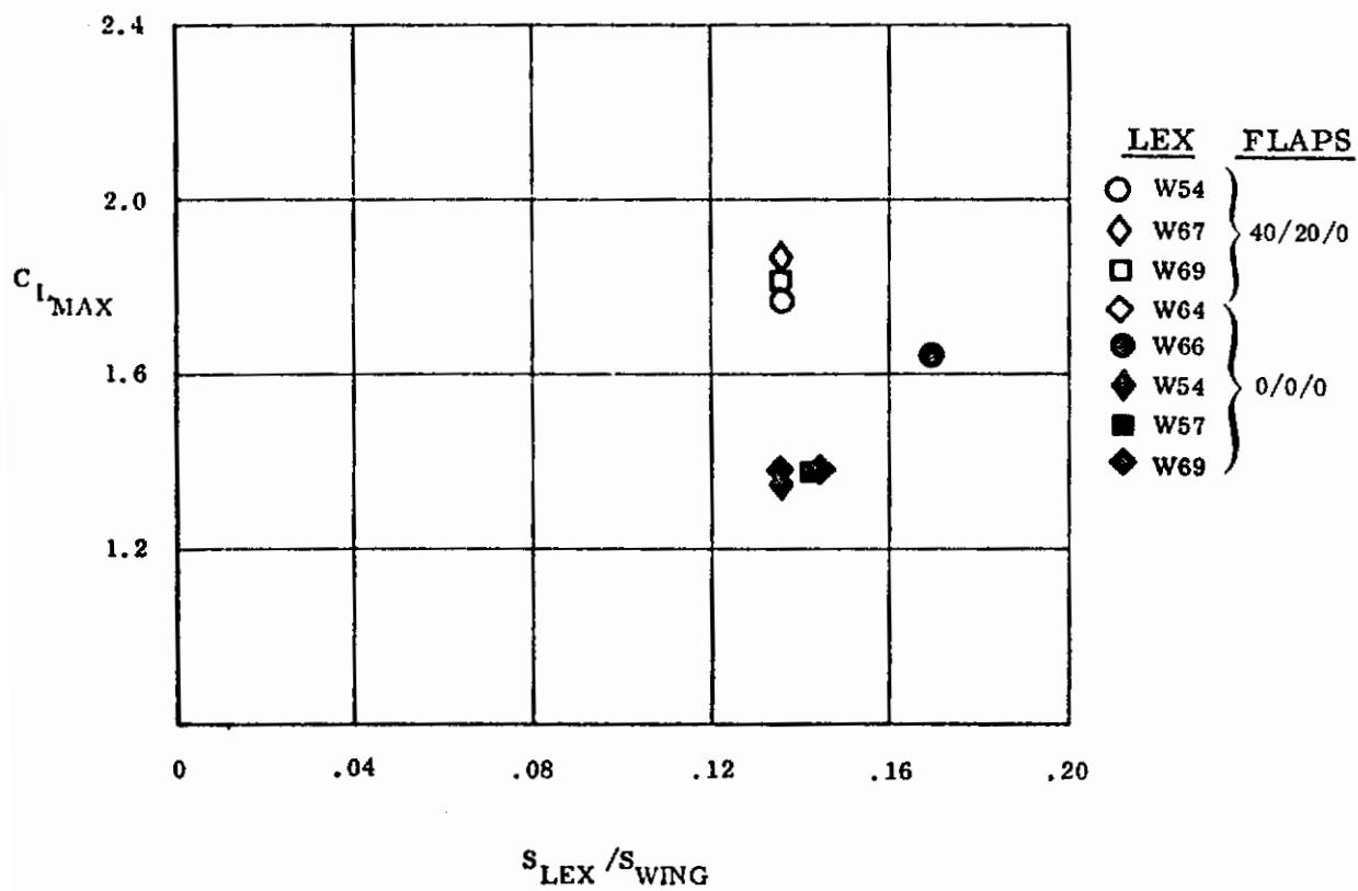
Figure 94. LEX Effects on  $C_{LMAX}$
