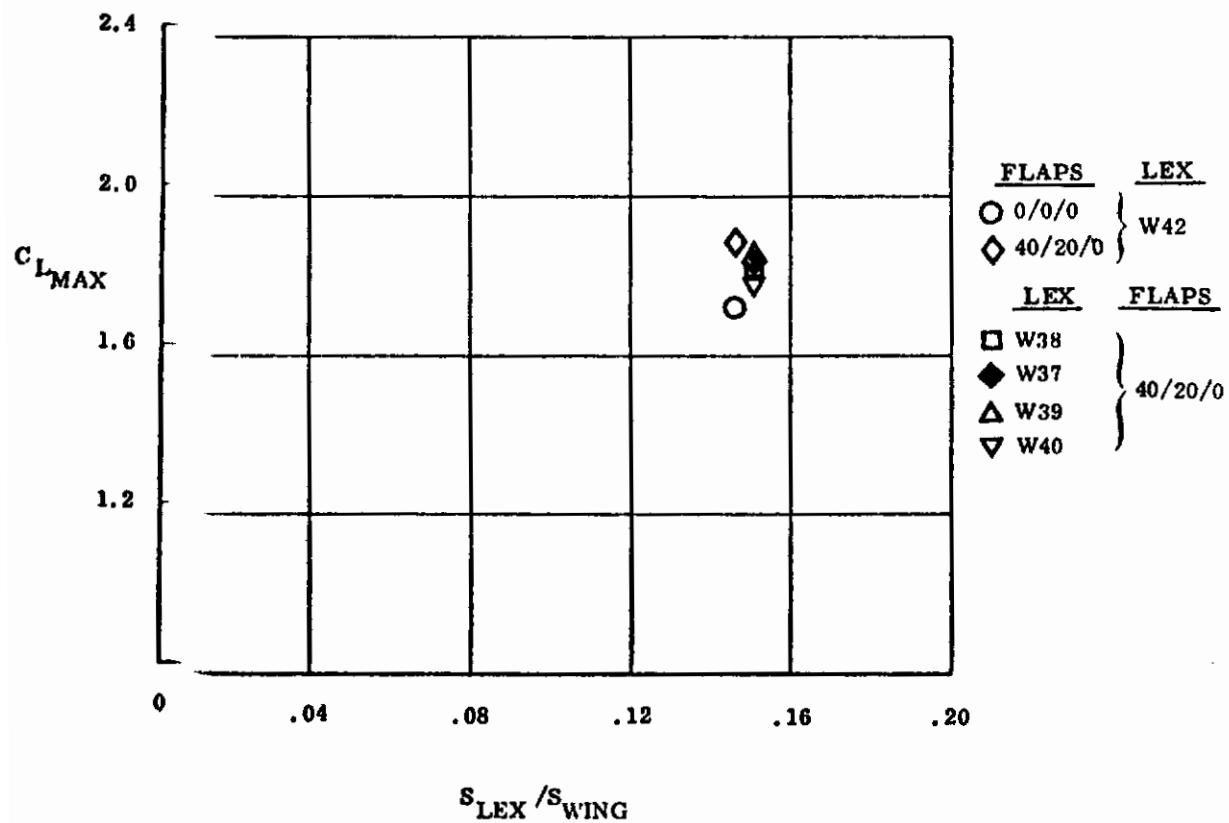
Figure 83. Effect of LEX Planform and Effect of Flaps on  $C_{L MAX}$
