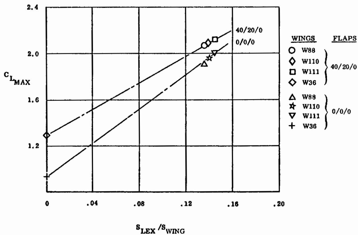
Figure 69. Effect of Small Wing Planform Changes on  $C_{L_{MAX}}$
