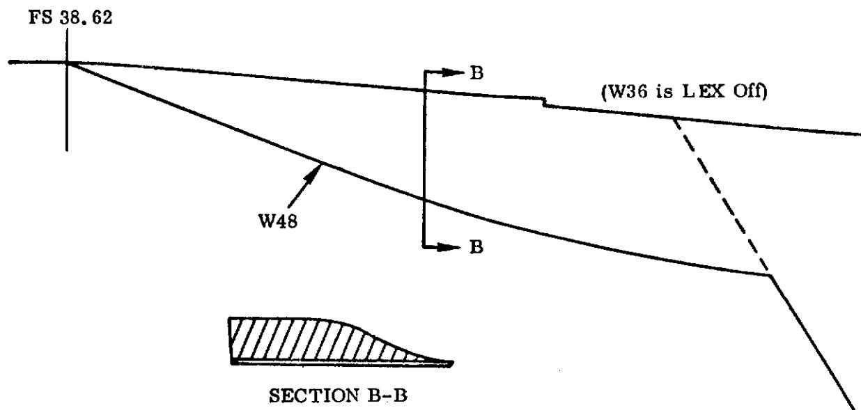
Figure 34. LEX Geometry W48 and W36
