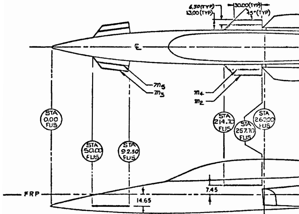
Figure 228. Fuselage Vortex Generators
