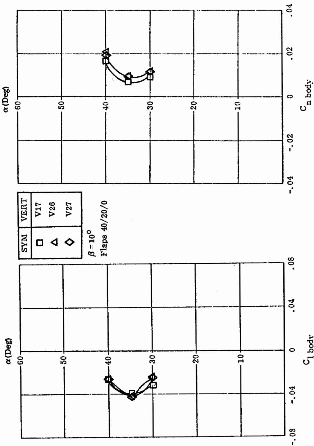
Figure 166. Effect of Vertical Tail Location
