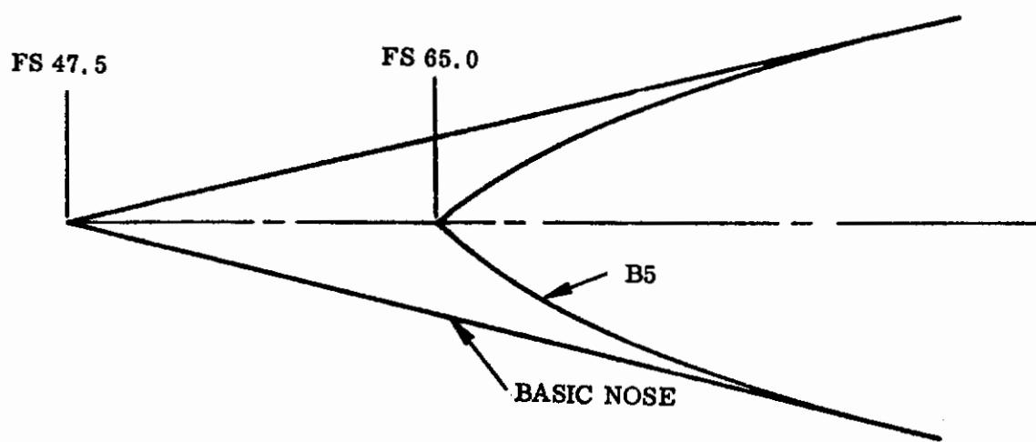
Figure 245. Basic Nose and Blunt Nose B5
