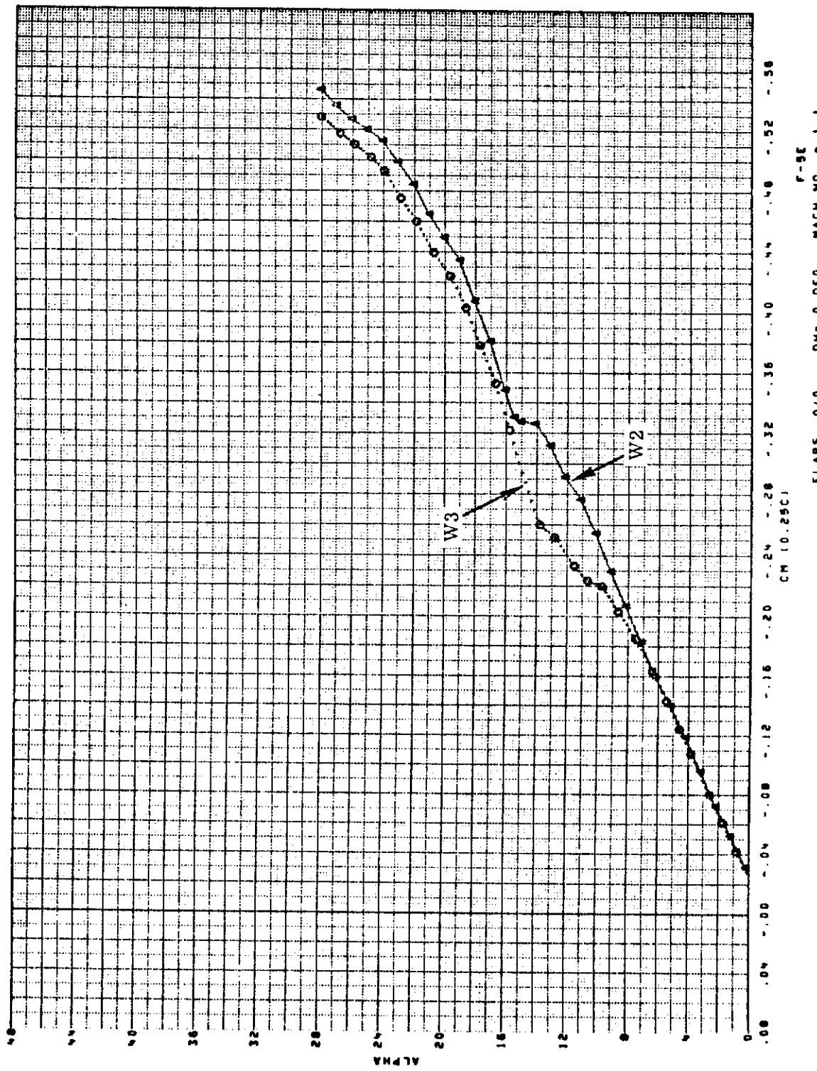
Figure 375. Comparison of Lex W3 and W2 at Mach = 1.1
