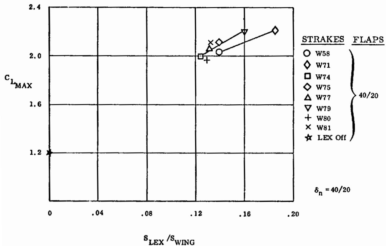
Figure 48. Strake Effects on  $C_{L_{MAX}}$
