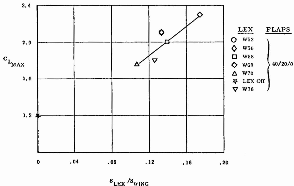
Figure 47. Effect of LEX Geometry on  $C_{L_{MAX}}$
