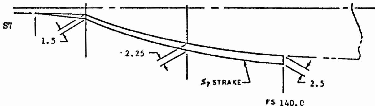
Figure 180. Nose Strake Planforms
