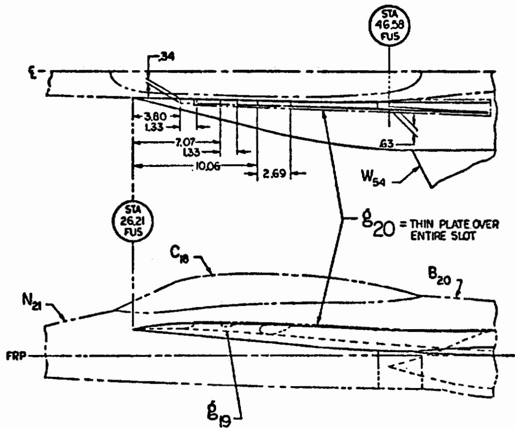
Figure 106. Sealing Lex Gutter (g19, 20)
