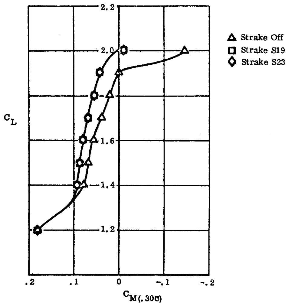
Figure 101. Effect of Nose Strakes
