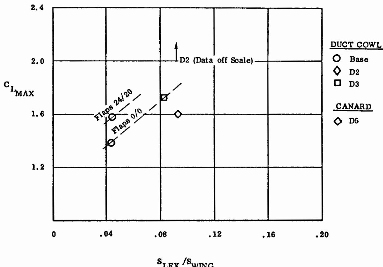
Figure 217. Effect of Duct Cowls and Canard D5
