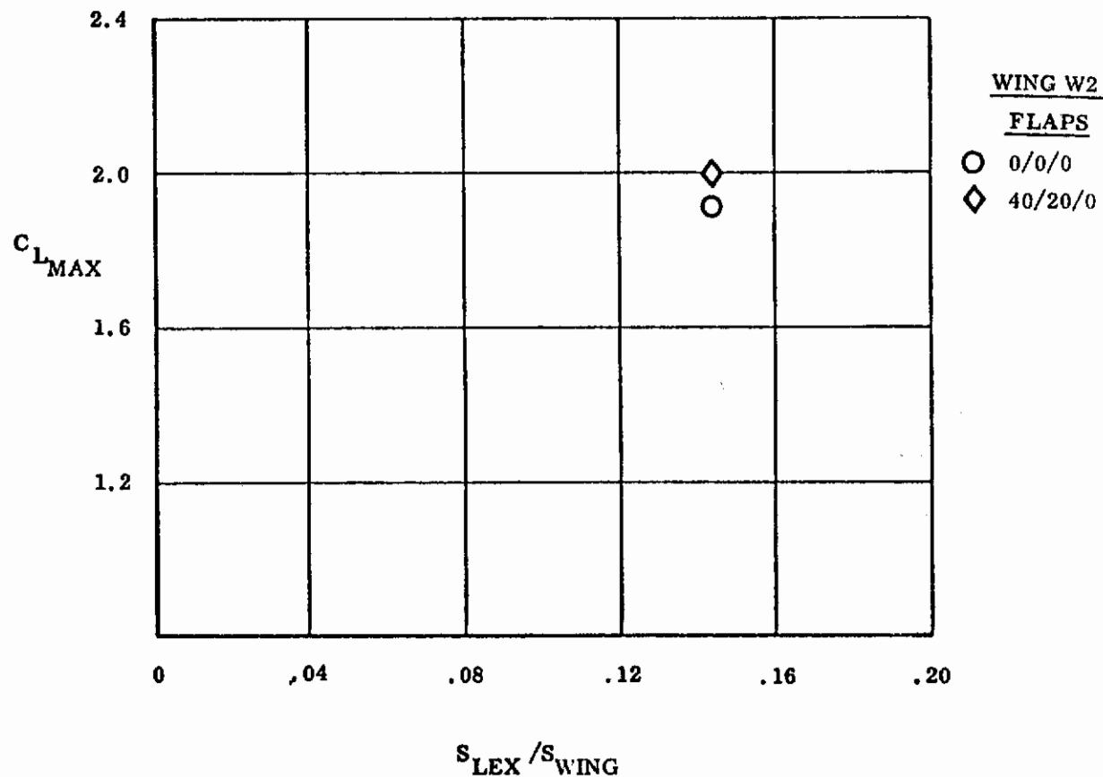
Figure 112. Effect of Flaps on  $C_{L_{MAX}}$
