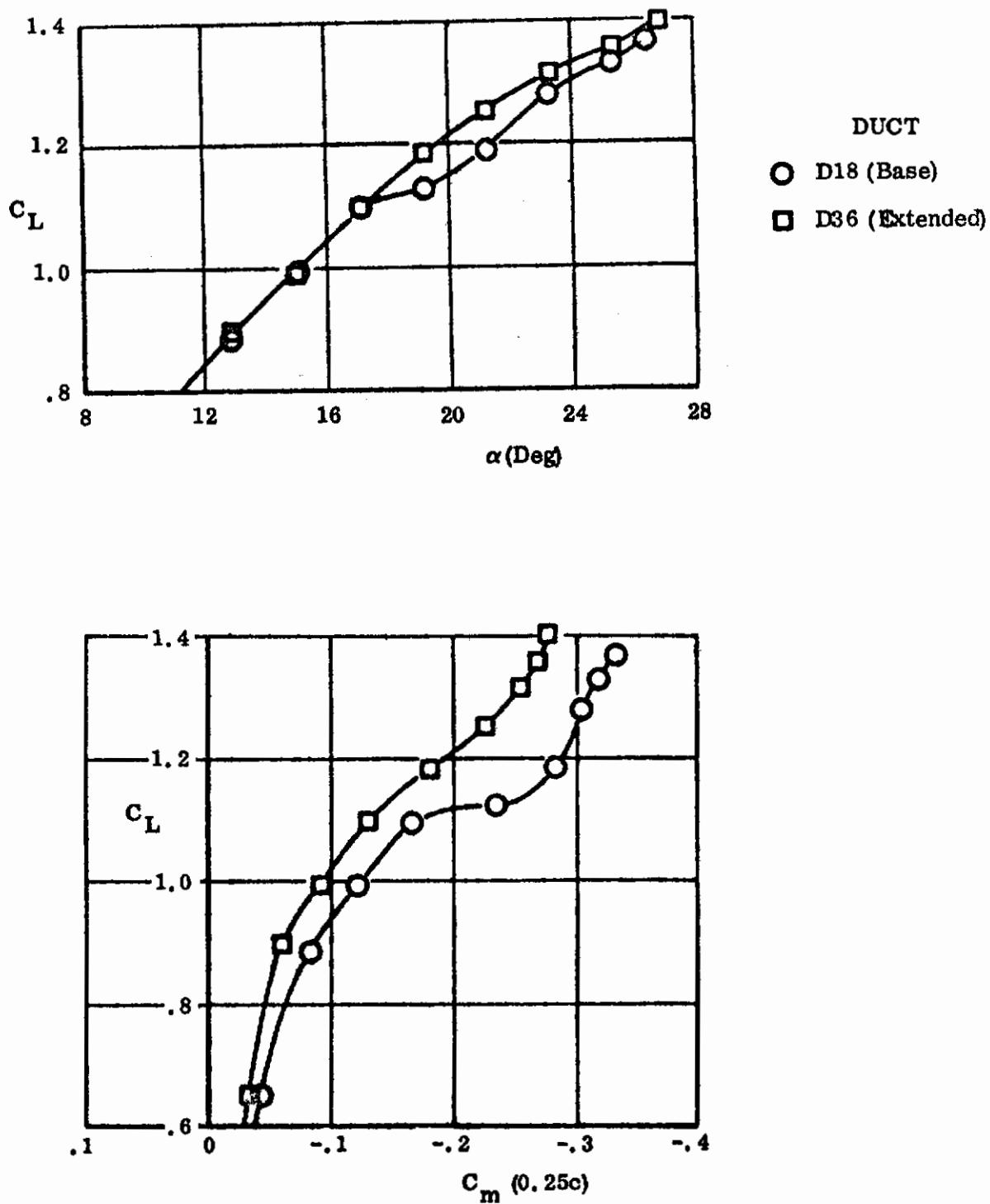
Figure 207. Effect of Duct Extension
