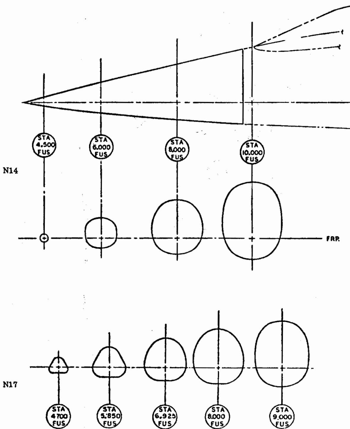
Figure 153. Nose Cross Sections
