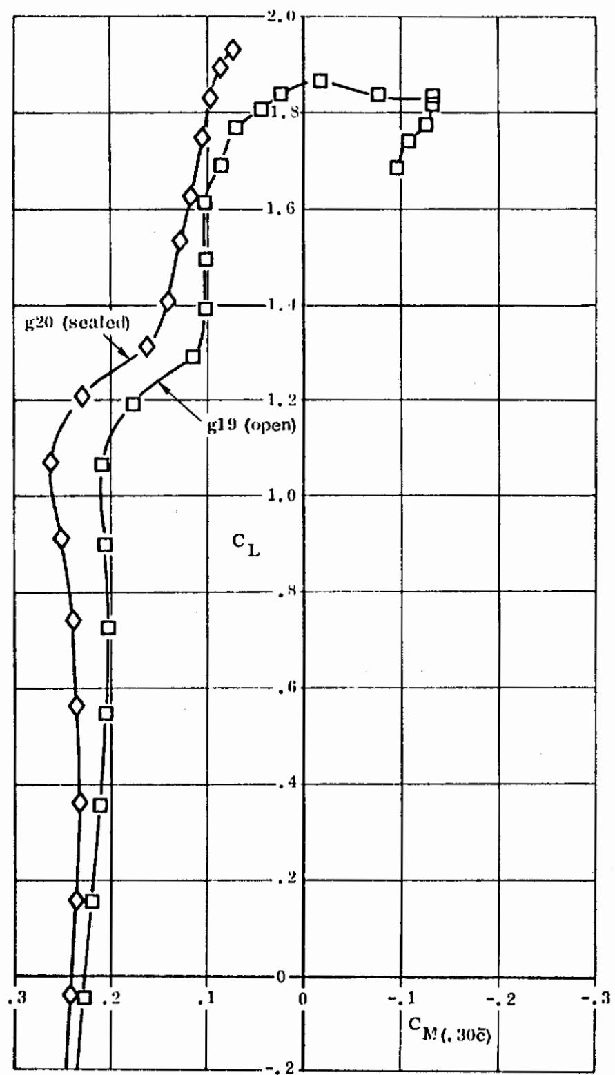
Figure 107. Effect of Sealing Lex Gutter (g19, g20)
