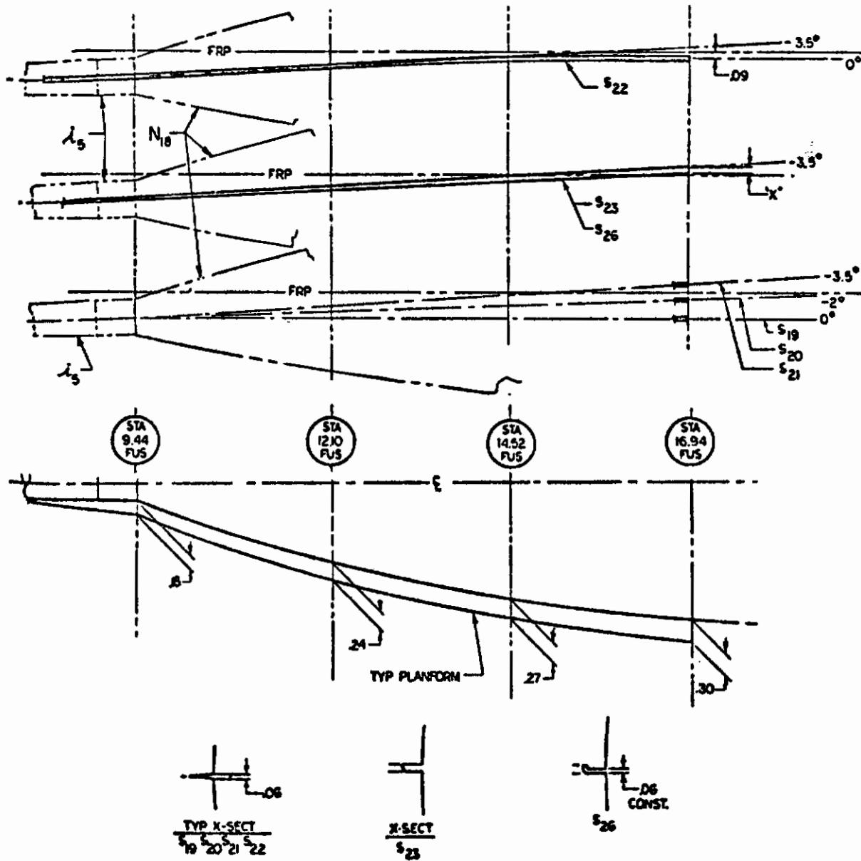
Figure 99. Nose Strake Angle Variation (S19, 20, 21, 22) and
