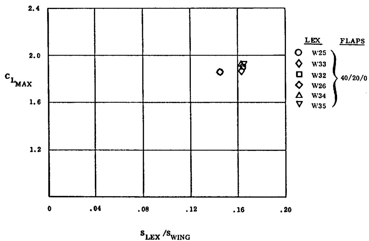
Figure 141. Effect of Lex Strake Length on  $C_{LMAX}$
