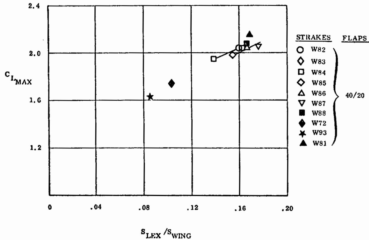
Figure 53. Effect of Small LEX Changes on C<sub>LMAX</sub>
