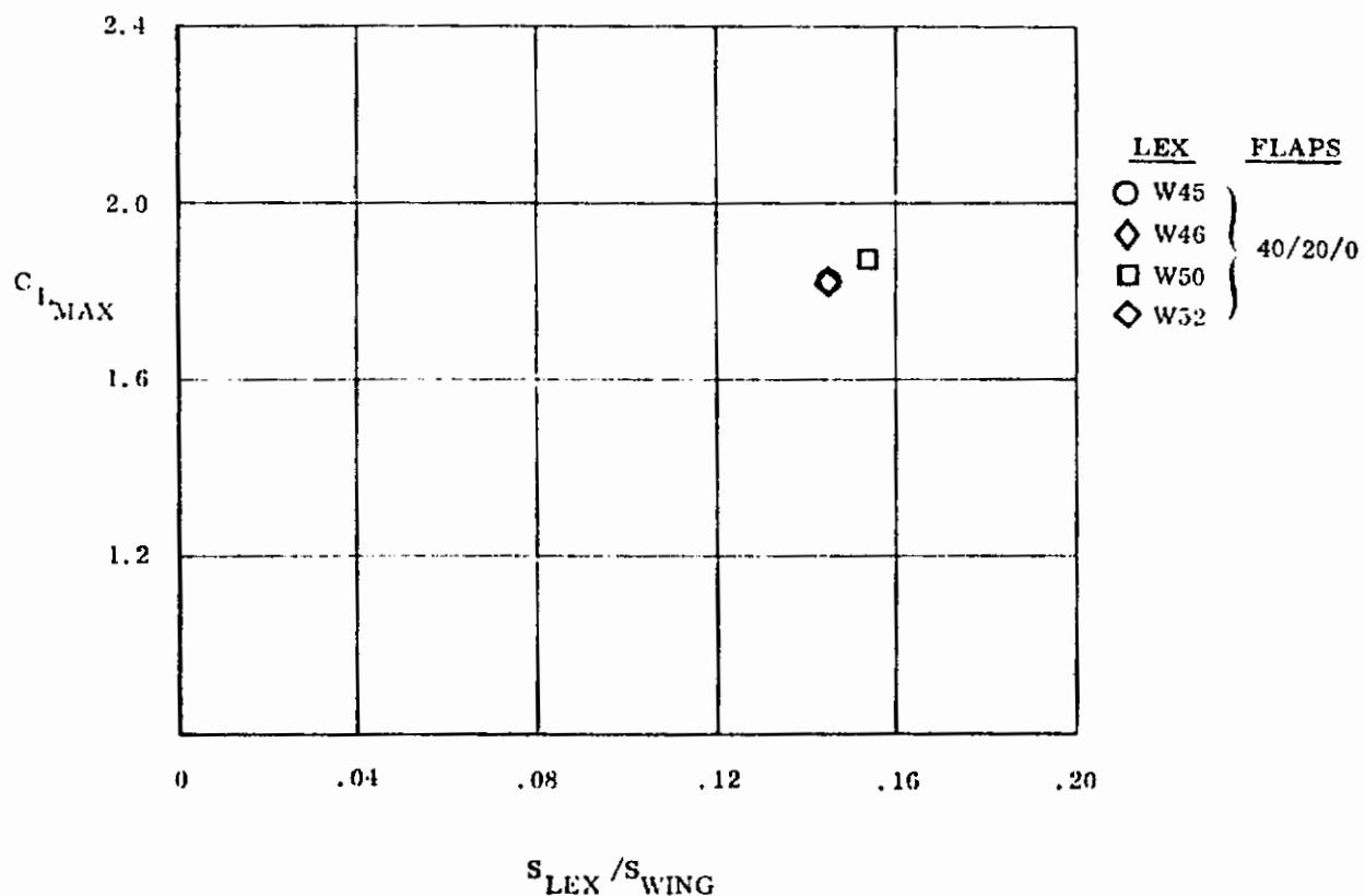
Figure 87. Effect of LEX Angle and LEX Strake on  $C_{LMAX}$
