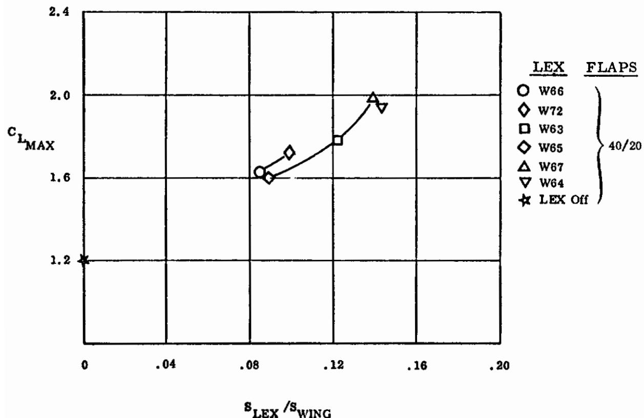
Figure 46. Effect of LEX Planform on  $C_{L_{MAX}}$
