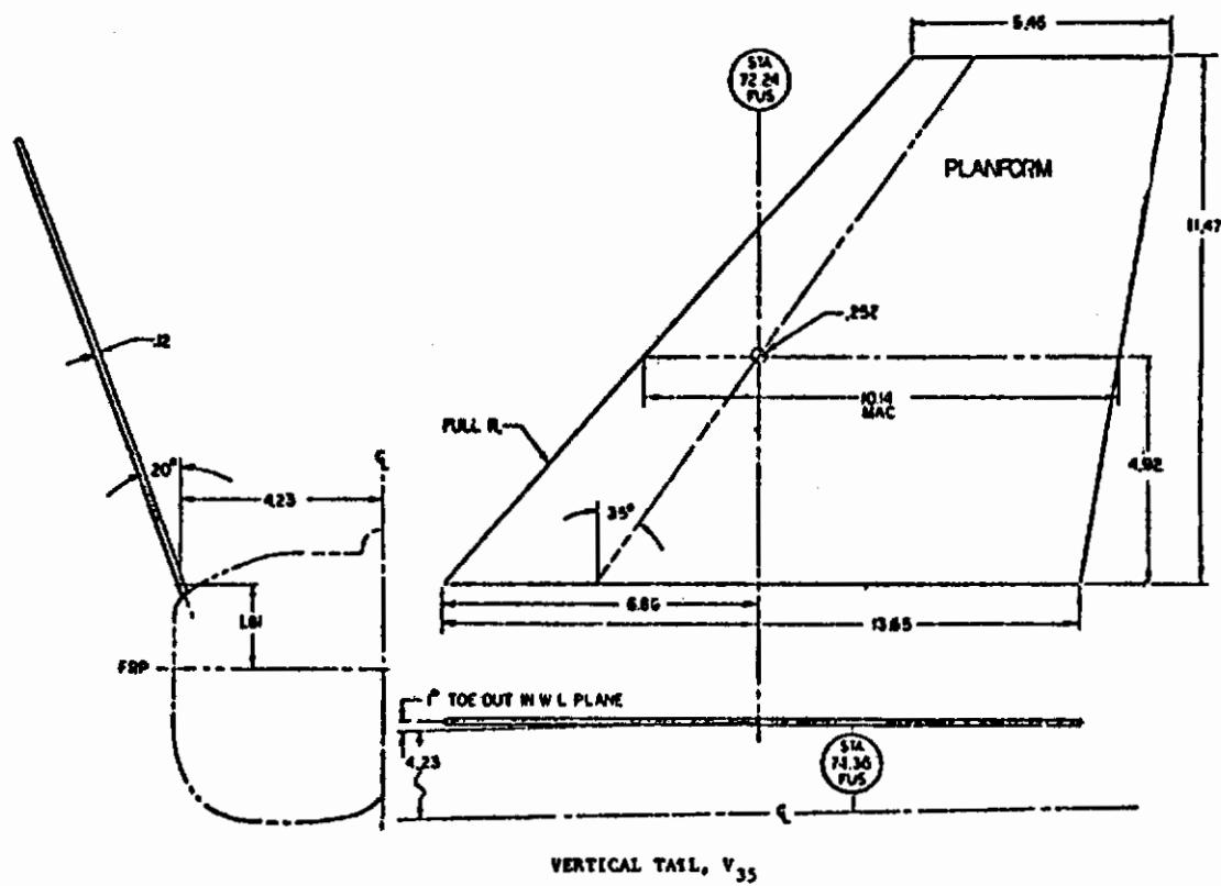
Figure 150. Vertical Tail, V35
