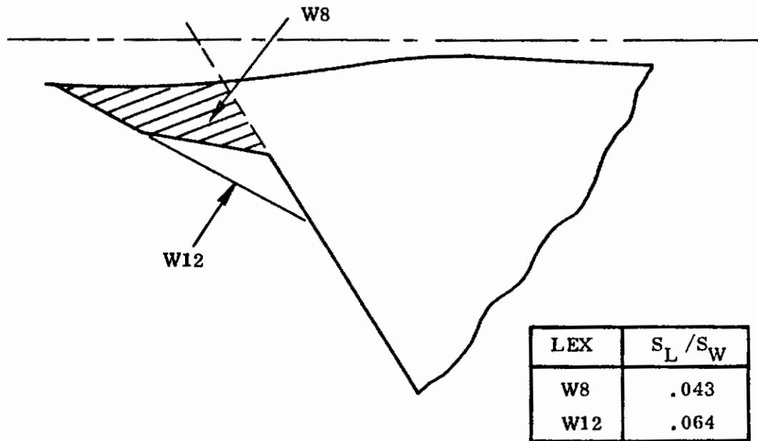
Figure 223. Lex Geometry W8, W12
