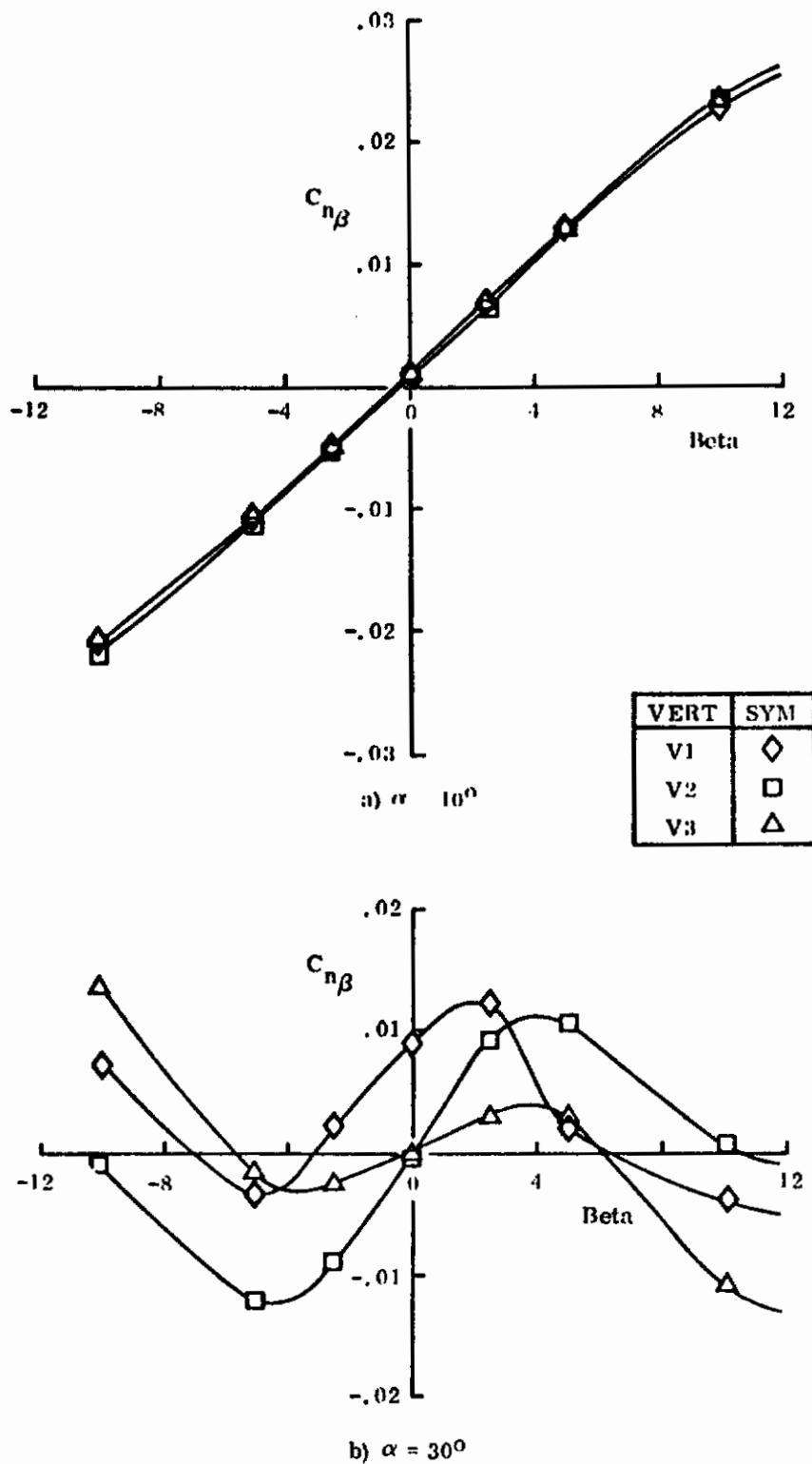
Figure 2. Effect of Angle of Attack on Sideslip Data for Various Vertical Tails
