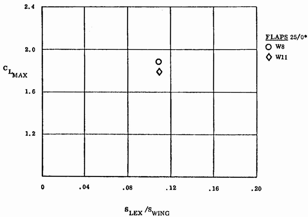
Figure 184. Effect of Lex Camber on  $C_{LMAX}$
