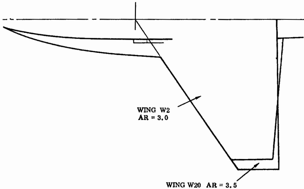
Figure 129. Variation in Wing Aspect Ratio (W2, W20)
