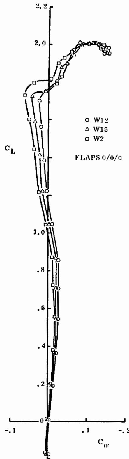
Figure 121. Effect of Lex Cross Section on  $C_L - C_m$  Curve
