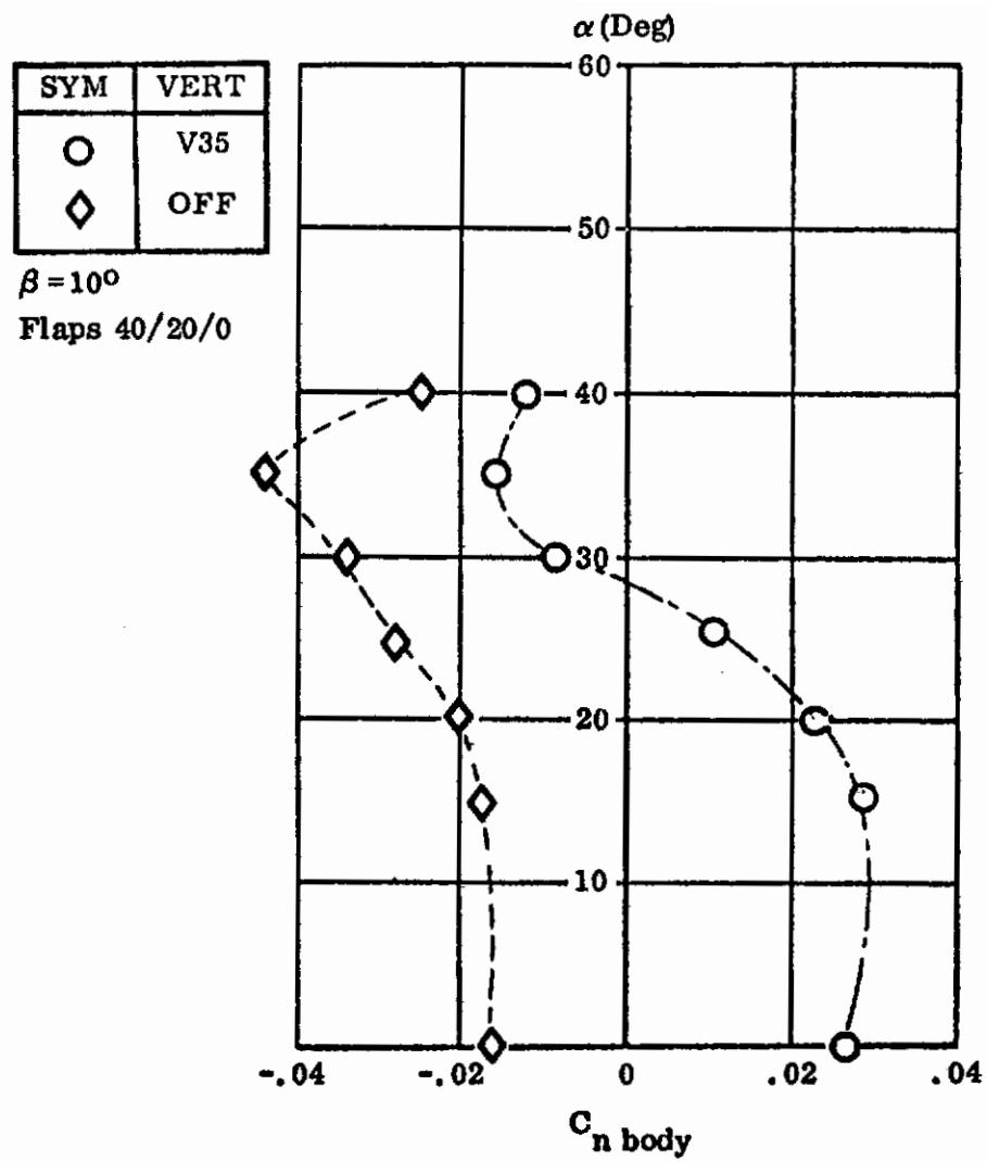
Figure 151. Effect of Vertical Tail
