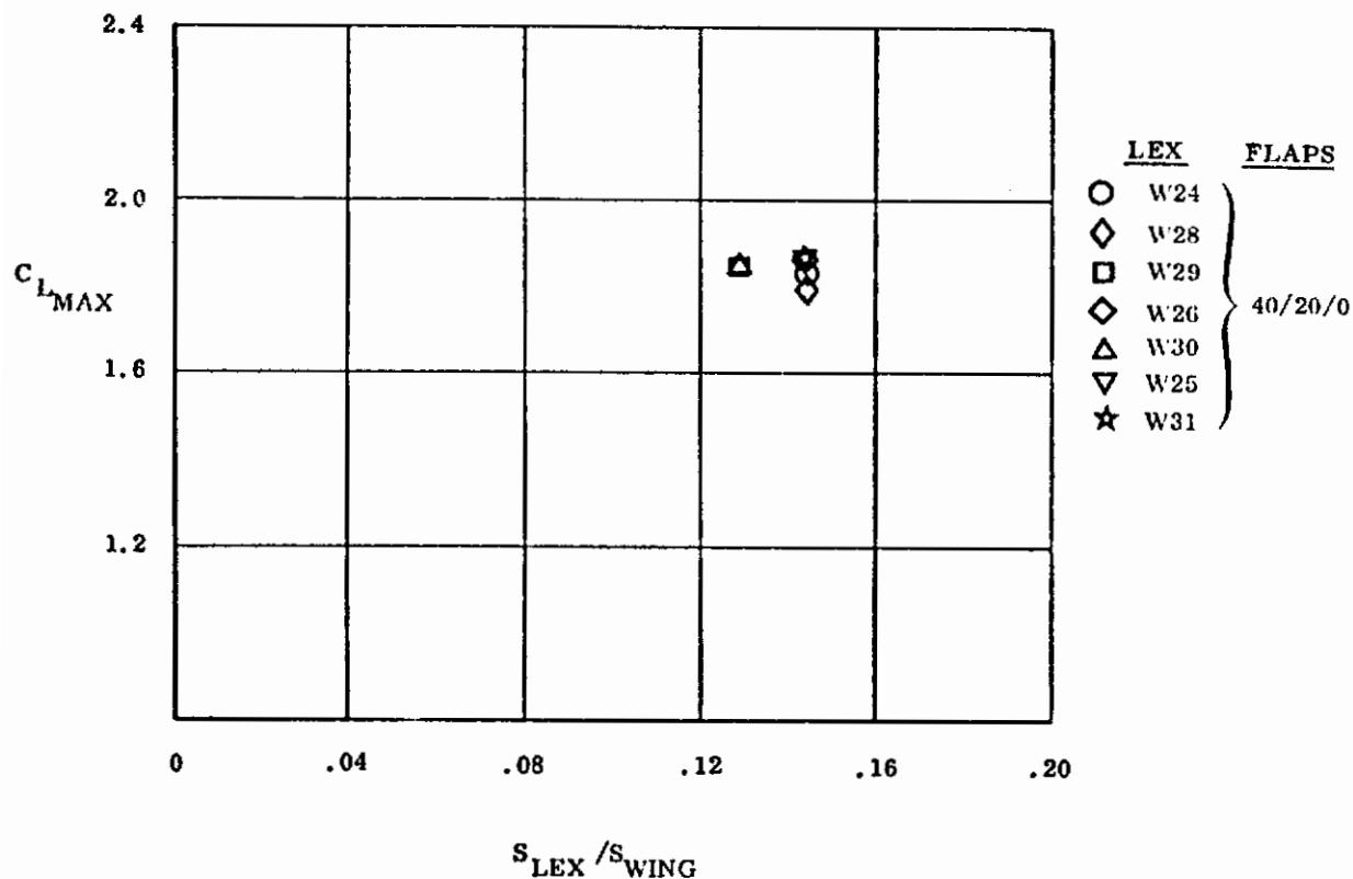
Figure 140. Effect of Lex Cross Section and Lex Strake on  $C_{L_{MAX}}$
