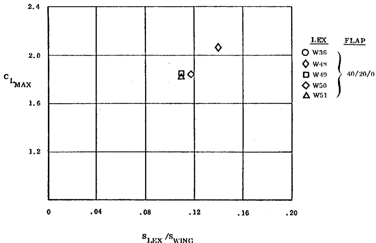
Figure 35. Effect of LEX Geometry on  $C_{L_{MAX}}$
