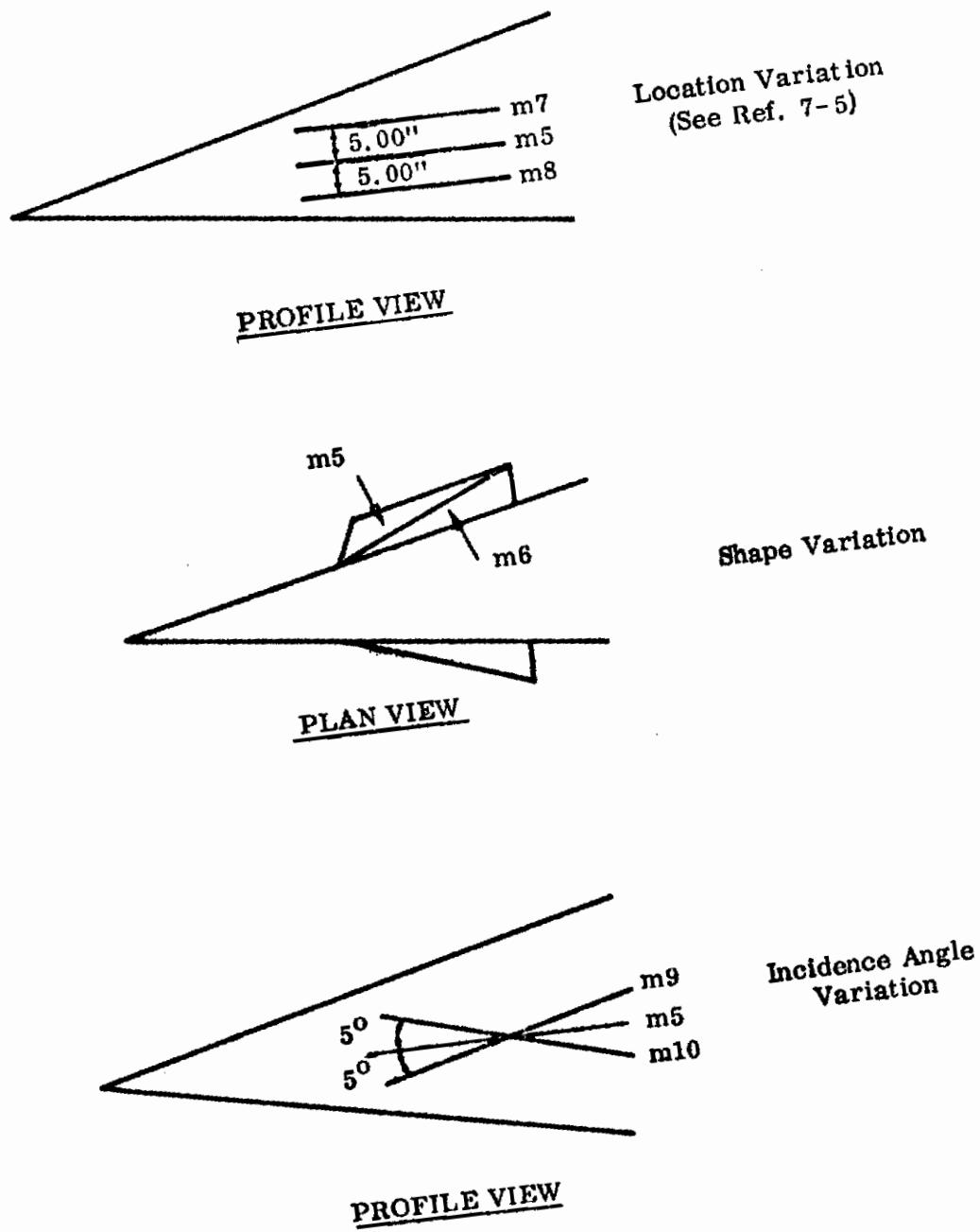
Figure 231. Fuselage Vortex Generators, m<sub>5</sub>-m<sub>10</sub>
