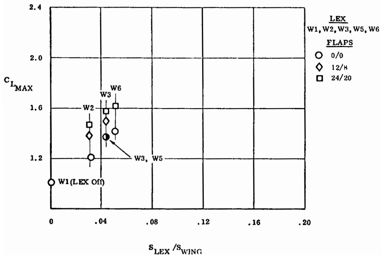
Figure 212. Effect of Lex Area, Lex Airfoil, and Flaps on  $C_{L_{MAX}}$
