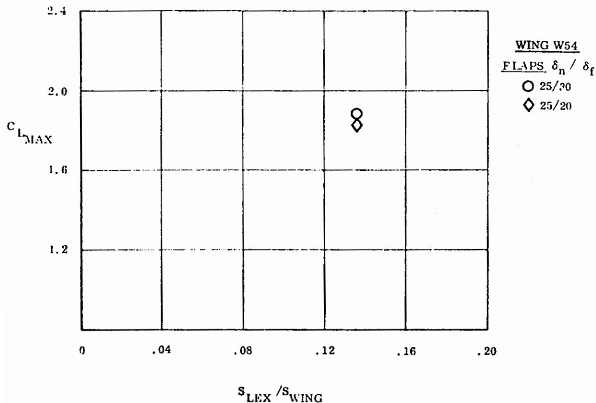
Figure 96. Effect of Flaps on  $C_{L_{MAX}}$
