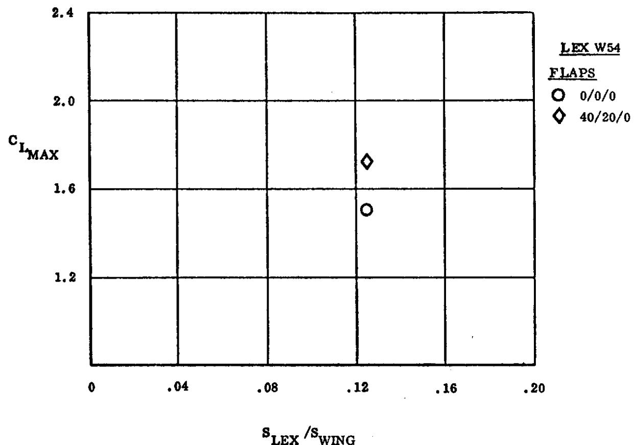
Figure 148. Effect of Flaps on  $C_{L_{MAX}}$
