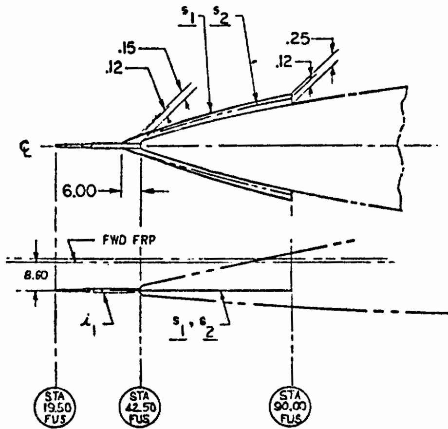
Figure 240. Nose Strakes  $S_1$ ,  $S_2$
