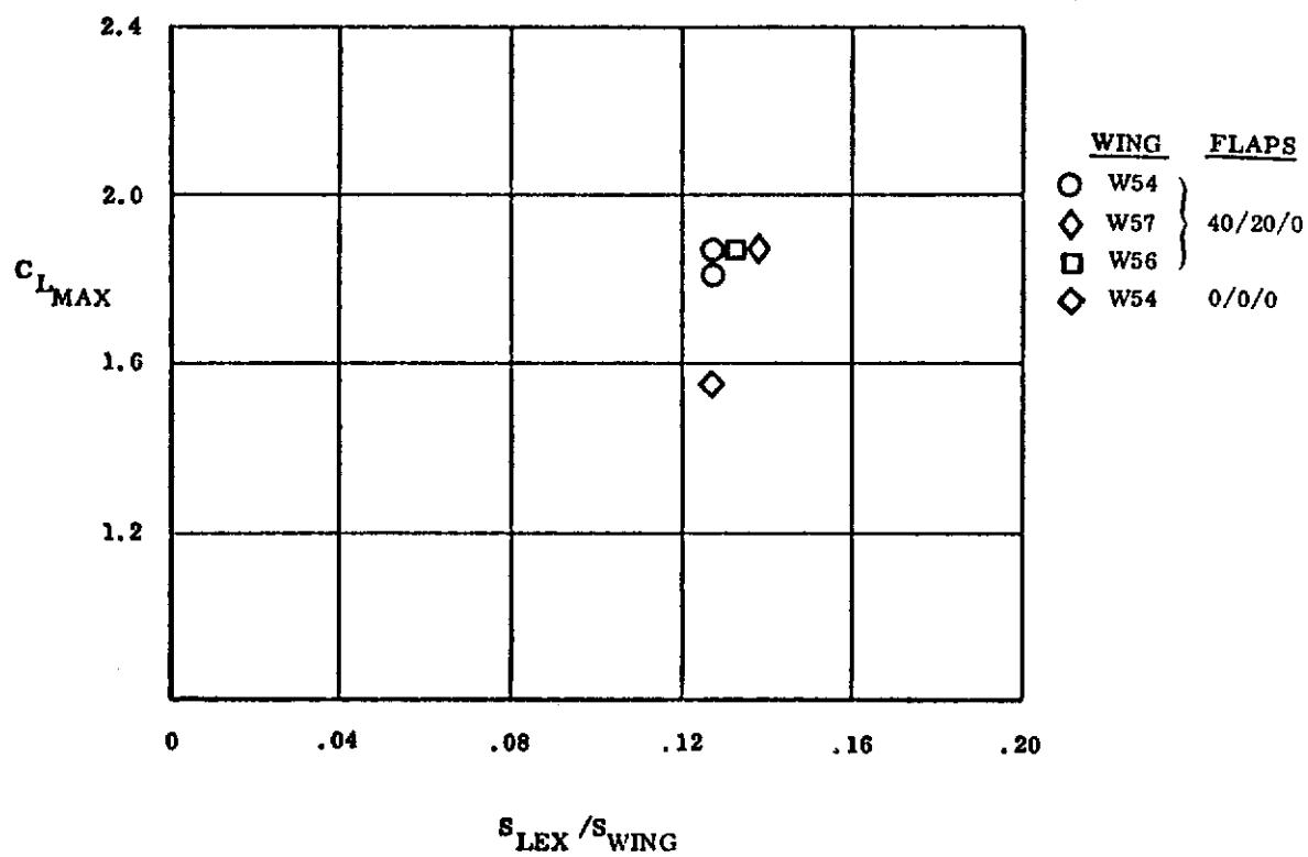
Figure 156. Effect of Strakes on  $C_{LMAX}$
