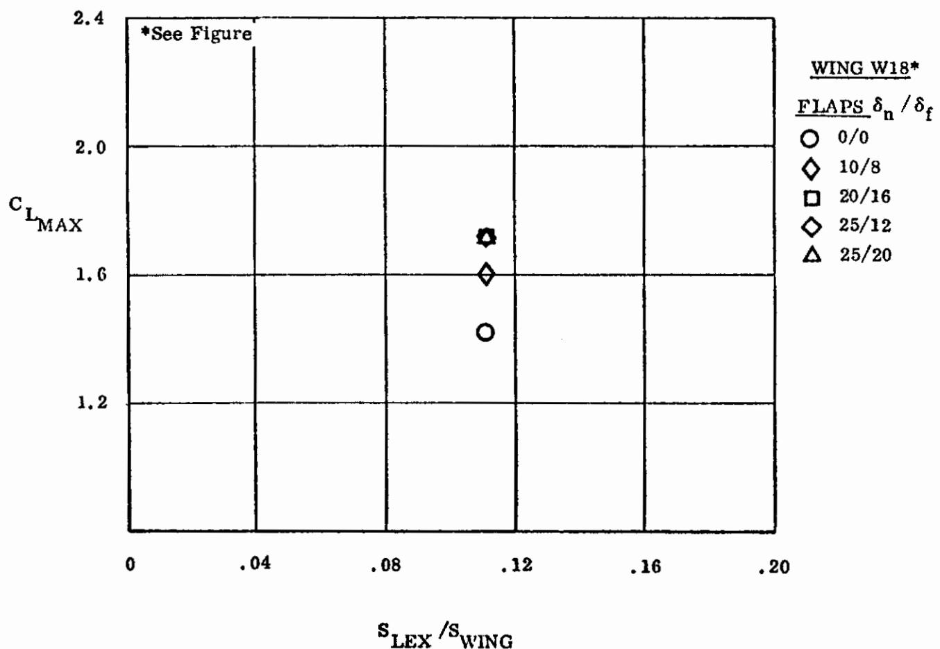
Figure 193. Effect of Flaps on Wing W18
