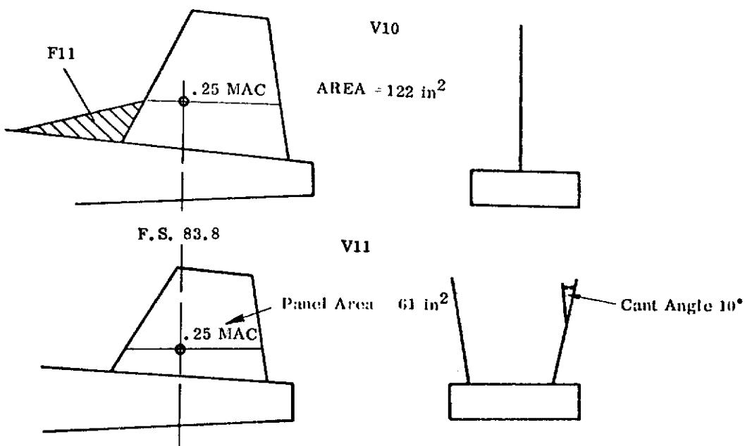
Figure 19. Vertical Tail and Dorsal Geometries
