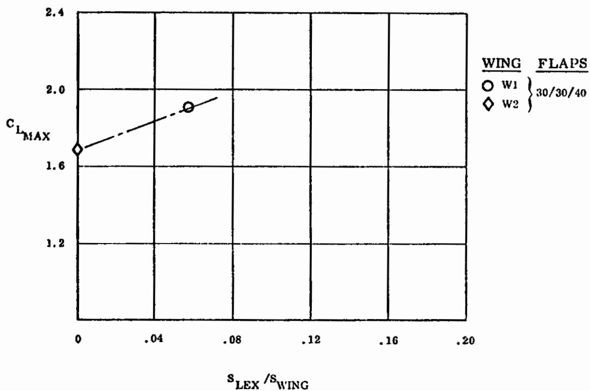
Figure 8. Effect of LEX with Full Flaps on  $C_{L_{MAX}}$
