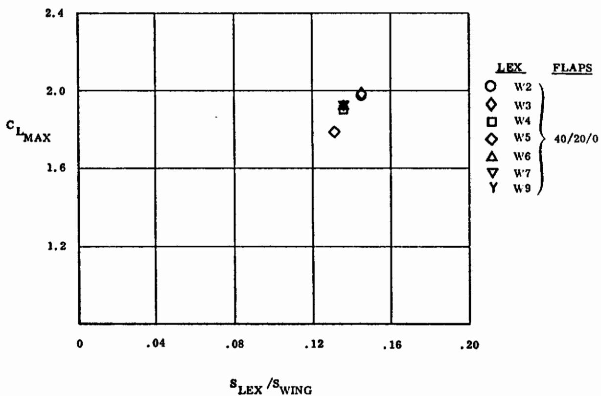
Figure 110. Effect of Lex Variation on  $C_{L_{MAX}}$
