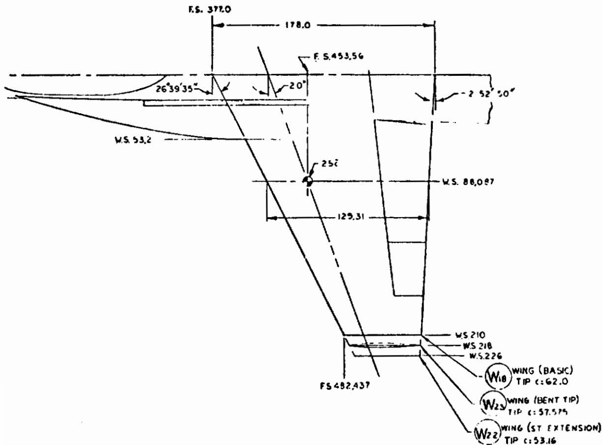
Figure 196. Wing Tips W18, W22, W23
