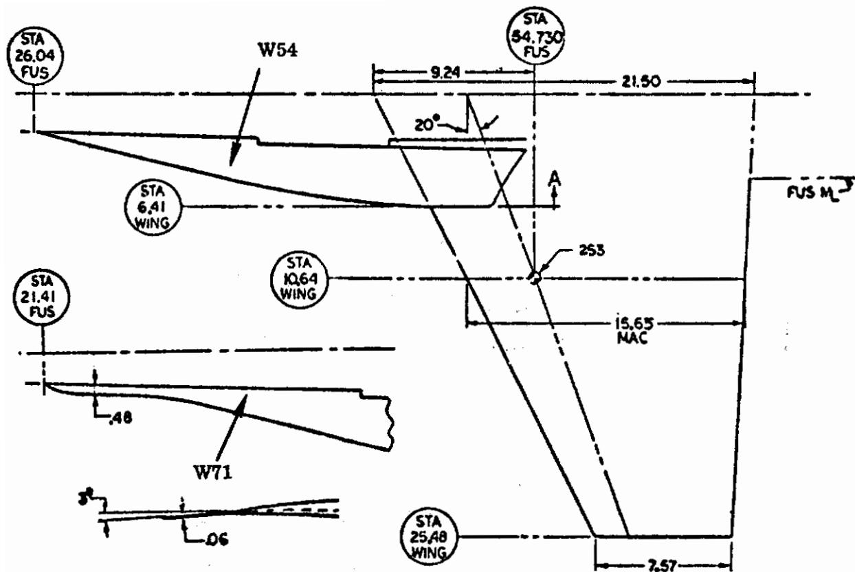
Figure 145. Lex Strakes, W54 & W71
