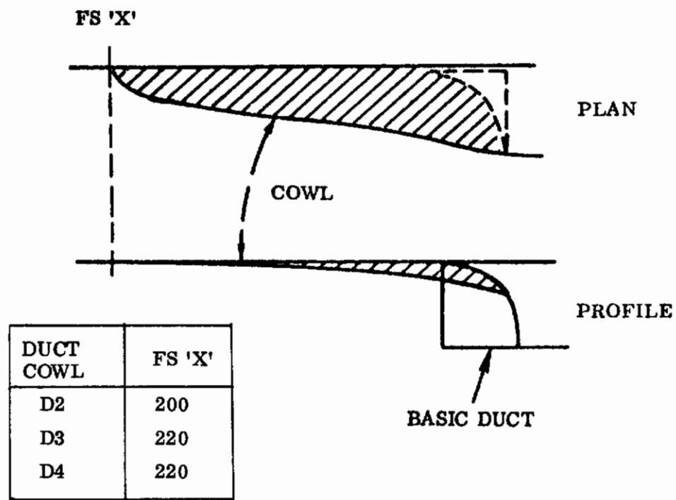
Figure 216. Duct Cowls (D2, D3, D4)
