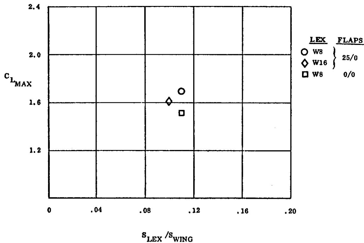
Figure 189. Effect of Planform, Effect of L. E. Flaps on  $C_{L_{MAX}}$
