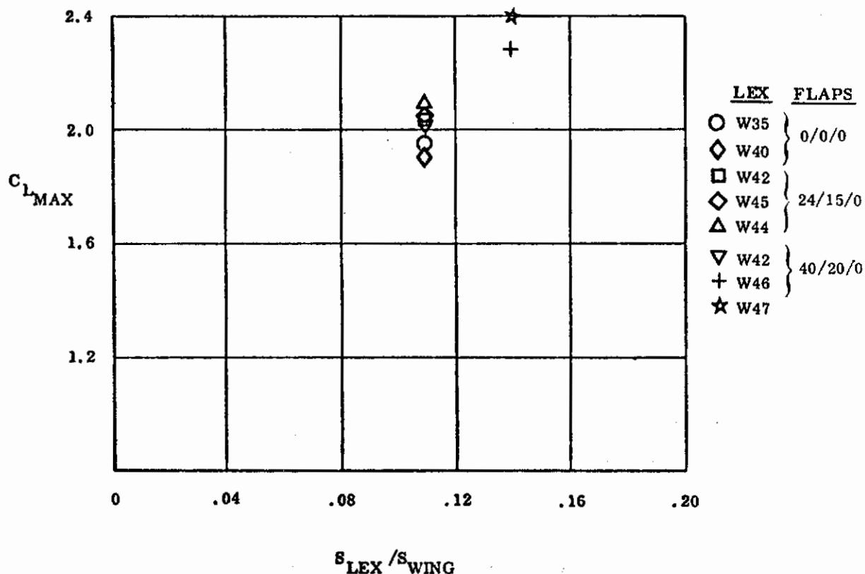
Figure 28. Effect of LEX Geometry Changes on  $C_{L_{MAX}}$
