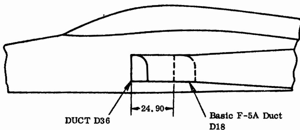
Figure 206. Duct Extensions D18, D36
