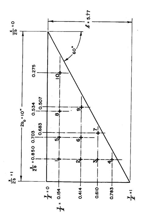
FIGURE D.8b LOCATION OF INFLUENCE-COEFFICIENT POINTS FOR DELTA-WING MODEL WITH ELEVON
