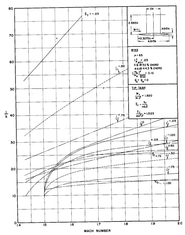
FIGURE 3.15 (Continued) THEORETICAL RESULTS FOR STRAIGHT WING WITH TIP TANK, FREE TO ROLL
