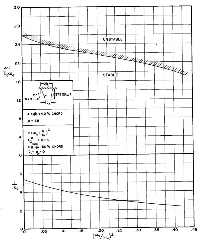
FIGURE 3.7 THEORETICAL RESULTS FOR BARE STRAIGHT-WING PLANFORM
