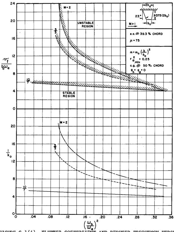
FIGURE C.1(i) FLUTTER COEFFICIENT AND REDUCED FREQUENCY VERSUS
