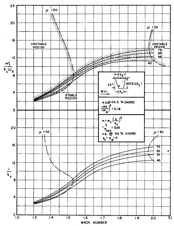
FIGURE 3.1(e) THEORETICAL RESULTS FOR BARE STRAIGHT-WING PLANFORM, e.a. AT 44.3% CHORD,  $\left(\frac{\omega_h}{\omega_\alpha}\right)^2 = 0.16$
