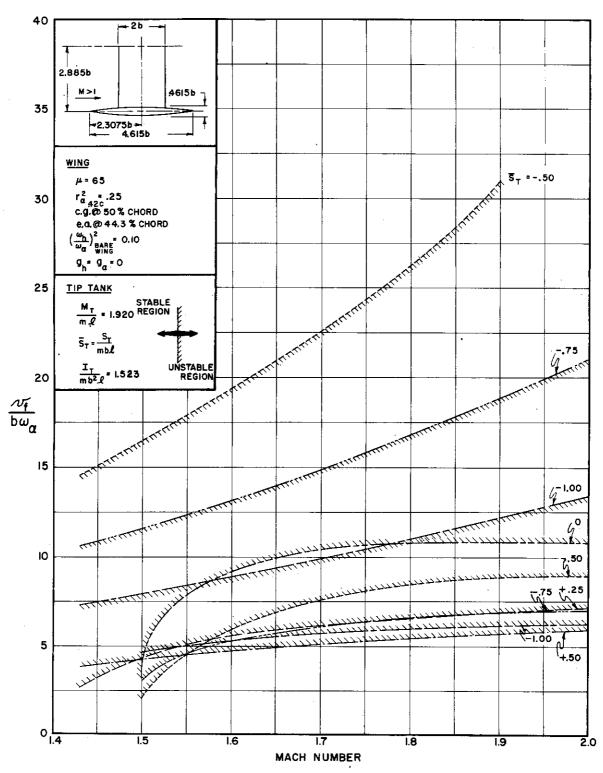
FIGURE 3.15 THEORETICAL RESULTS FOR STRAIGHT WING WITH TIP TANK, FREE TO ROLL
