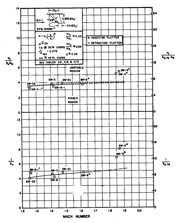
FIGURE 3.8 EXPERIMENTAL FLUTTER STABILITY BOUNDARY FOR BARE SWEPT-WING PLANFORM
