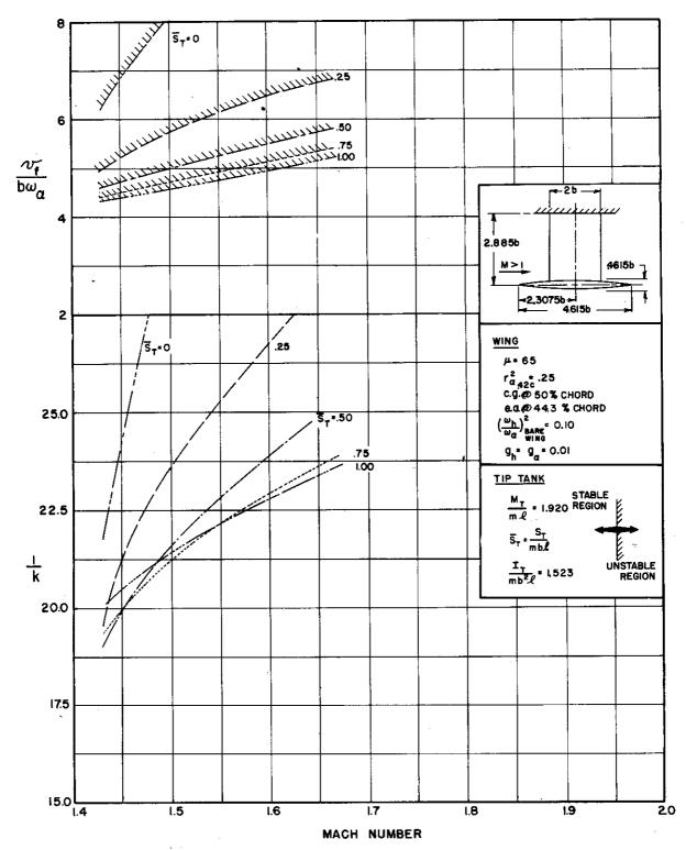
FIGURE 34.14 THEORETICAL RESULTS FOR CANTILEVER STRAIGHT WING WITH TIP TANK, STRUCTURAL DAMPING INCLUDED
