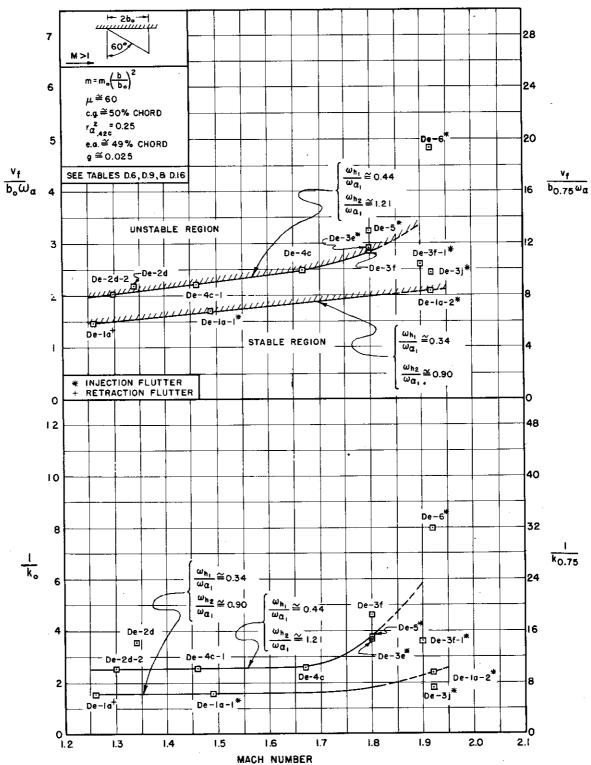
FIGURE 3.10 EXPERIMENTAL FLUTTER STABILITY BOUNDARIES FOR BARE DELTA-WING PLANFORM
