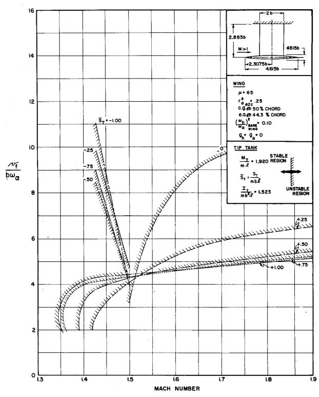
FIGURE 3.13 THEORETICAL RESULTS FOR STRAIGHT WING WITH TIP TANK, NO STRUCTURAL DAMPING
