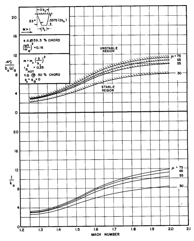
FIGURE 3.1(b) THEORETICAL RESULTS FOR BARE STRAIGHT-WING PLANFORM, e.a. AT 39.3% CHORD,  $\left(\frac{\omega_h}{\omega_a}\right)^2 = 0.16$
