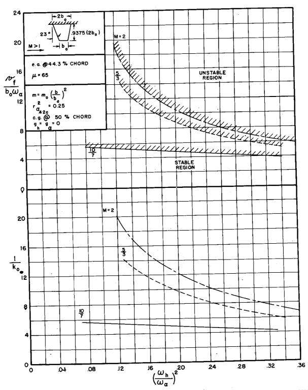
FIGURE C.1(h) FLUTTER COEFFICIENT AND REDUCED FREQUENCY VERSUS FREQUENCY RATIO FOR BARE STRAIGHT-WING PLANFORM, e.a. AT 44.3% CHORD,  $\mu = 65$
