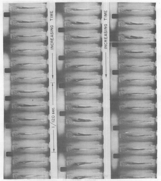
(a) Straight Wing with Free Aileron, Cantilever (Model ST-le)
