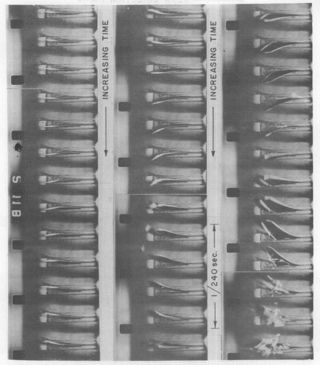
(e) Bare Swept Wing, Cantilever (Model SW-5, Injection Flutter)
