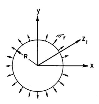
FIGURE B.2 RADIAL FLOW DUE TO A SOURCE
