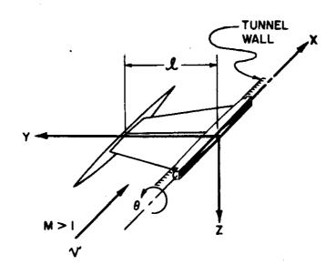
FIGURE A.2 AXIS SYSTEM FOR WING WITH TIP TANK
