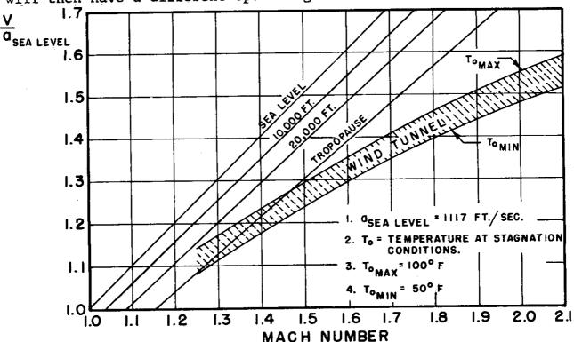
FIGURE 3.2 VELOCITY VERSUS MACH NUMBER FOR EXTREME RANGES OF
