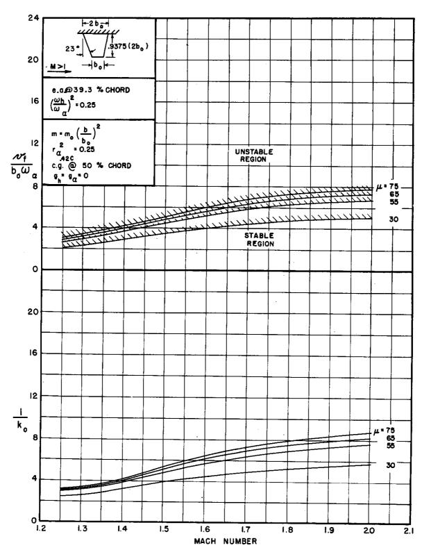
FIGURE 3.1(c) THEORETICAL RESULTS FOR BARE STRATCHT-WING PLANFORM, e.a. AT 39.3% CHORD  $\left(\frac{\omega_h}{\omega_a}\right)^2 = 0.25$
