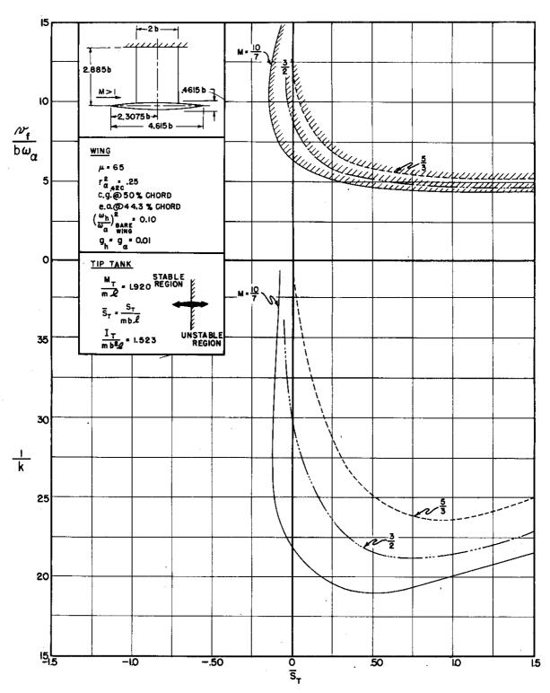
FIGURE C.5 FLUTTER COEFFICIENT AND REDUCED FREQUENCY VERSUS TIP-TANK STATIC-UNBALANCE PARAMETER FOR STRAIGHT-WING PLANFORM, STRUCTURAL DAMPING INCLUDED
