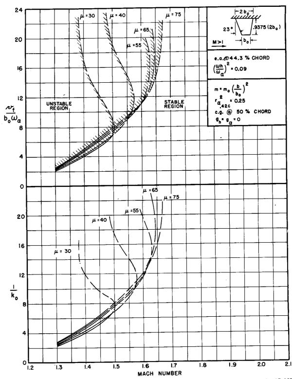
FIGURE 3.1(d) THEORETICAL RESULTS FOR BARE STRAIGHT-WING PLAN-FORM, e.a. AT 44.3% CHORD,  $\left(\frac{\omega_h}{\omega_a}\right)^2$  = 0.09
