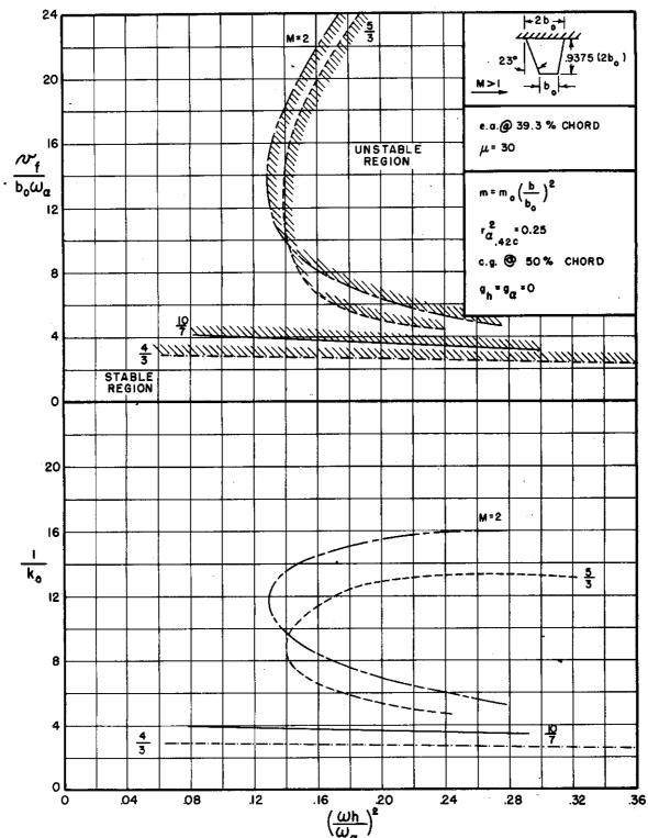
FIGURE C.1(a) FLUTTER COEFFICIENT AND REDUCED FREQUENCY VERSUS FREQUENCY RATIO FOR BARE STRAIGHT-WING PLANFORM,
