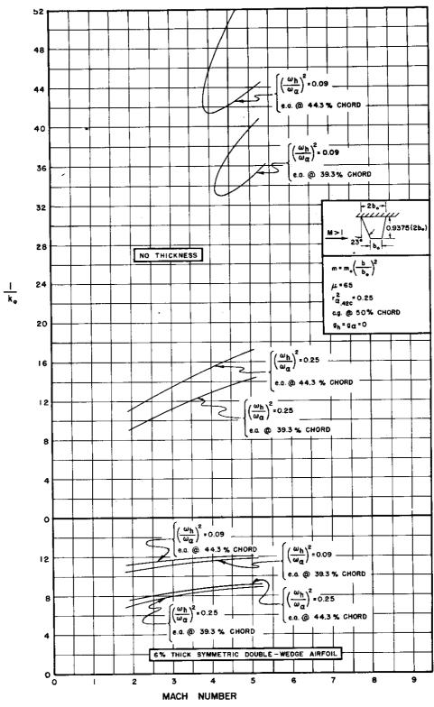
FIGURE 3.6 (Continued) THEORETICAL RESULTS FOR BARE STRAIGHT-WING PLANFORM BASED ON PISTON THEORY
