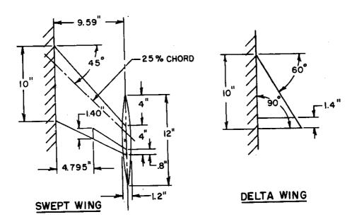
AIRFOIL SECTION SYMMETRICAL DOUBLE WEDGE ON ALL MODELS, 6% THICK EXCEPT AS NOTED FOR DELTA WINGS IN TABLE D.6
