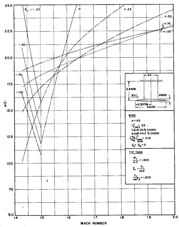
FIGURE 3.13 (Continued) THEORETICAL RESULTS FOR STRAIGHT WING WITH TIP TANK, NO STRUCTURAL DAMPING
