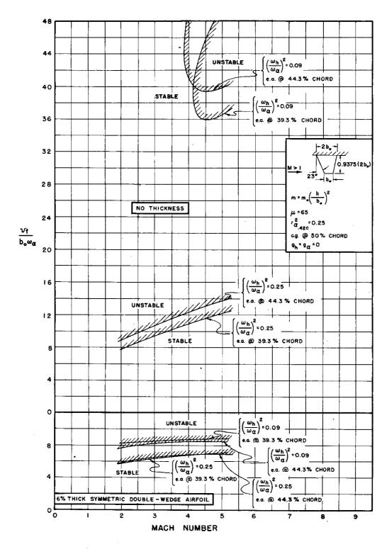
FIGURE 3.6 THEORETICAL RESULTS FOR BARE STRAIGHT-WING PLANFORM
