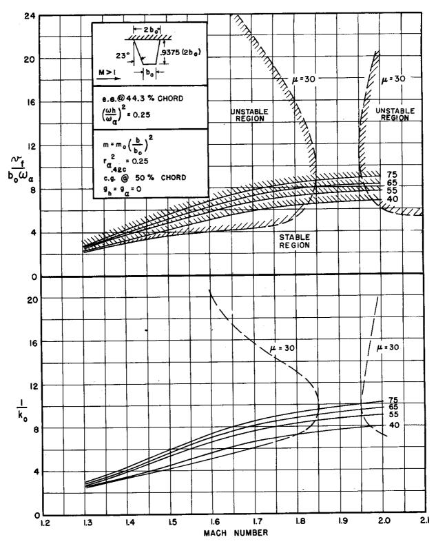
FIGURE 3.1(f) THEORETICAL RESULTS FOR BARE STRAIGHT-WING PLAN-FORM, e.a. AT 44.3% CHORD,  $\left(\frac{\omega_h}{\omega_A}\right)^2 = 0.25$
