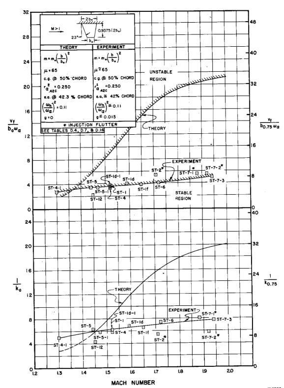
FIGURE 3.4 THEORETICAL AND EXPERIMENTAL FLUTTER STABILITY
