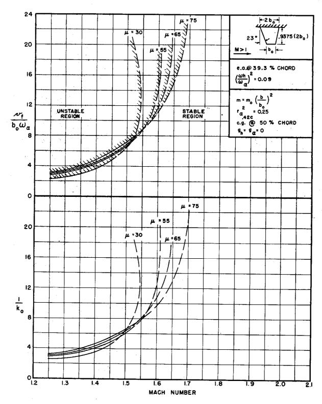
FIGURE 3.1(a) THEORETICAL RESULTS FOR BARE STRAIGHT-WING PLAN-FORM, e.a. AT 39.3% CHORD,  $\left(\frac{\omega_h}{\omega_d}\right)^2 = 0.09$
