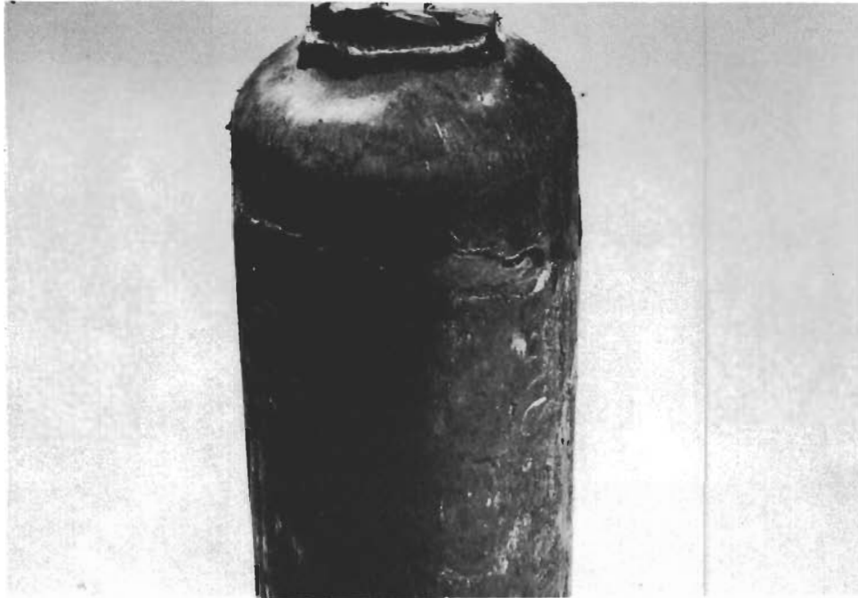
FIGURE 54 Shape of billet during glass extrusion when billet nose is machined as type A, Fig. 8.
