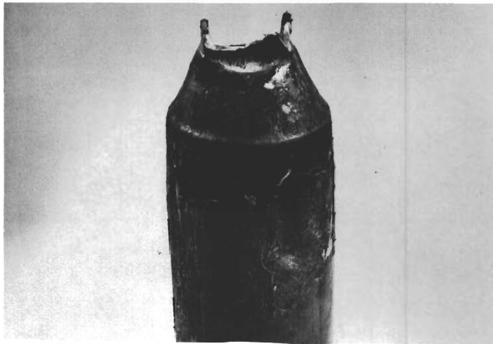
FIGURE 55 Shape of billet during glass extrusion when billet nose is machined as type B, Fig. 8.
