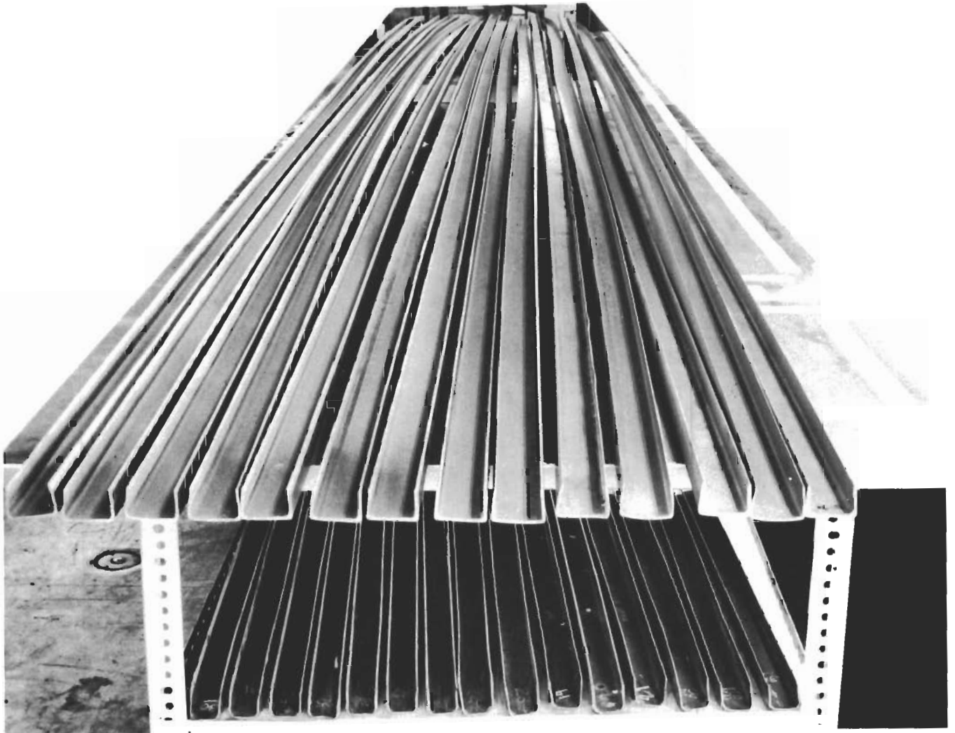
FIGURE 95 Photograph showing the Beryllium U-channels produced by the clad technique in Phases I, II, and III of this program for the development of extruded Beryllium shapes.
