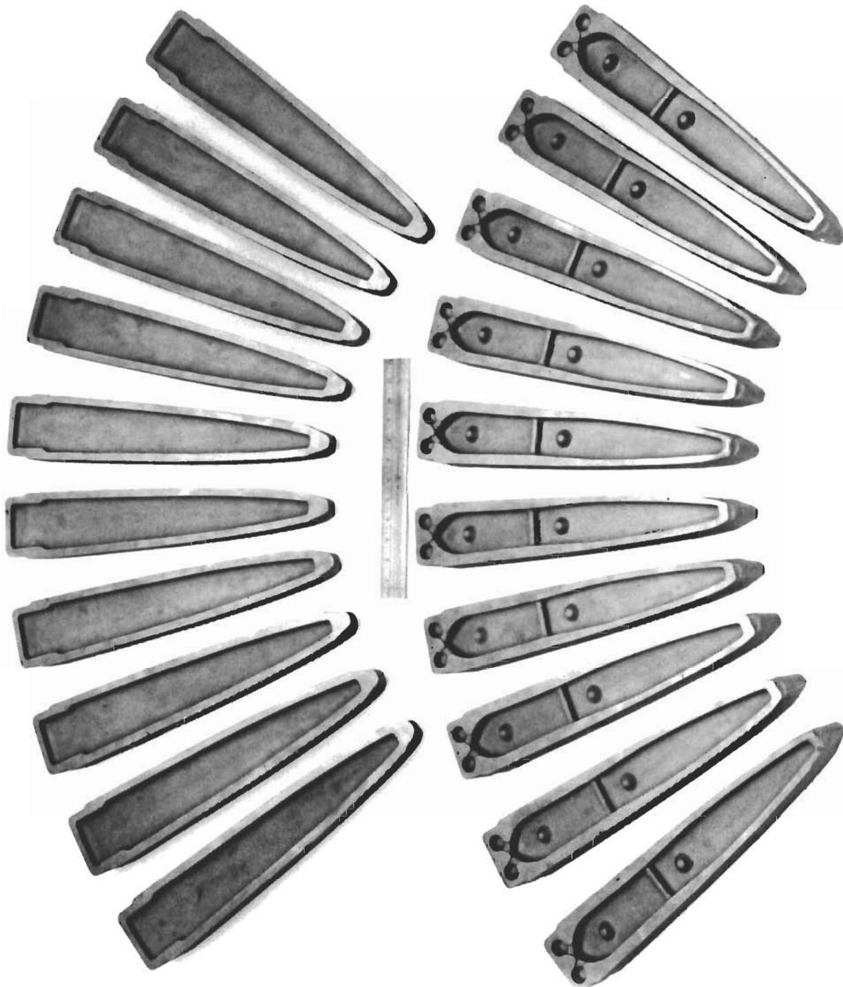
Figure 40. Ten High Strength Steel (D6ac) Fin Rib Forgings Produced with 6000 Ton Hydraulic Press for TRW Evaluation. Upper and Lower Views Represent Upper and Lower Die Impressions, Respectively, for the Finish Forging Operation. Shown after Trimming and Abrasive Blasting.
