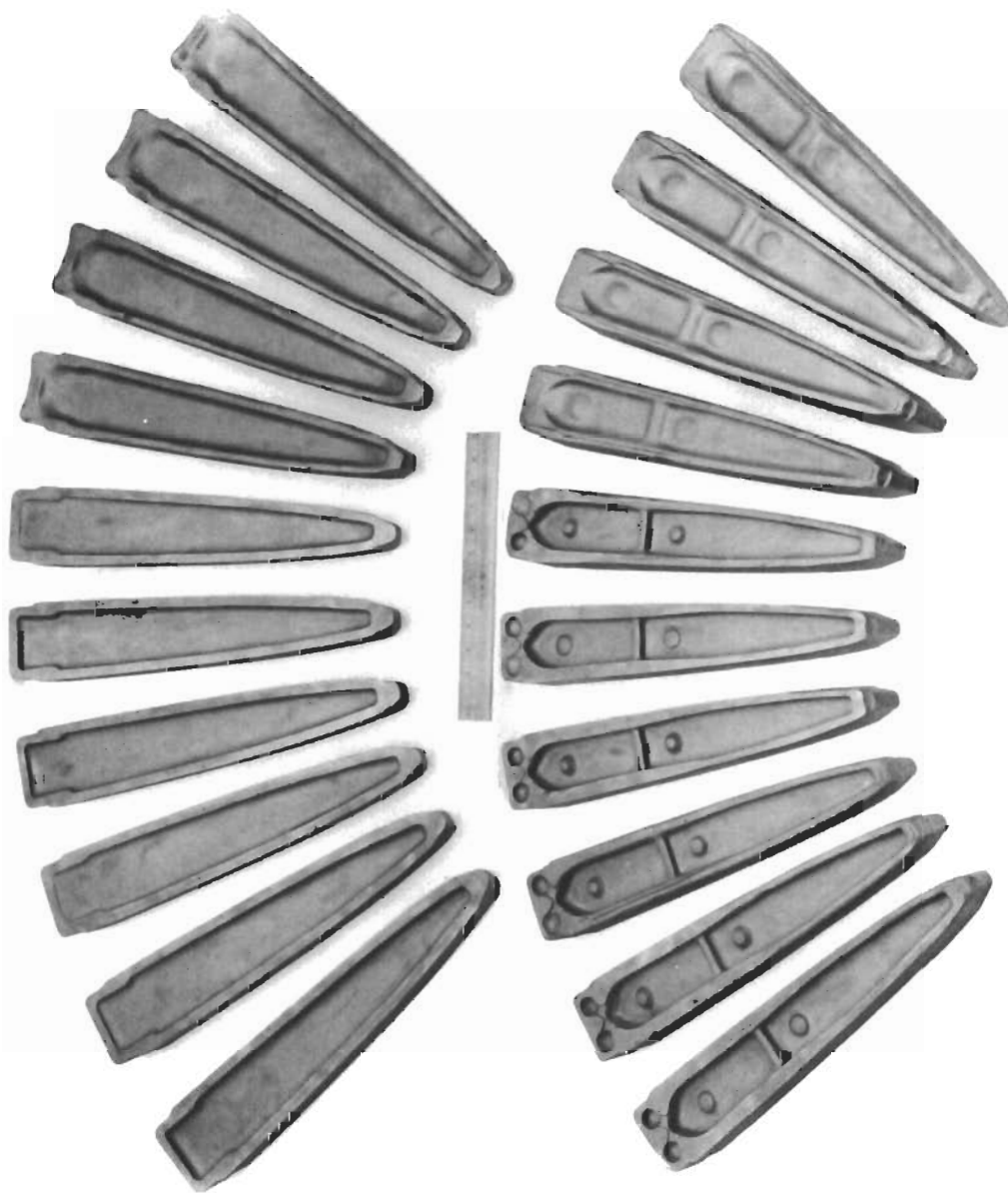
Figure 45. Ten Nickel-Base Alloy (Inconel 718) Fin Rib Forgings Produced with 6000 Ton Hydraulic Press for TRW Evaluation. Upper and Lower Views Represent Upper and Lower Die Impressions, Respectively, for the Finish Forging Operation. Shown after Trimming and Abrasive Blasting.
