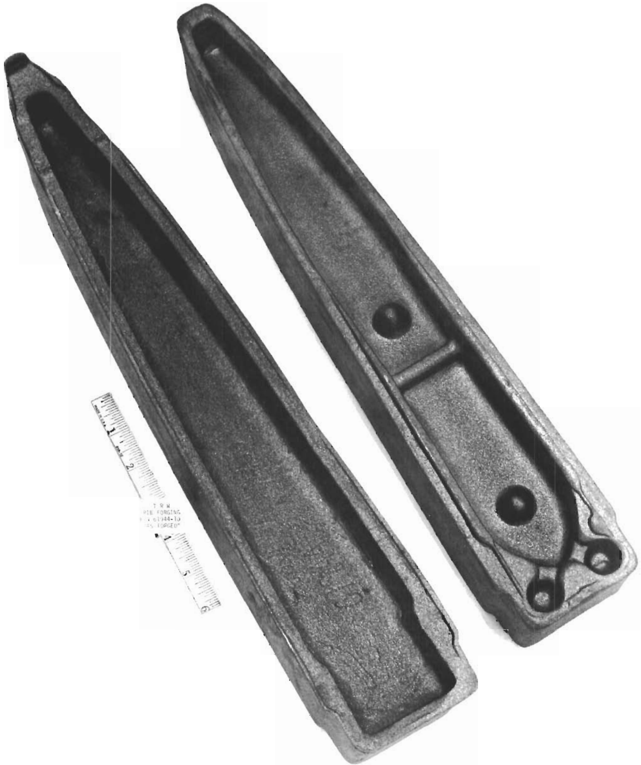
Figure 36. Upper (left) and Lower (right) Die Views of D6ac Forging Produced with 6000 Ton Hydraulic Press. As-Forged and Abrasive Blasted Prior to "Trimming" of Excess Rib Height.
