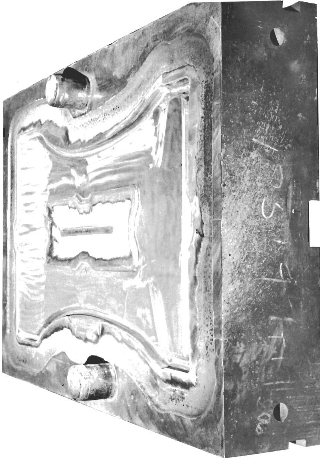
Figure 128. Upper Die for the Finish Bulkhead Forging Operation with the 50,000 Ton Hydraulic Press. Impression Polished and Photograph Taken after Completion of All Program Forging Efforts with the Press.
