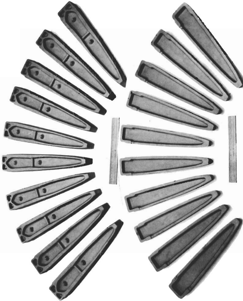
Figure 60. Ten High Strength Steel (D6ac) Fin Rib Forgings Produced with 4000 Ton Mechanical Press for TRW Evaluation. Upper and Lower Views Represent Upper and Lower Die Impressions, Respectively, for the Finish Forging Operation. Shown after Trimming and Abrasive Blasting.
