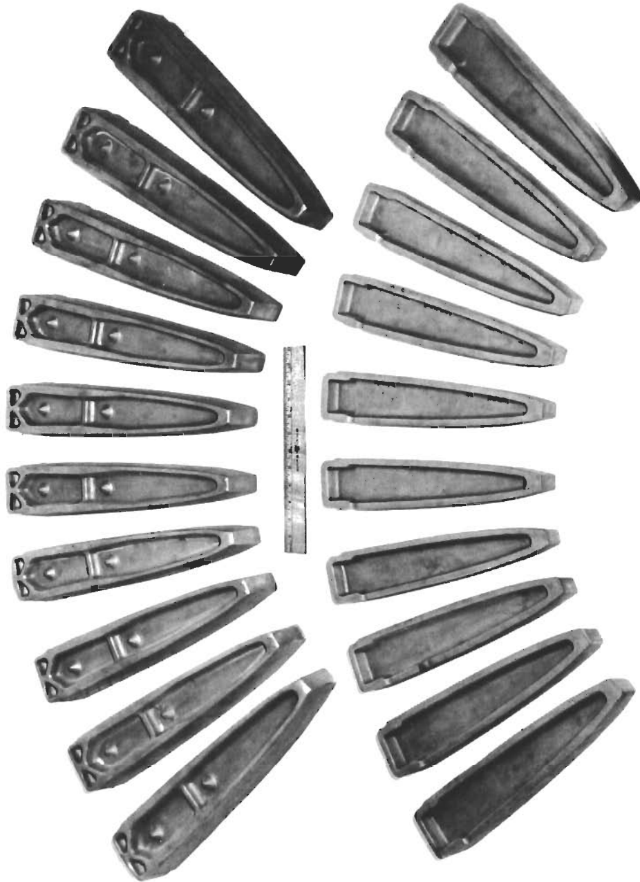
Figure 23. Ten Titanium Alloy (Ti 6Al-4V) Fin Rib Forgings Produced with 12,000 Pound Steam Drop Hammer for TRW Evaluation. Upper and Lower Views Represent Upper and Lower Die Impressions, Respectively, for the Finish Forging Operation. Shown after Trimming and Abrasive Blasting.
