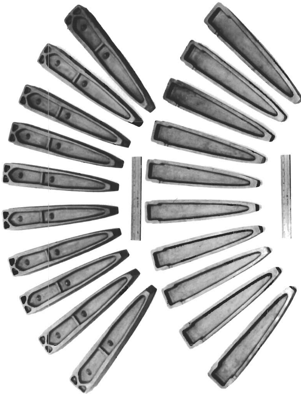
Figure 62. Ten Titanium Alloy (Ti 6Al-4V) Fin Rib Forgings Produced with 4000 Ton Mechanical Press for TRW Evaluation. Upper and Lower Views Represent Upper and Lower Die Impressions, Respectively, for the Finish Forging Operation. Shown after Trimming and Abrasive Blasting.
