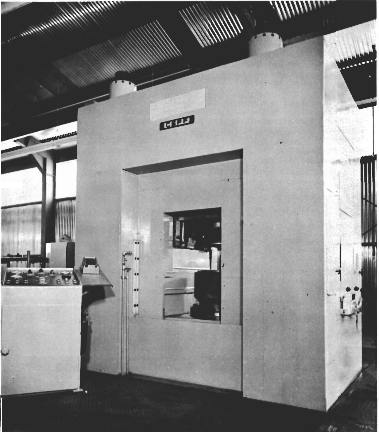
Figure 68. Model HE-55, CEFF-Type HERF Machine Rated at 400,000 Foot Pounds per Blow. Similar to Machine Employed at Precision Metal Products Div., Macrodyne-Chatillon Corp. to Produce Fin Rib Forgings. Dies Shown Installed are not Pertinent to Program.
