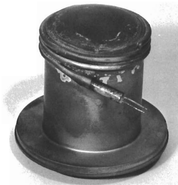
Figure 103. Input heater brazed to hot cylinder of unit 447525-100 (HAC photo 4R02722)
