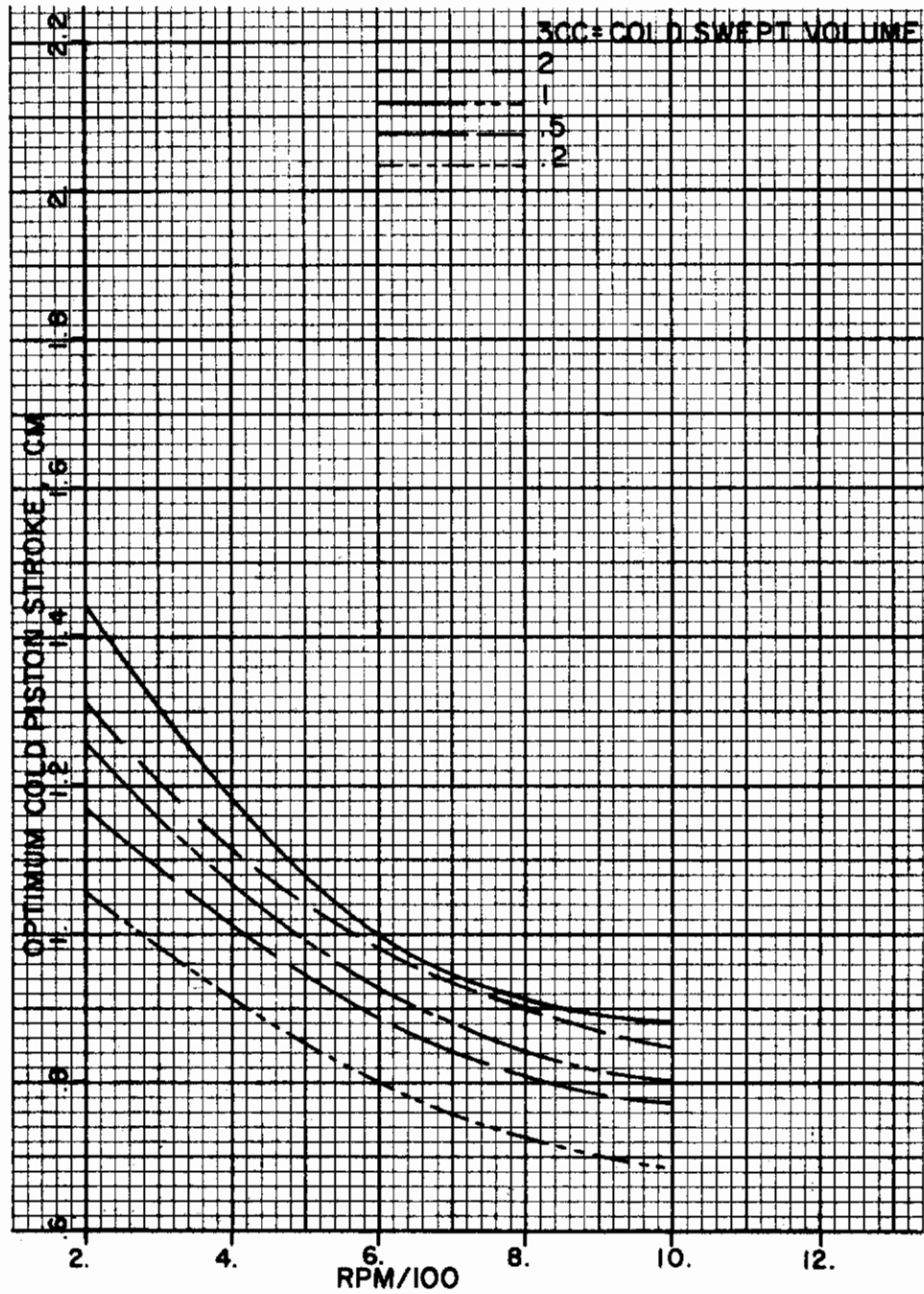
Figure 49. Optimum piston stroke as a function of rpm for five cold volumes.
