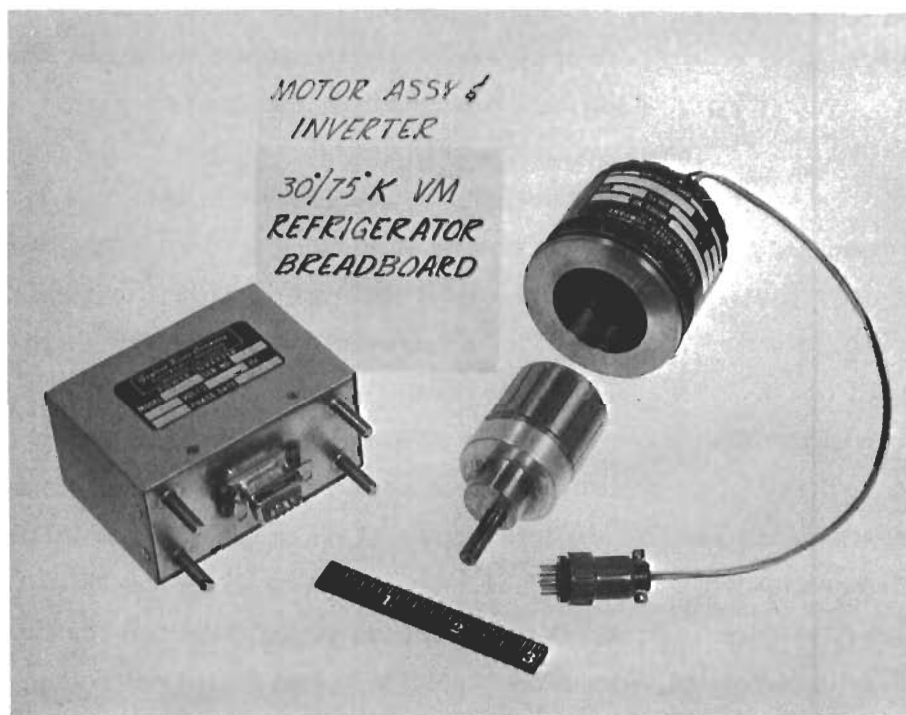
Figure 87. Drive motor and inverter of unit 447550-100 (HAC photo 4R02921)
