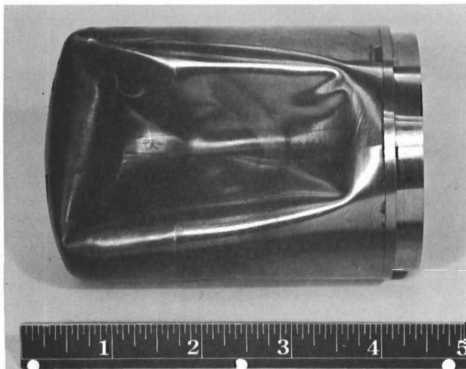
Figure 83. Side view of failed hot displacer of unit 447550-100 (HAC photo 4R02723)
