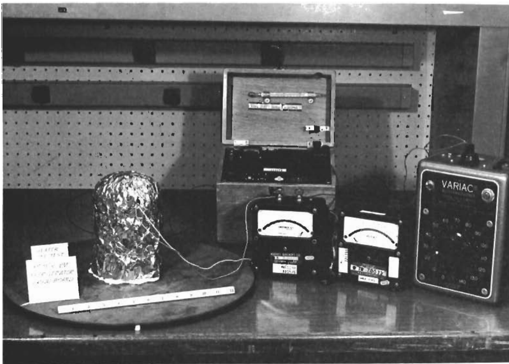
Figure 86. Heater life test setup for unit 447550-100 (HAC Photo 5R02717)
