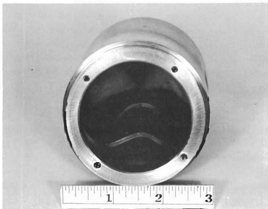
Figure 84. End view of failed hot displacer of unit 447550-100 (HAC photo 4R02724)
