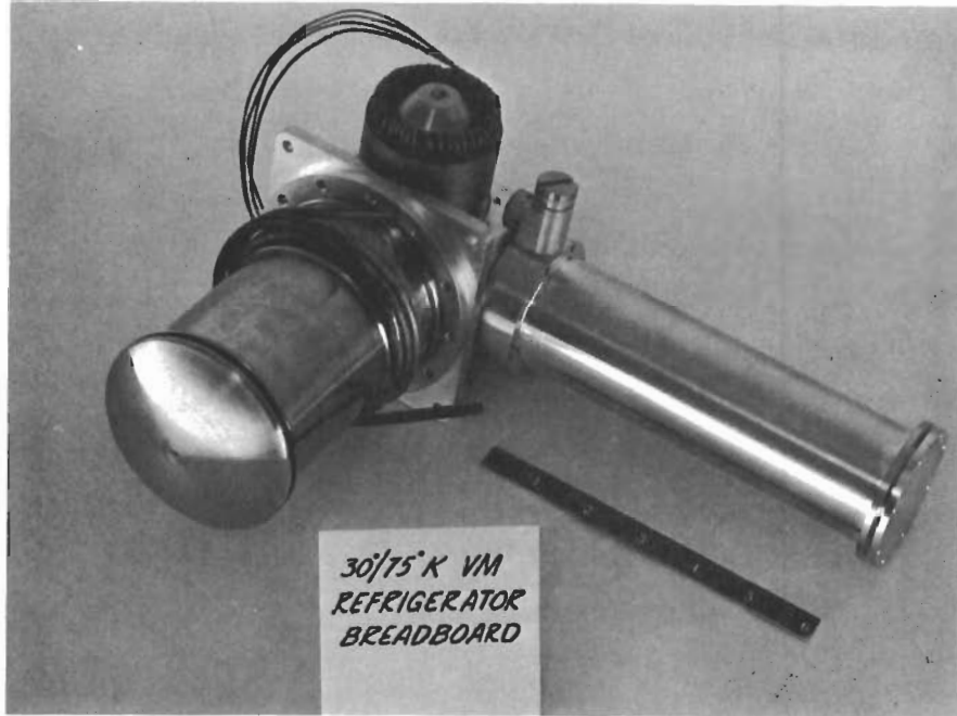
Figure 2. 30°/75°K Vuilleumier cryogenic refrigerator breadboard, assembly (HAC photo 5R00588)
