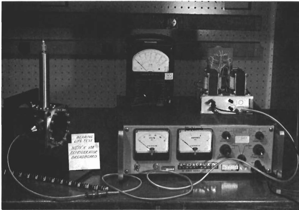
Figure 80. Setup for bearing life test of unit 447550-100 (HAC photo 5R02719)
