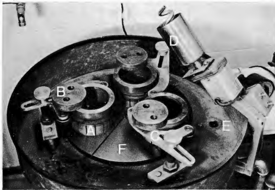
Figure 1. Lap for producing finely lapped surfaces for microscopic examination and air void analysis. A. Slotted specimen holder, rotating. B. Cover plate to set on top of specimen. C. Guide yoke that retains specimen holder. D. Grit-slurry cup mounted on its motor and containing a spiral agitator/pump. E. Drain. F. Grooved lap.
