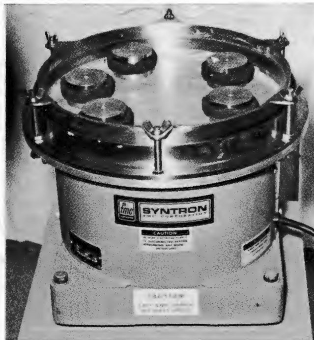
Figure 10. Syntron vibratory polisher and weights complete with sponge rubber bumpers. The thin sections are attached to the bottom of the weights.
