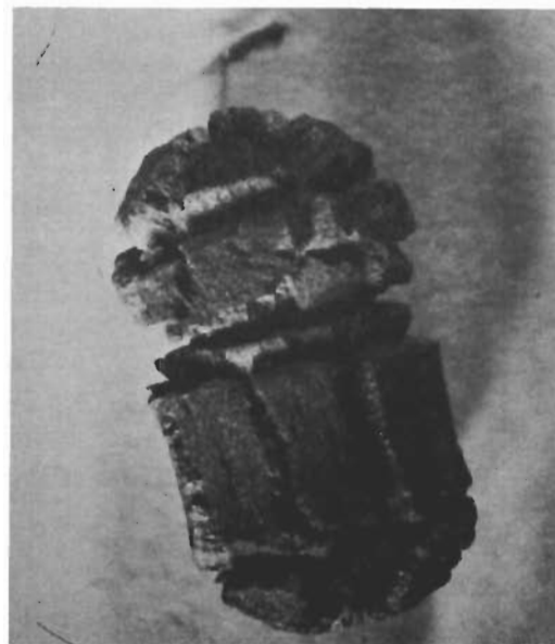
B. W oxidized at 1150°C 5 torr - 2 hr. 10X
