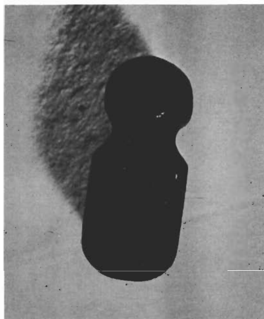
B. W oxidized at 1150°C 5 torr - 2 hr. 10X
