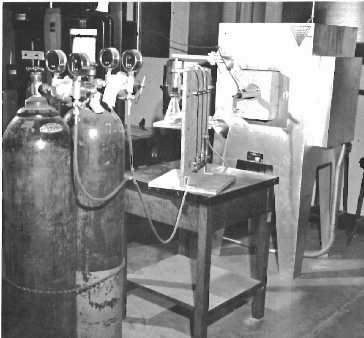
Figure 2 APPARATUS EMPLOYED IN THE SYNTHESIS OF SiC WHISKERS BY PYROLYTIC GASEOUS REACTION
