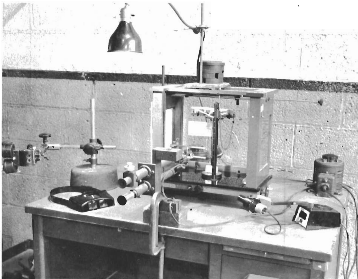
Figure 4 MODIFIED ANALYTICAL BALANCE AND ASSOCIATED FILAR MICROSCOPE FOR THE TENSILE TESTING OF WHISKERS
