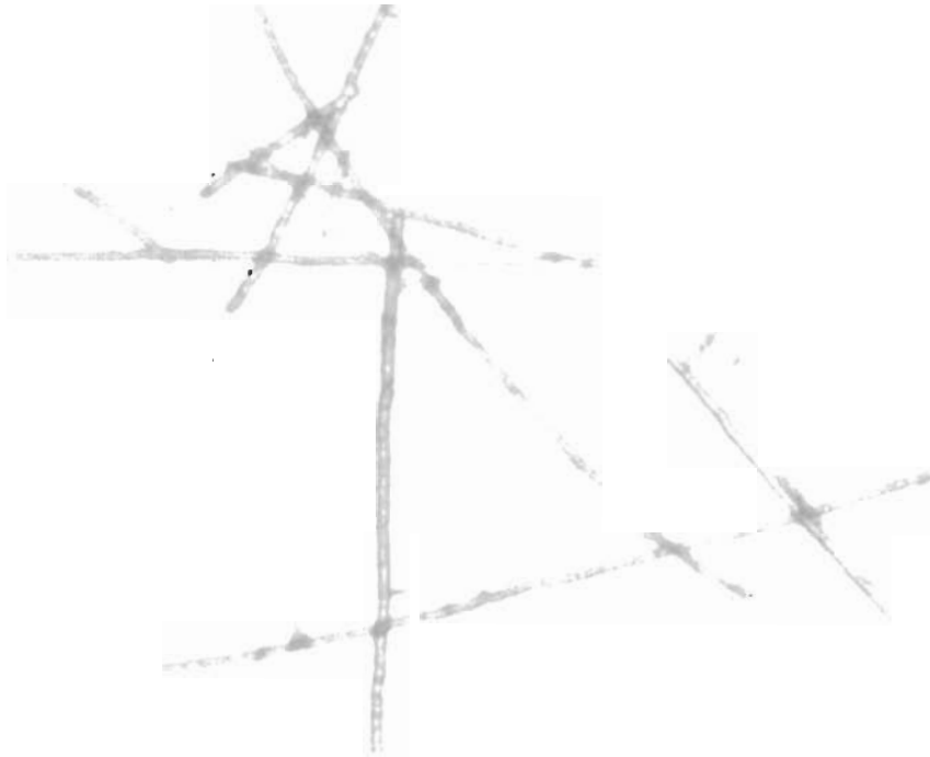
Figure 8 SHORT, STUBBY NEEDLE-LIKE GROWTH OF SiC TYPICAL OF FORMATION IN AREA B
