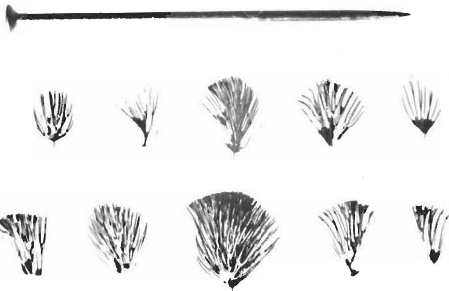
Figure 7 "BUSH" FORM OF SILICON METAL FOUND TO DEPOSIT IN AREA A OF REACTION TUBE -3.5 X MAG.
