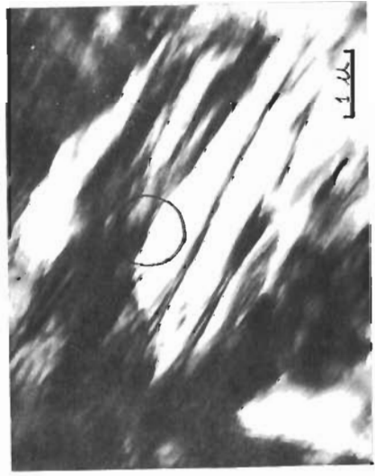
A. Bright field of tempered martensite plates. Circle indicates selected area
