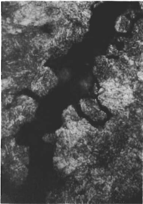
Crack Region - Etched Electrolytically at 10 A in 10% Chromic Acid
