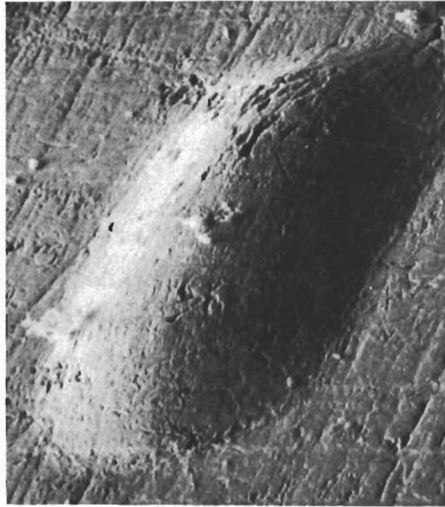
Fig. 283 - Blistered Surface of Fe-Cu Specimen Held at -1400 mV SCE in Acetate + Arsenite Solution. Scanning Electron Microscopy 1000X
