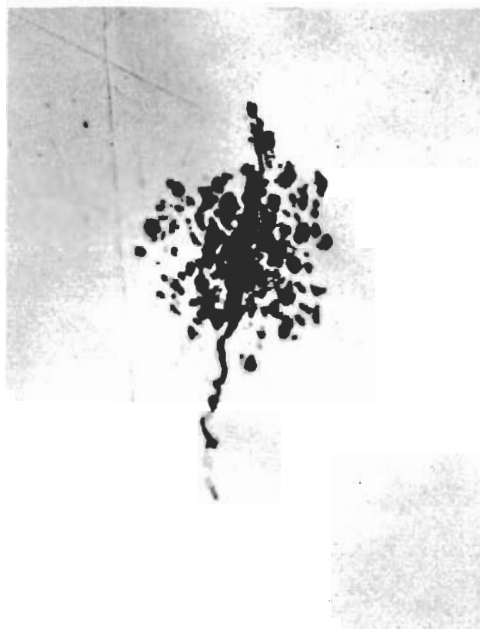
Fig. 62 - Crack Propagation from a Pit X250
