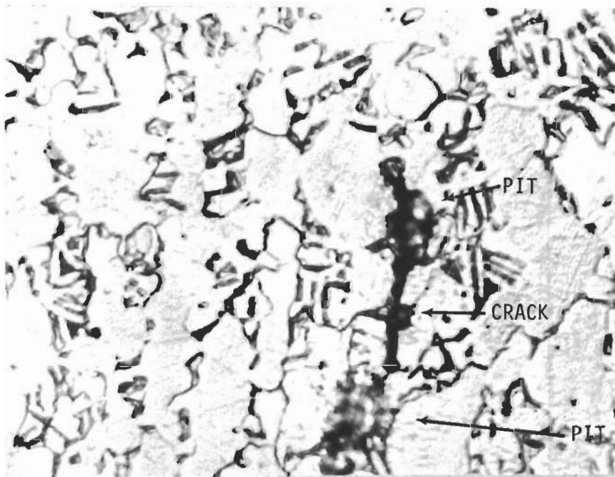
Fig. 65 - Preferential Corrosion at the \alpha - \beta Interface and \beta Phase in Ti-6Al-4V (note: micro-crack between two small pits) Kroll's Etch X2000
