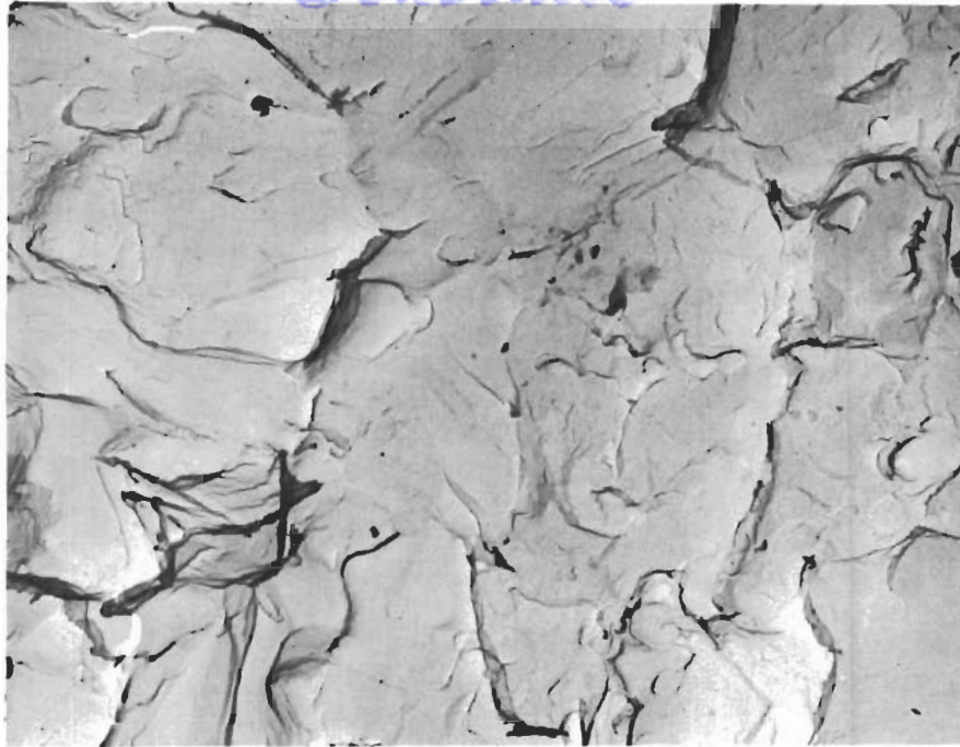
Fig. 68 - Electron Micrograph of Fracture Surface of Ti-6Al-4V Specimen (note: cleavage fracture) X7000
