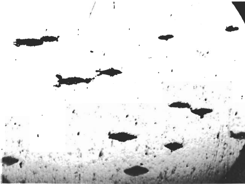
Fig. 80 - Linking of Propagating Cracks; Shape of the Crack 18 Minutes after the Initiation (100X)
