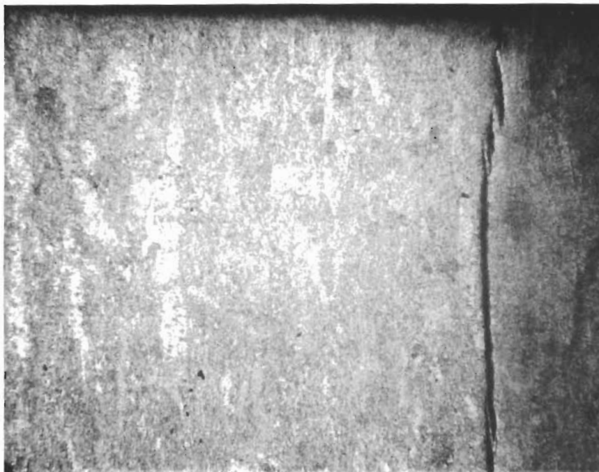
Fig. 42 - Stress Corrosion Cracking of Ti-8Al-1Mo-1V in \text{CH}_3\text{OH} + 0.5\% \text{Br}_2 X50
