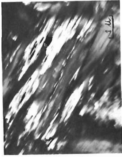
D. Dark field of spot C, [0\ 1\ 1]_T direction of twin
