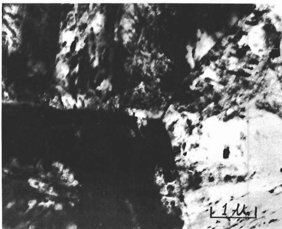
Fig. 181 - Grain Boundaries in AISI 4340 Steel of Tempered Bainite Structures Showing No Grain Boundary Precipitation of Carbides
