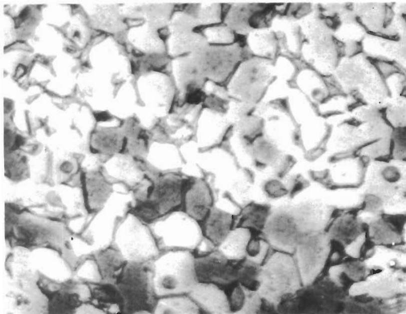
Fig. 76 - Grain Size of 10% Rolled and 32 Hour Annealed Specimen at 918° C; Average Grain Diameter 0.0110 Inch (1000X)
