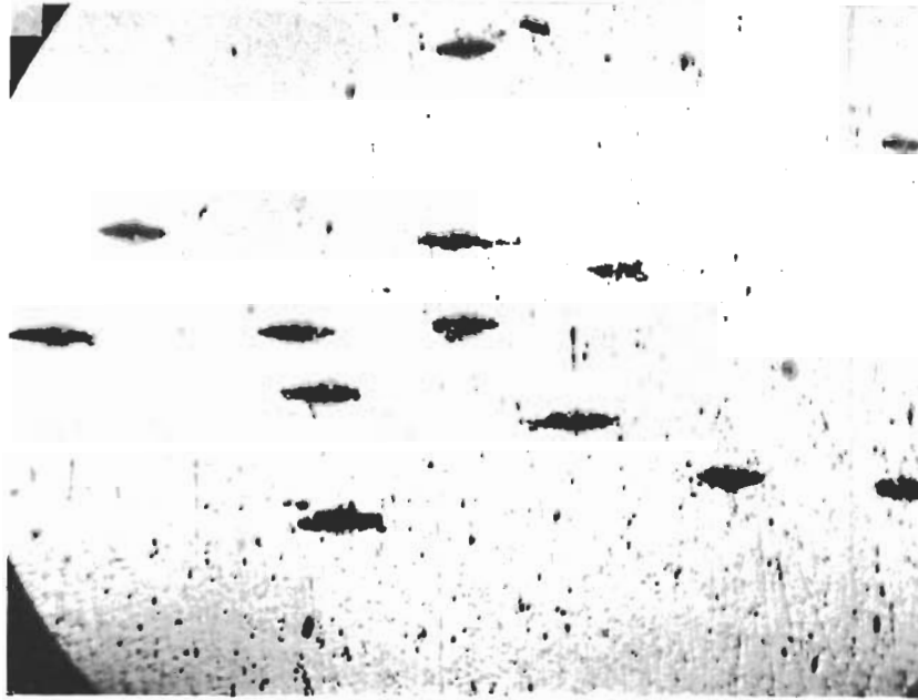
Fig. 79 - Crack Propagation from the Pit; Shape of the Crack 18 Minutes after the Initiation (100X)
