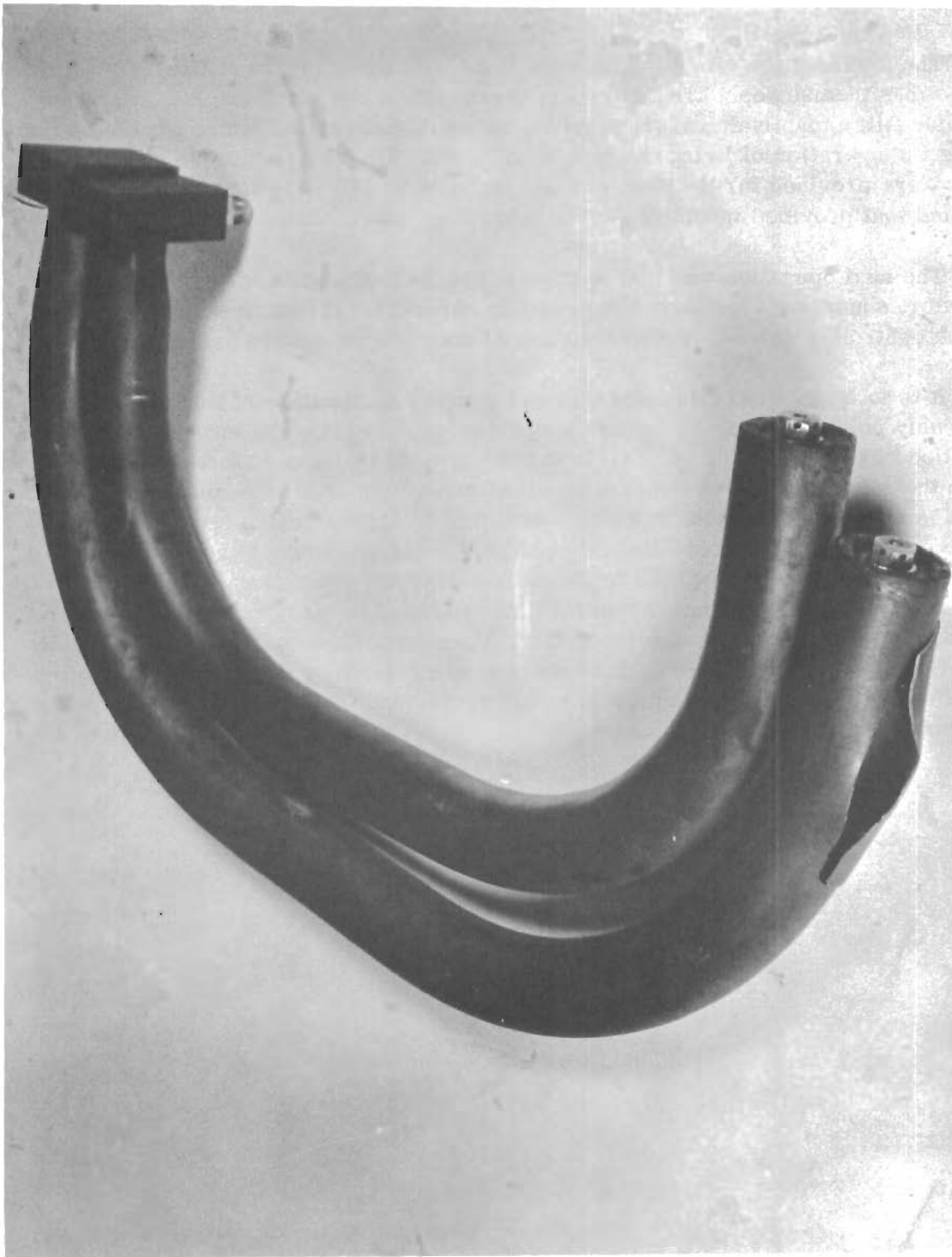
Figure 39. Test Tubes Showing High Pressure Rupture
