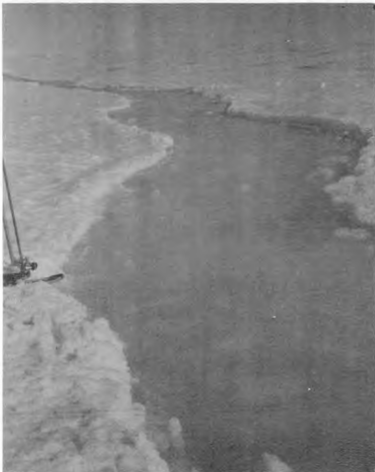
Fig. 1. Inflow channel to Alpha Lake. Note the water flowing over the snow forming a dune-type regime on the channel bottom. The small ice crystals are similar to dunes in a sand channel. The stream is flowing on snow and ice crystals which are about two feet deep.
