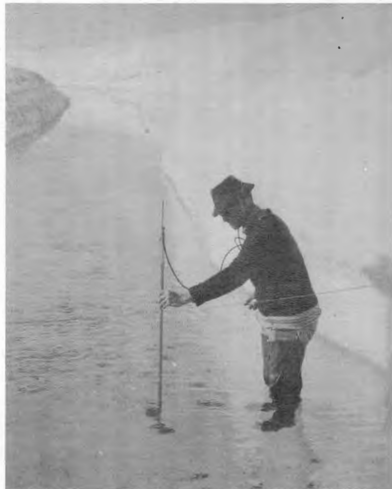
Fig. 2. Bill Mattox measuring streamflow in outlet channel to Alpha Lake. Note cryoconite in channel bottom and melting effects on ice. Location is on ice rise one mile north of Ward Hunt Island.
