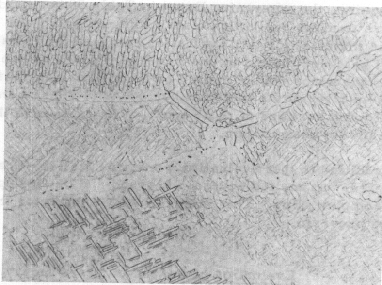
FIGURE 36. Ti-3Mn-COMPLEX ALLOY WELD METAL
