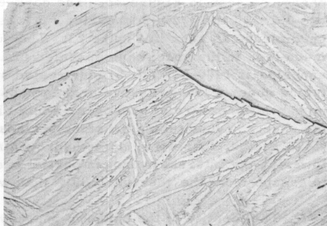
FIGURE 22. Ti-3Mn-COMPLEX ALLOY ANNEALED 5 HOURS AT 1600°F IN ARGON, SOLUTION TREATED AT 1300°F, AND OVERAGED FOR 24 HOURS AT 900°F
