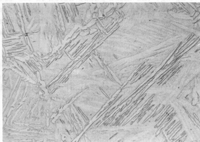
FIGURE 23. Ti-3Mn-COMPLEX ALLOY ANNEALED 5 HOURS AT 1600°F IN VACUUM, SOLUTION TREATED AT 1300°F, AND OVERAGED 24 HOURS AT 900°F
