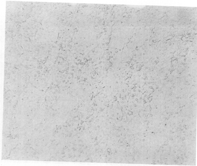
FIGURE 5. Ti-5Mn-2.5Cr ALLOY ROLLED AT 1450°F, SOLUTION TREATED 1 HOUR AT 1300°F, AND AGED 48 HOURS AT 800°F
