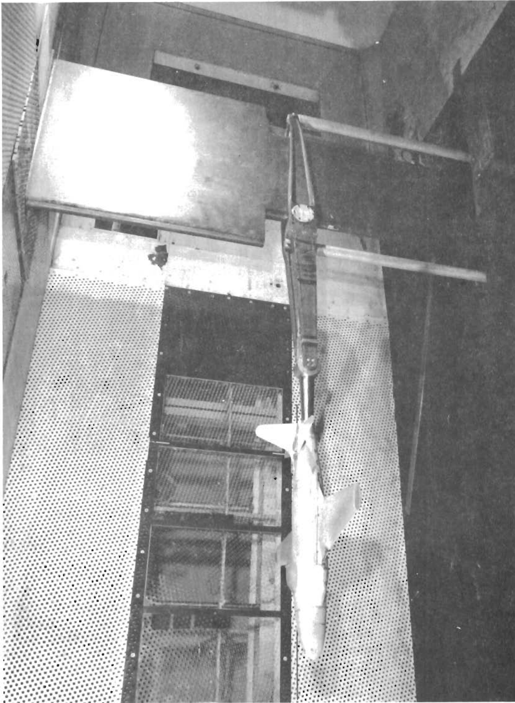
Figure 9 THE OSCILLATOR INSTALLED IN THE WIND TUNNEL
