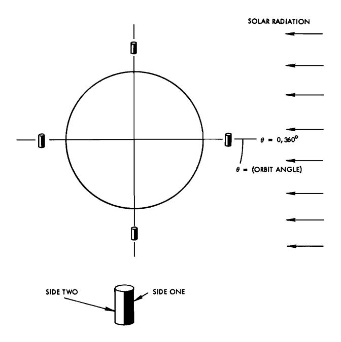
Figure 6-1. Orbit Orientation for Preliminary Analysis
