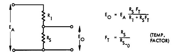
RESISTANCE THERMOMETER CIRCUIT
