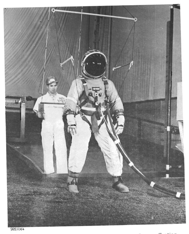
Figure 4-37. Lunar Gravity Simulation - Human Factors Testing
