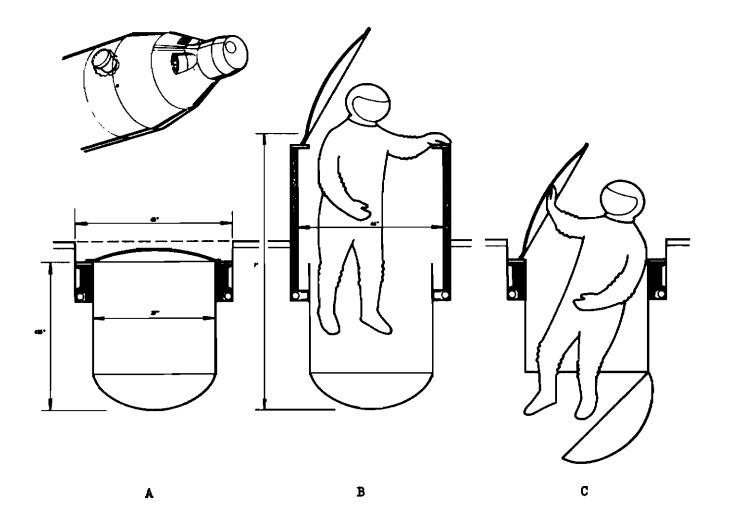
Figure 4-54. Expandable Airlock Incorporated in Existing Vehicle Hatch Structure
