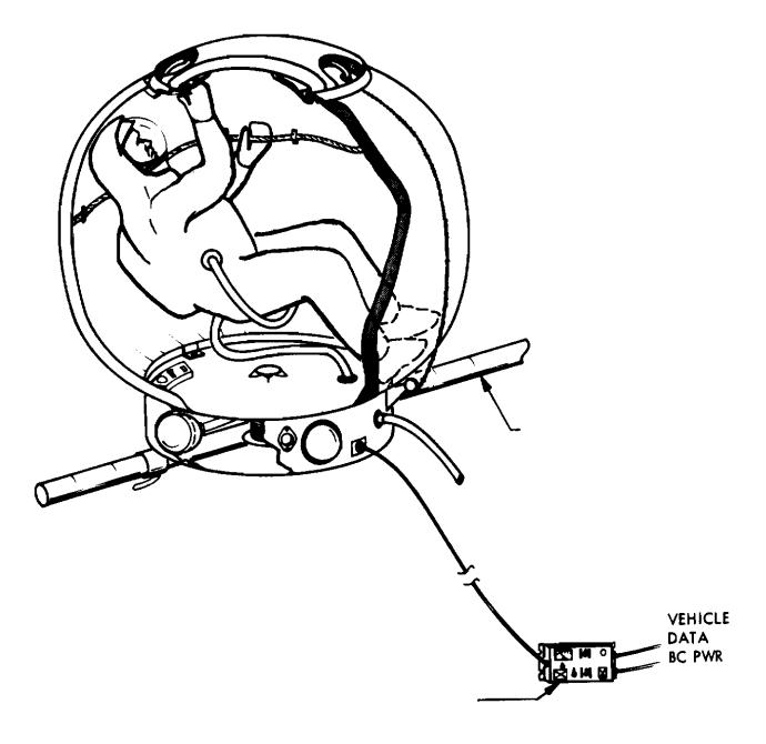
Figure 7-10. Airlock Experiment Package Configuration
