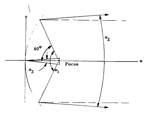
$W_1$  may be calculated from the conic plane angle 60° by  $W_1 = 4 \pi \sin^2 \frac{\theta}{2}$   $W_1 = 4 \pi \sin^2 30^\circ = 4 \pi (.25)$  $W_1 = 3.15$  steradians
