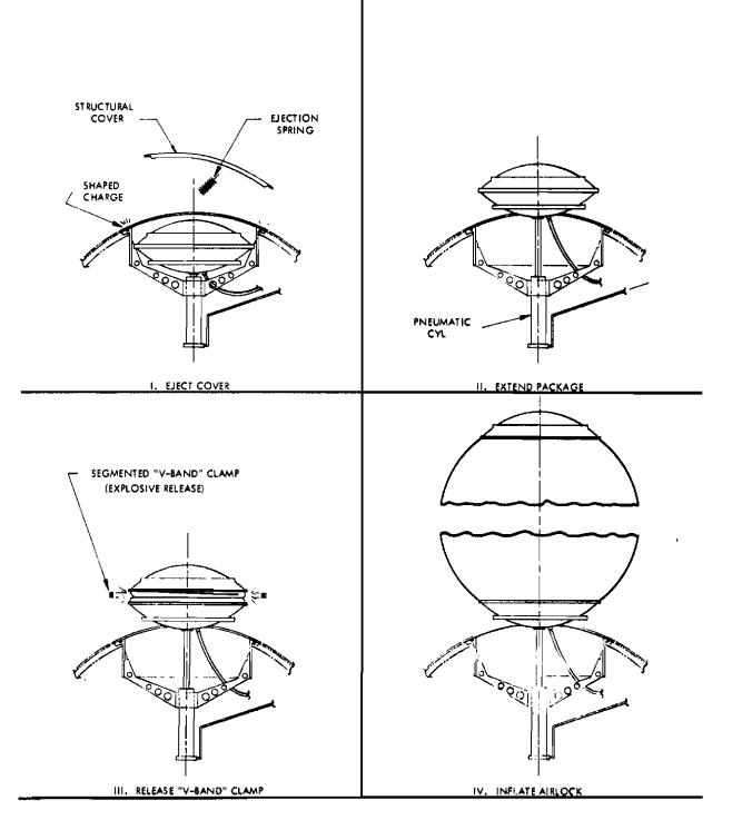
Figure 4-12. Deployment Sequence for Elastic Memory Airlock, Integral Stowage Configuration for a MSI
