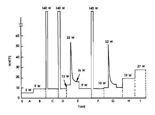
Figure 7-2. Modular Parabola Power Requirements for a Remotely Deployed, MSL Vehicle Experiment
