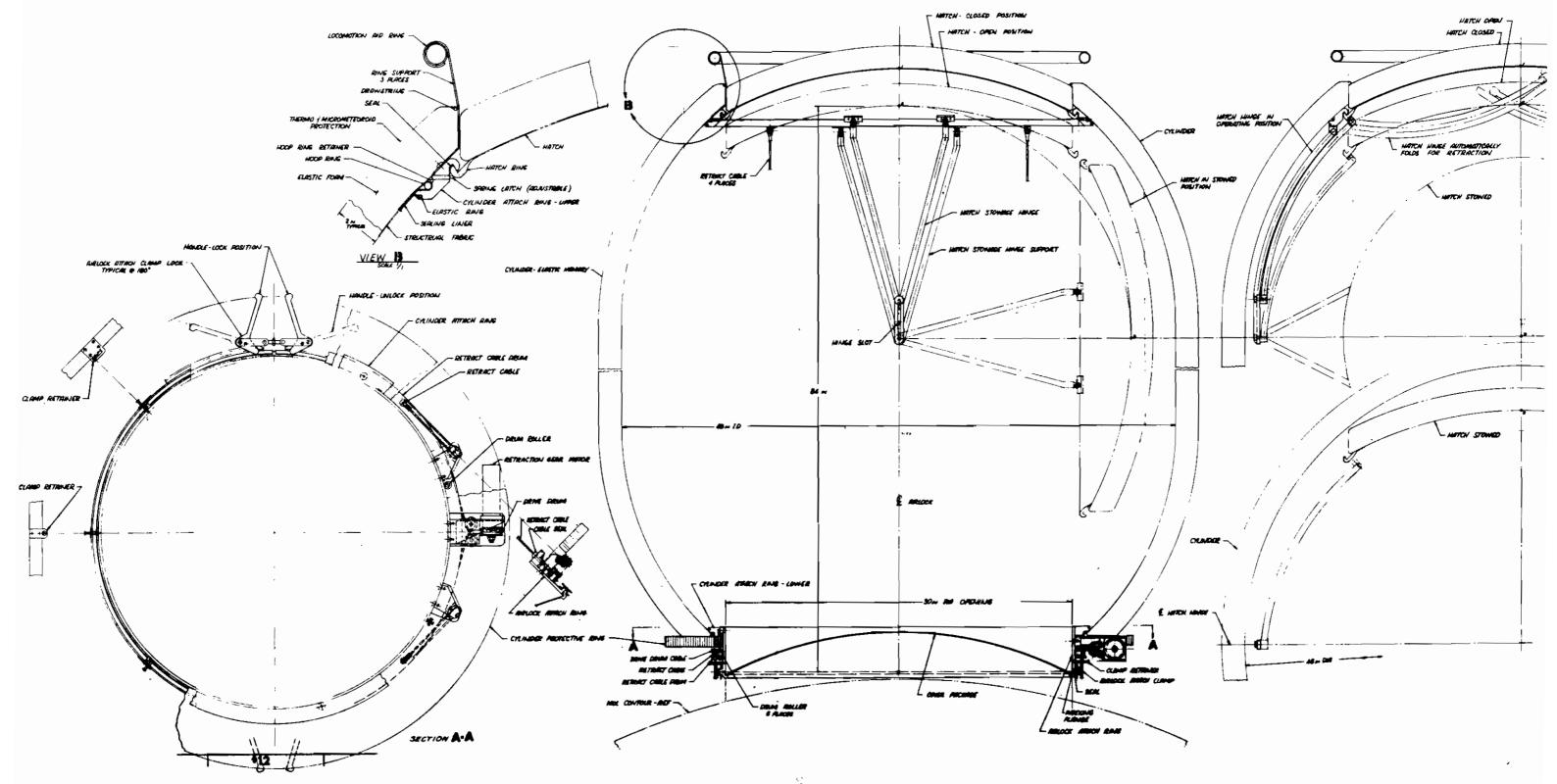
Figure 2-4 Preliminary Configuration of the Elastic Memory Airlock
