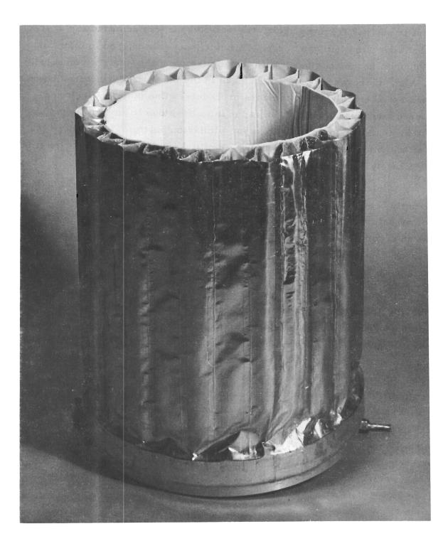
Figure 3-11. Rigidized Goodyear Cylinder
