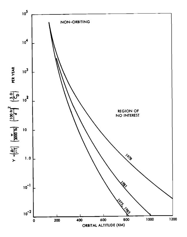
Figure 6-6. Orbital Decay Rates, 1975-1985
