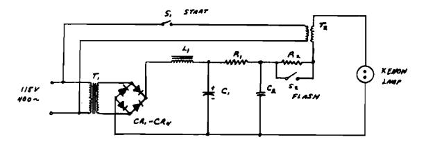
POWER SUPPLY FOR TYPICAL XENON LAMP (MAJOR CIRCUIT COMPONENTS)
