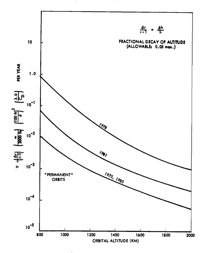
Figure 6-7. Orbital Decay Rates, 1975-1985
