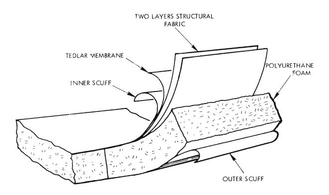
Figure 2-1. Airlock Expandable Wall Cross Section
