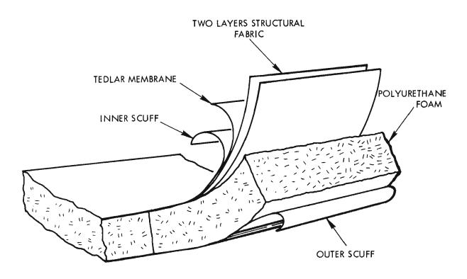
Figure 3-14. Sample Elastic Recovery Laminar Composite
