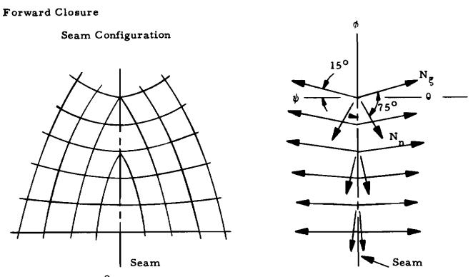
$\psi = 15^{\circ}$  Assumed Fiber Orientation with respect of Principal axes  $\theta$  and  $\phi$
