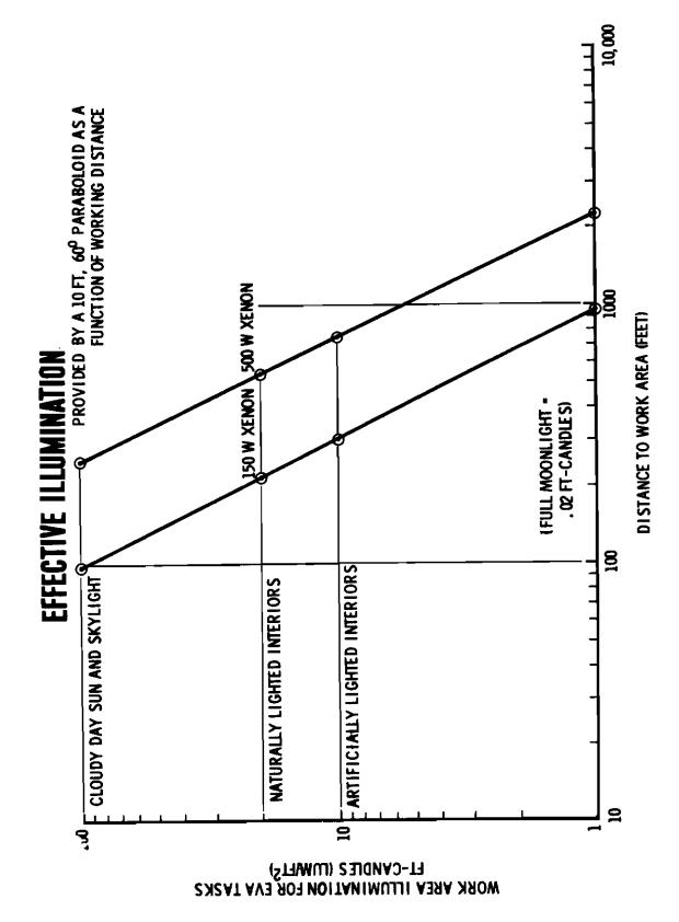
Figure 5-38. EVA Work Area Illumination Versus Distance
