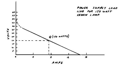
Figure 5-41. Xenon Power Conditioner Schematic and Lamp Power Load Line
