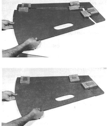
Figure 5-14. Parabola Panel and Joint Mock-Up
