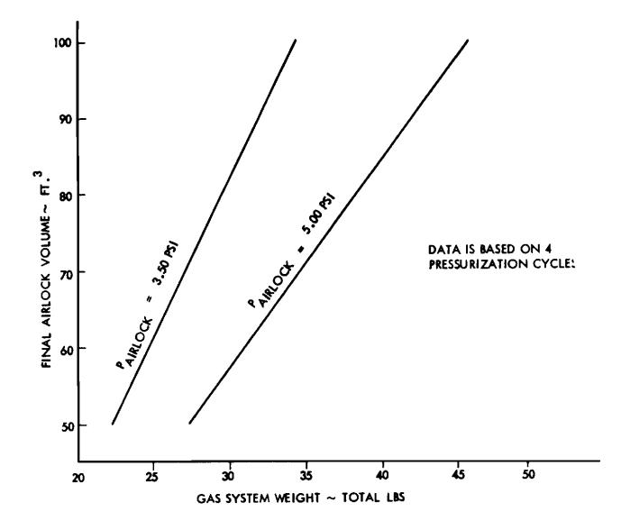
Figure 4-16. Pressurization System Weight Versus Airlock Volume
