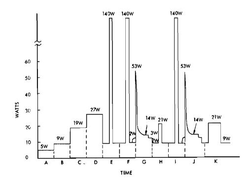
Figure 7-1. Elastic Memory Airlock Power Requirements
