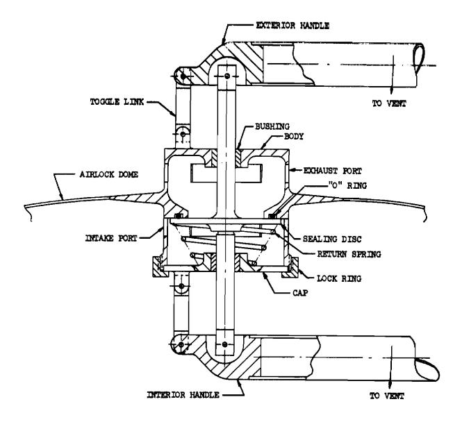
Figure 4-53. Airlock Vent Valve
