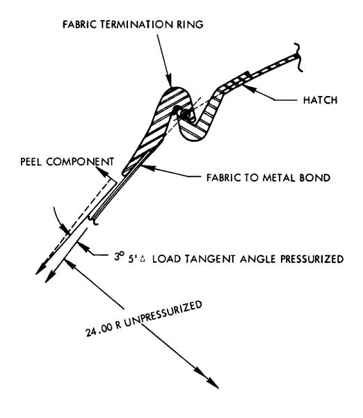
Figure 4-4. Typical Diagrammatic Crosssection of Fabric Termination Ring and Hatch Interface
