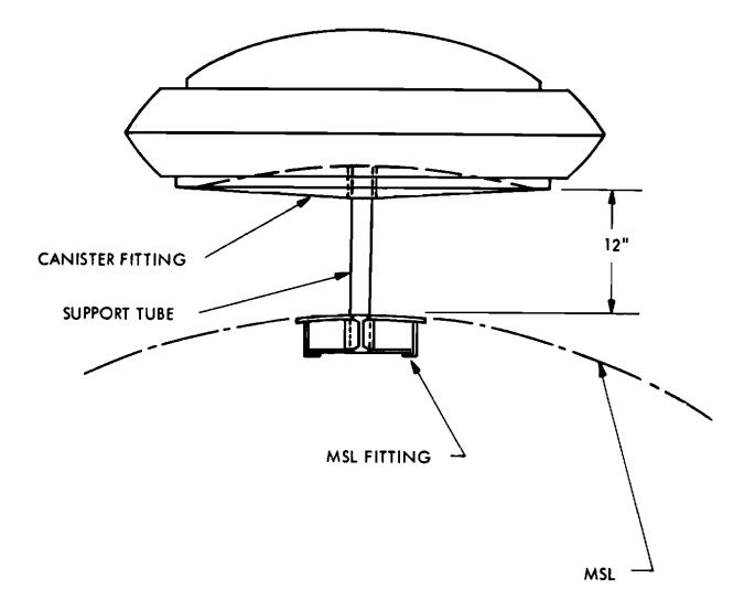
Figure 4-13. Airlock Deployment Configuration for Nonintegral (Internally) Stowed Option
