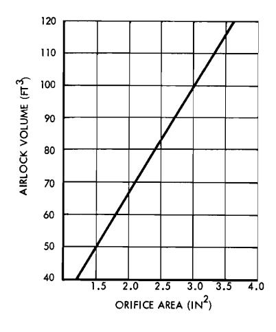
Figure 4-19. Vent Area Versus Airlock Volume for One-Minute Venting
