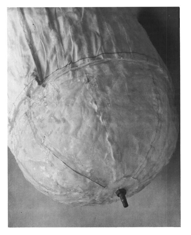
Figure 3-9. GCA-Viron Nylon Cylinder Showing Inflated End Cup with Patchy Bubbled Areas of Gelatin
