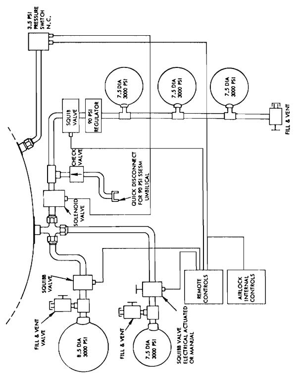
Figure 2-6. Pressurization System
