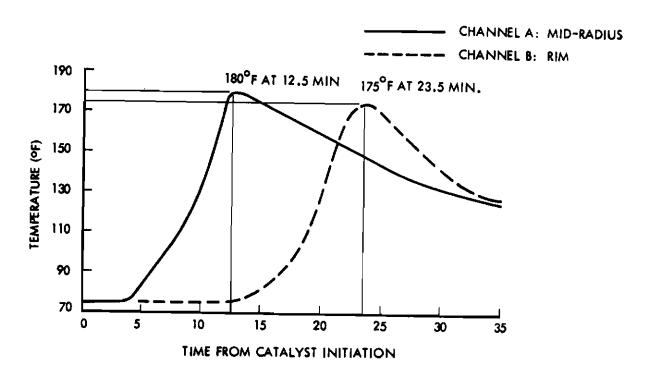
Figure 3-2. NCR Exothermic Reaction Temperatures
