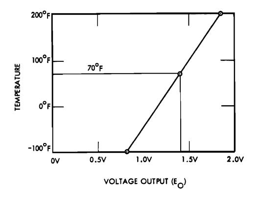
Figure 4-30. Electrical Output of Resistance Thermometer Versus Temperature
