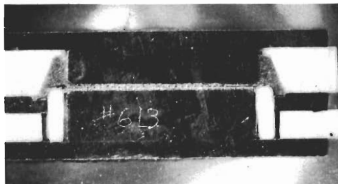
Fig. 19 Triode with Grid Stretched Over Ceramic Cylinder
