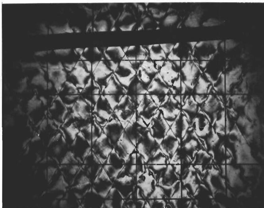
Figure 41. Stress Patterns for a Tension Loading of a Boron Filament-Reinforced Plate, Post Failure
