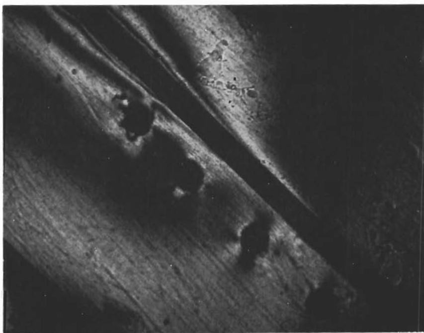
Figure 51. Unbonding in Microspecimen Subjected to Tension (Mercury Green Monochromatic Light With Crossed Quarter-Wave Plates) 35X
