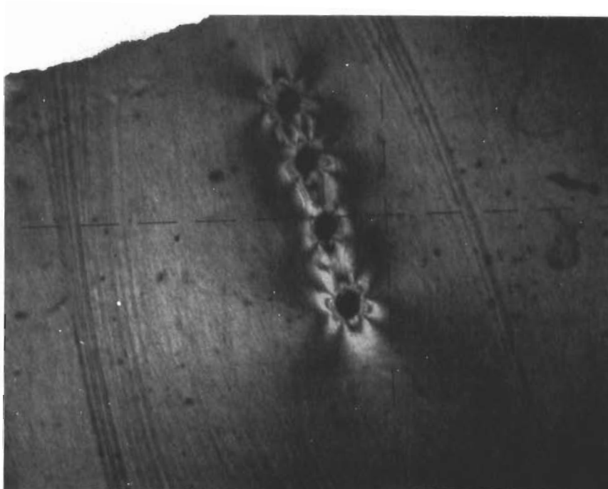
Figure 50. Microspecimen Subjected to Tension (Mercury Green Monochromatic Light With Crossed Quarter-Wave Plates) 25X
