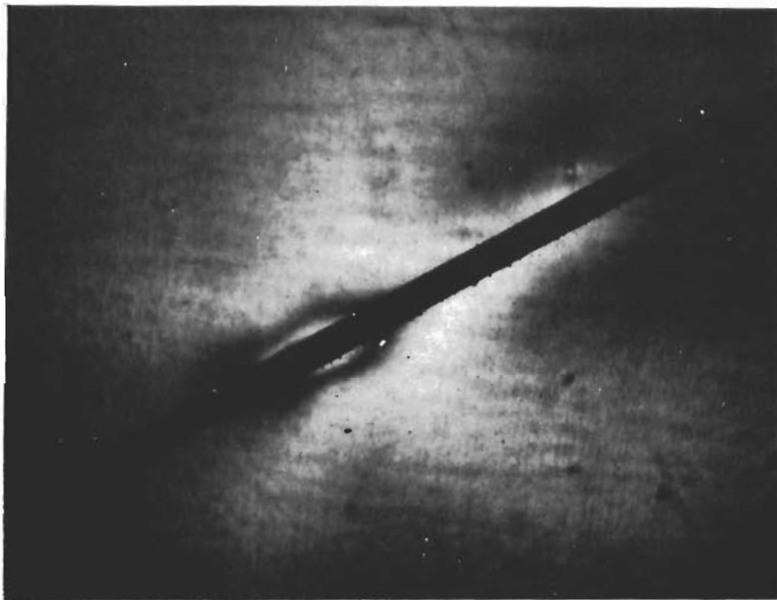
Figure 53. Detail of Reinforced Disk Subjected to Diametral Compression (Mercury Green Monochromatic Light With Crossed Quarter-Wave Plates) 35X
