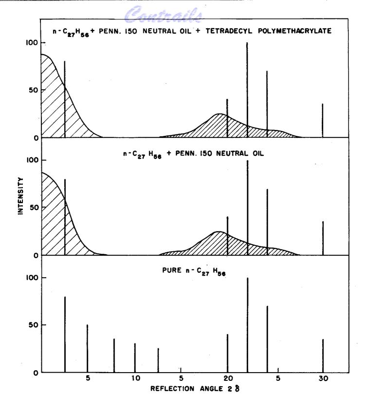
FIG. 18-EFFECT OF POUR POINT DEPRESSANT ON X-RAY DIFFRACTION PATTERNS OF n - HEPTACOSANE
