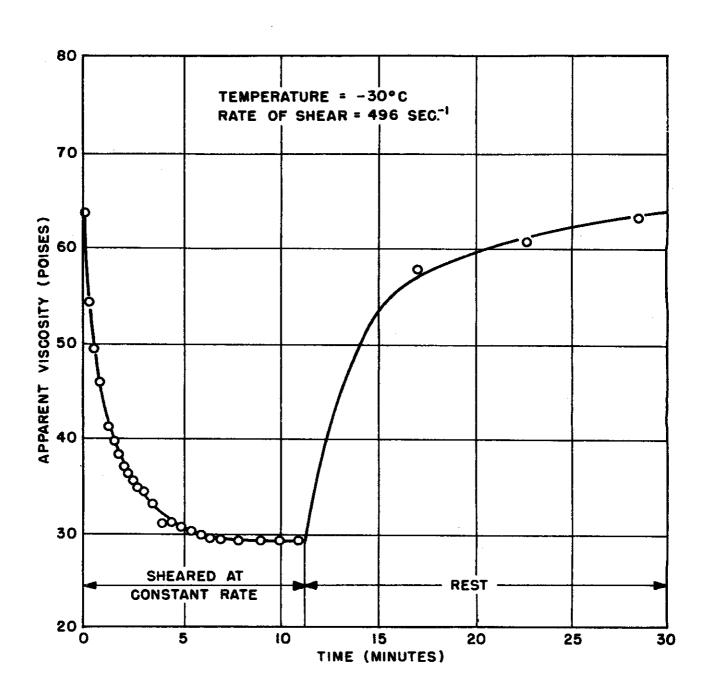
FIG. 79 - RECOVERY OF VISCOSITY ON STANDING AFTER SHEARING TO EQUILIBRIUM AT A HIGH RATE OF SHEAR.
