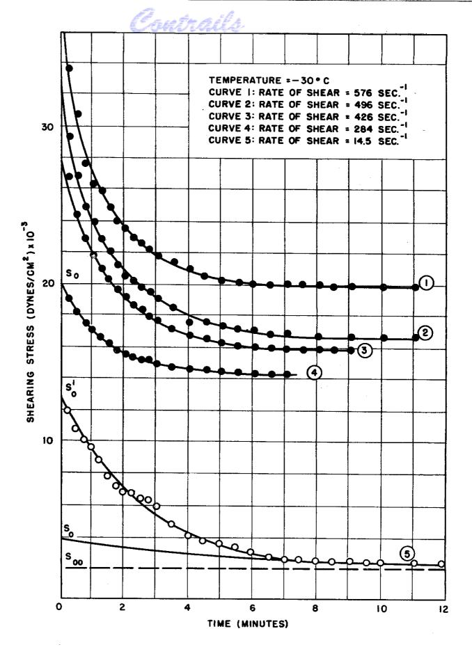
FIG. 74-STRESS RELAXATION CURVES AT CONSTANT RATES OF SHEAR.
