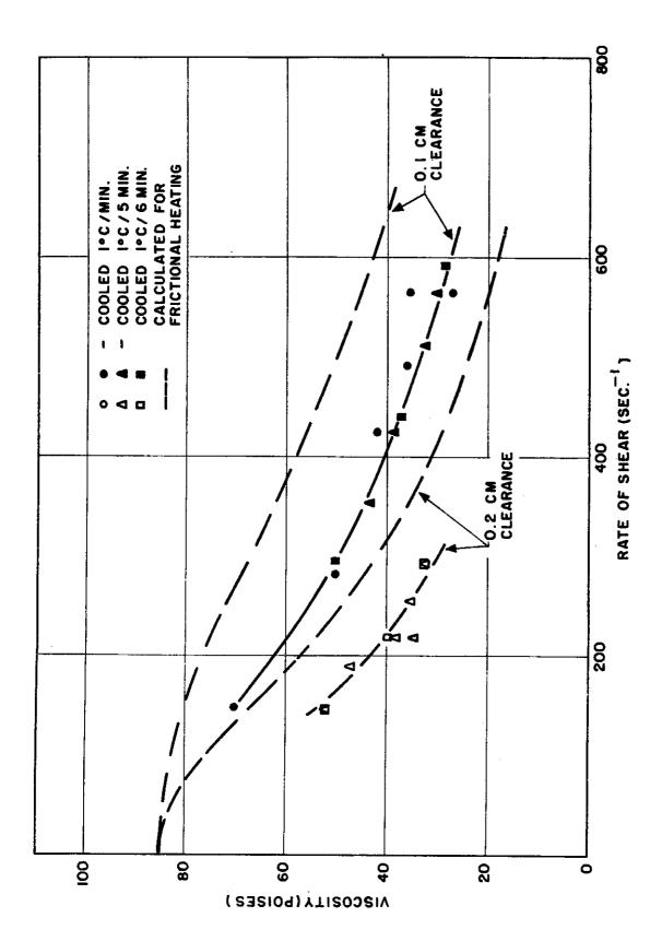
FIG. 32 - EQUILIBRIUM VISCOSITIES OBSERVED WITH THE INTERCHEMICAL VISCOMETER AND CALCULATED FOR FRICTIONAL HEATING. PENN. 150 NEUTRAL OIL AT -30°C
