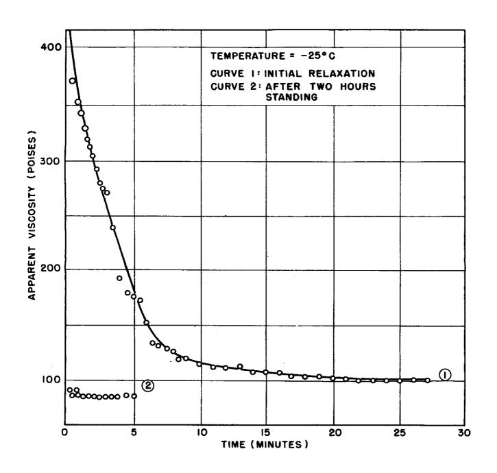
FIG. 80 - RELAXATION CURVES DETERMINED AT A LOW RATE OF SHEAR INITIALLY AND AFTER TWO HOURS STANDING.
