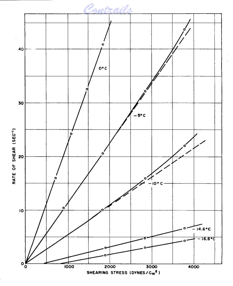
FIG. 34 - CONSISTENCY CURVES FOR GRADE 1100 AIRCRAFT OIL
