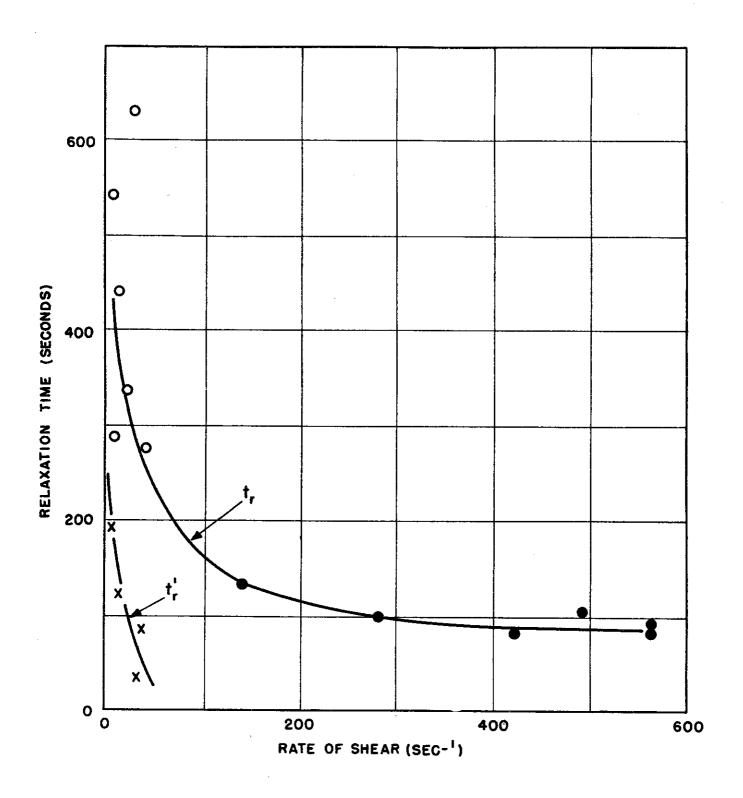
FIG. 76 - RELAXATION TIMES AS A FUNCTION OF RATE OF SHEAR TEMPERATURE \*-30 °C
