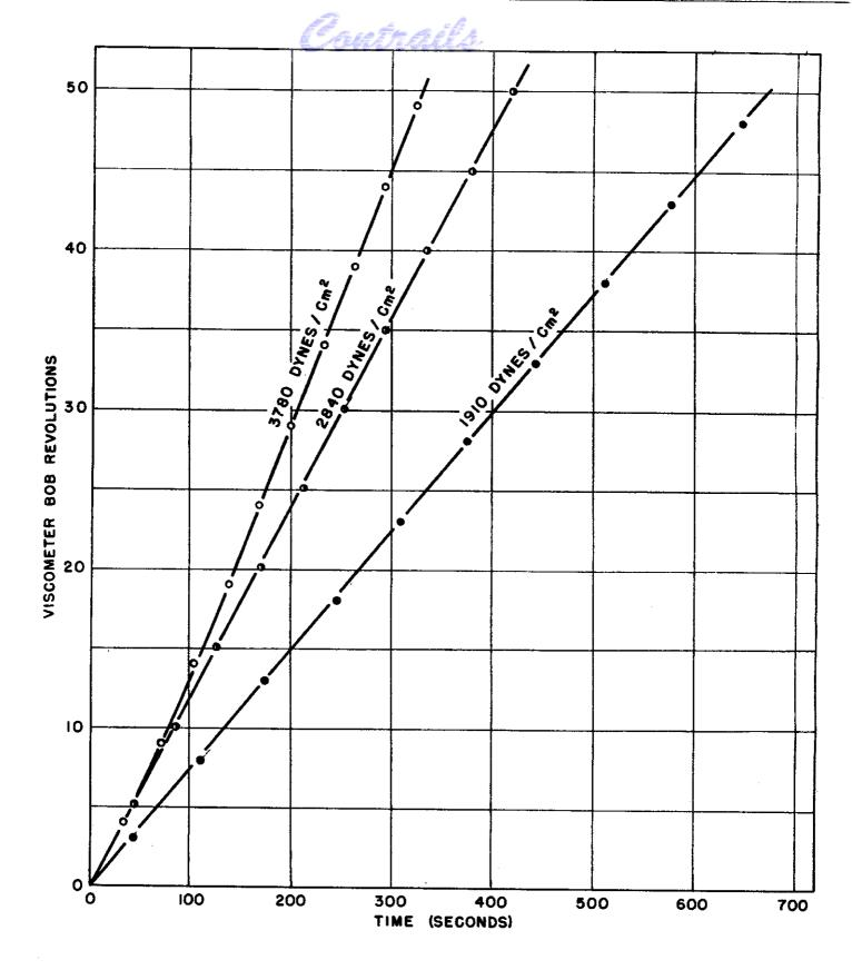
FIG. 35 - BOB REVOLUTIONS VS. TIME FOR GRADE 1100 OIL IN THE MODIFIED STORMER VISCOMETER BELOW THE POUR POINT (TEMPERATURE = -14°C, +8°F)
