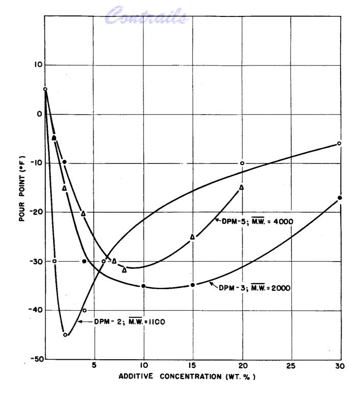
FIG.7 - PENNSYLVANIA MINERAL SEAL OIL ADDITIVE ACTIVITY OF DODECYL POLYMETHACRYLATE AS A FUNCTION OF AVERAGE MOLECULAR WEIGHT
