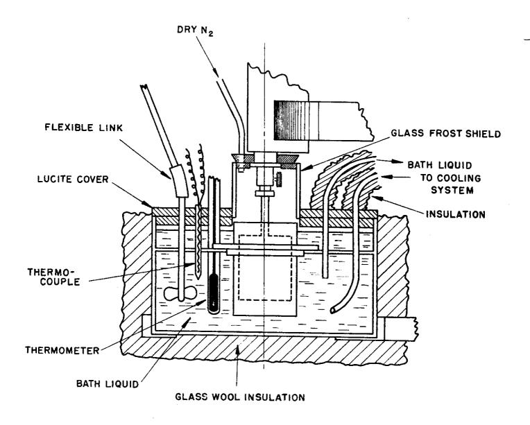
FIG. 20 - STORMER VISCOMETER MODIFICATIONS
