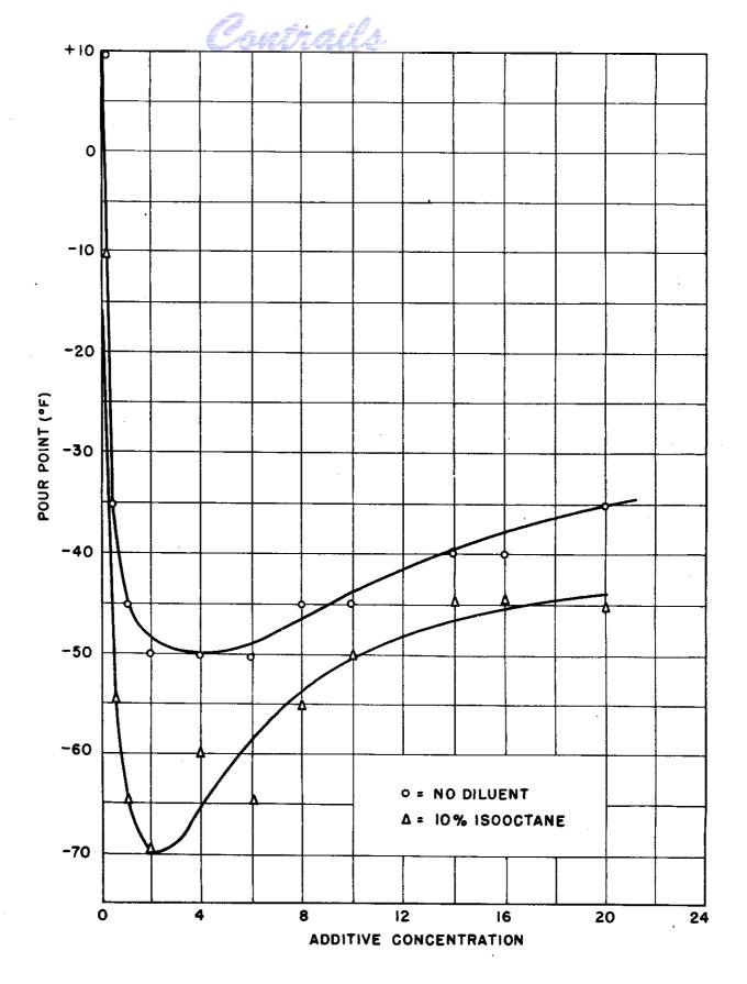
FIG. II - POUR POINT DEPRESSING EFFECT OF DODECYL POLY. METHACRYLATE (M.W.=14,000) ON PENNSYLVANIA
