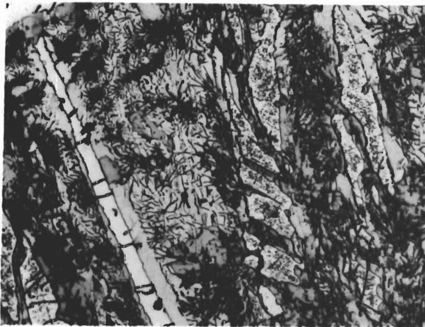
Figure 38. W-B-C (39-56-5 At.%), Melted and Rapidly Cooled. X375.
