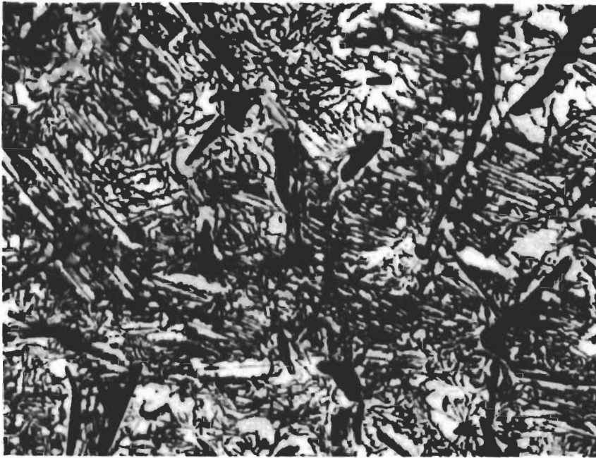
Figure 33. W-B-C (45-35-20 At.%), Rapidly Cooled from Liquidus Temperatures.
