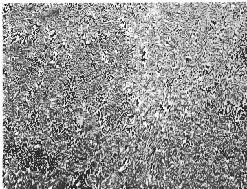
Figure 14. W-B-C (68-18-14 At.%), Melted and Rapidly Cooled. X680
