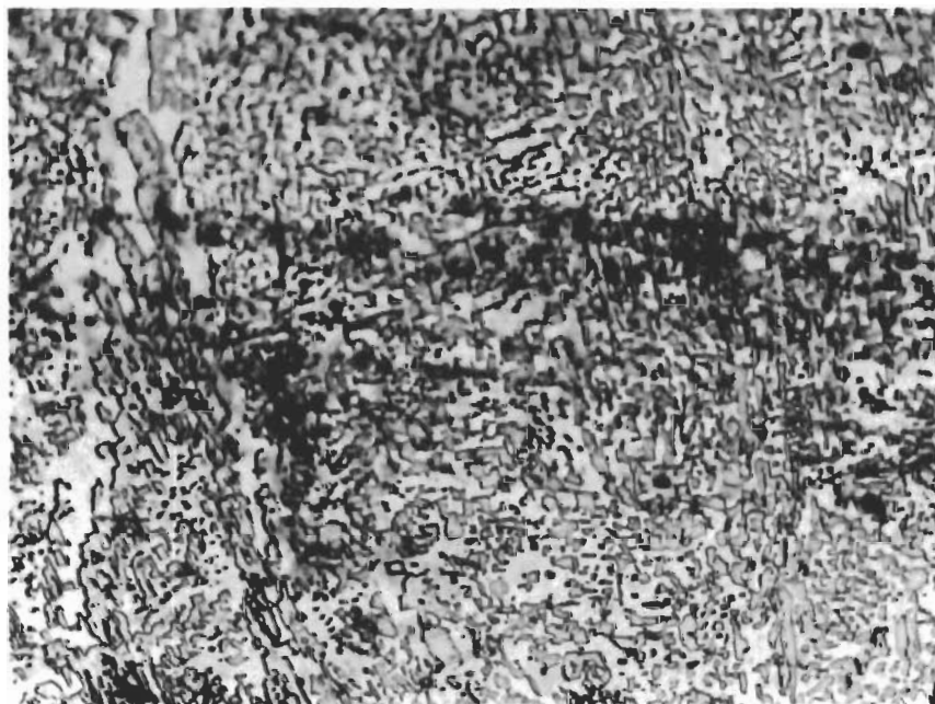
Figure 23. Sample Shown in Figure 28 Reequilibrated for 3 hours at 1800^{\circ}C and Rapidly Cooled. X520
