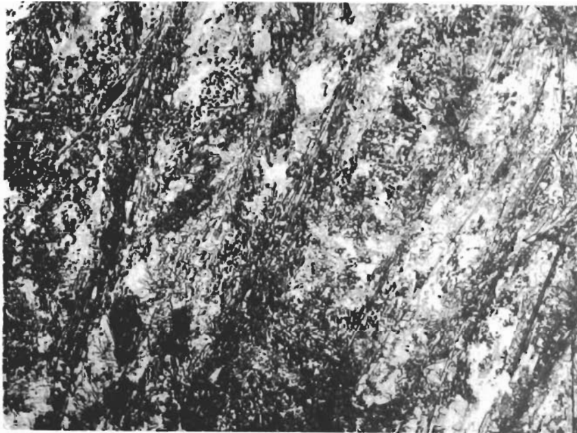
Figure 26. W-B-C (55-25-20 At.%), Melted and Rapidly X400 Cooled.
