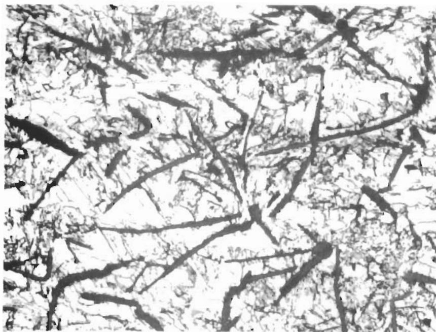
Figure 40. W-B-C (34-55-11 At.%), Melted and Rapidly Cooled.
