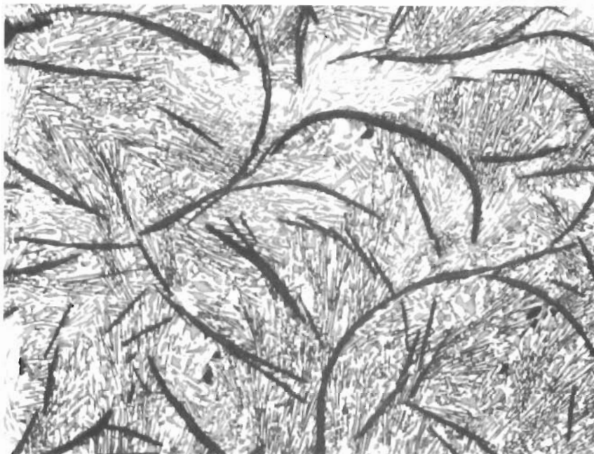
Figure 42. W-B-C (18-68-14 At.%), Melted and Rapidly Cooled. X270
