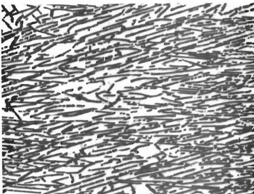
Figure 36. W-B-C (30-63-7 At.%), Rapidly Cooled from Liquidus Temperatures.
