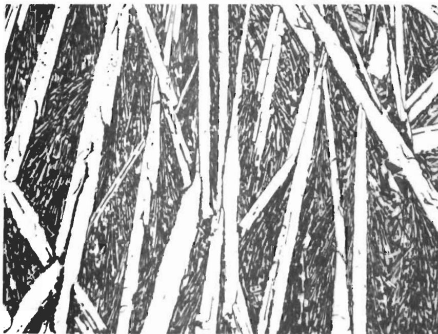
Figure 41. W-B-C (25-70-5 At.%), Melted and Rapidly Cooled.
